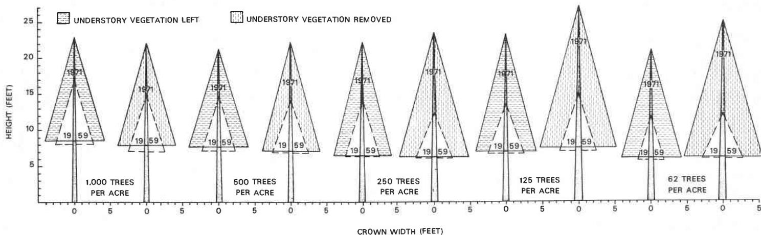
Average crown dimensions of the 62 largest diameter trees per acre in 1959 and 12 growing seasons later. Crown widths for 1959 were estimated from 1971 regressions of crown width on diameter.
