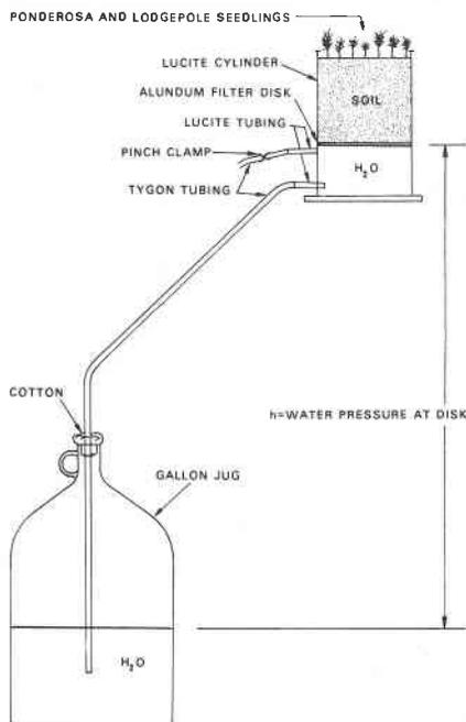
Apparatus for controlling soil water suction.
