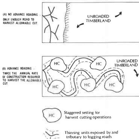
Harvesting the annual allowable cut from a continually receding "wall of timber." "A" requires less road construction than "B", advance roading.
