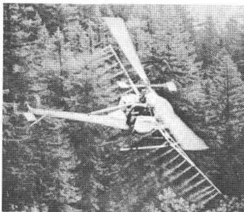
Helicopter applying 5 gallons of herbicidal spray per acre; the second 5 gallons per acre will be applied at right angles to the initial lines of flight.
