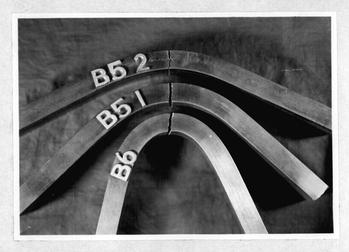
Figure 18. Results of Flexure Test. Lower "Y" Block, Upper Two Plate Material.
