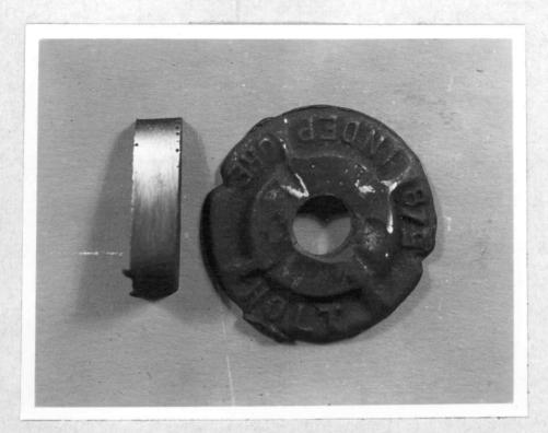
Figure 1h. Pinholes in Surface of Ductile Iron Washer (white) and Section of 1/2-inch Plate (dark).
