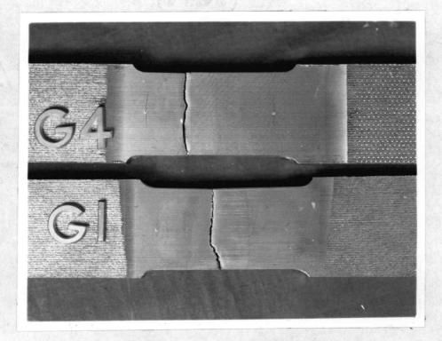
Figure 75. Fractured Heliarc Welded Test Specimen.
