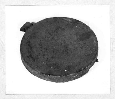
Figure 9. Ductile Iron Gear Blanks, 8 inches in Diameter.
