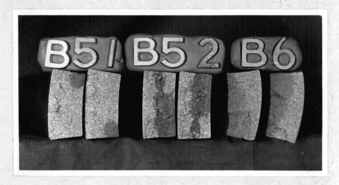
Figure 19. Fractured Ends of Specimens Shown in Figure 18.
