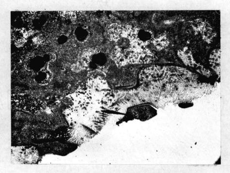
Figure 56. Preheated Fusion Zone. 100X.
