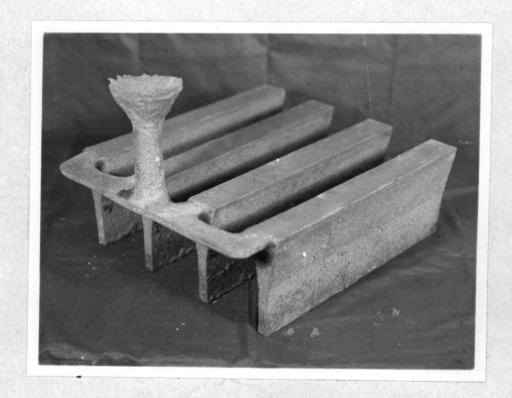
Figure 22. Gating System for Ductile Iron "Y" Blocks.
