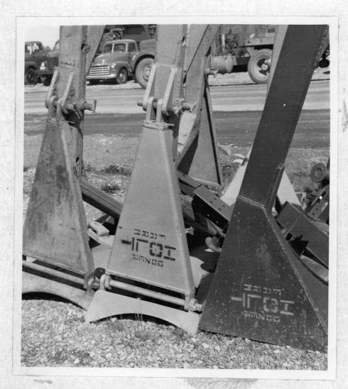
Figure 12. Ductile Iron Grader Blade Connection Brackets, Left and Center.
