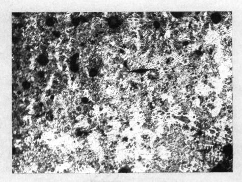
Figure 46. Parent Metal Heat Affected Zone of Weld in Figure 45. 100X.
