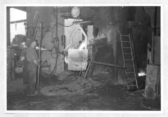
Figure 3. Tapping of Ductile Iron from Cupola.
