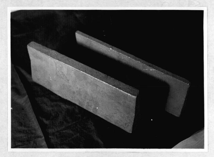
Figure 15. Ductile Iron "Y" Blocks.
