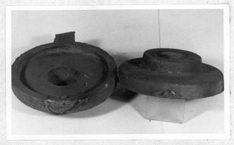
Figure 8. Ductile Iron Caps for Hydraulic Cylinder. Repair of Foundry Defects by Carbon Arc Welding is Shown.
