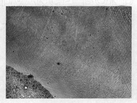
Figure 54. Carbide Network in Annealed Weld with 308-15 Electrodes. 100X.
