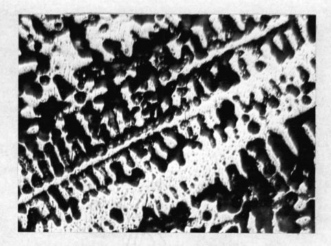
Figure 66. Weld Deposit. Ni-Rod 55 as Welded. 500X.
