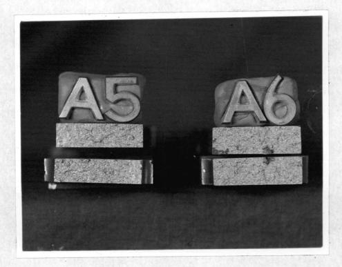
Figure 72. Ends of Bars in Figure 71. Few Defects are Noted.
