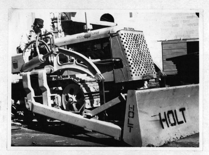
Figure 10. Ductile Cast Iron Power Arm in Operation.
