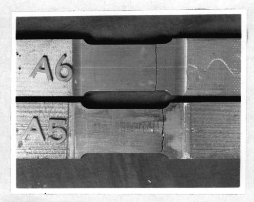
Figure 71. Parent Metal As-Cast "Y" Block Tensile Test Bars.
