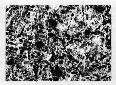
Figure 29. Ductile Iron As Cast. 100%.
