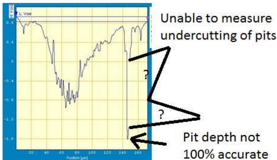
**Figure 83 - Limitations of the optical profilometry method.**
