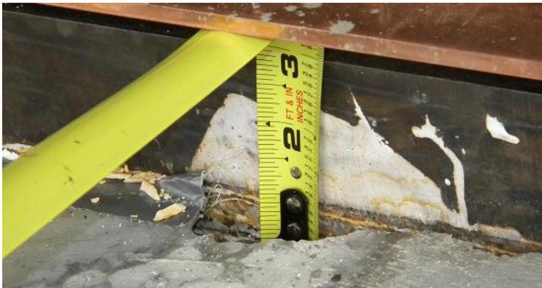
Figure 4.17b: Punching of 3 in. thick bearing plate at failure of Pile Cap #5
