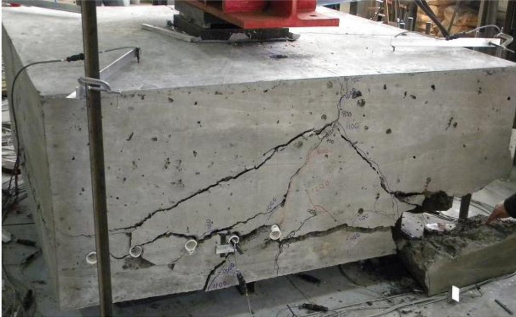
Figure 4.11a: Failure of Pile Cap #4
