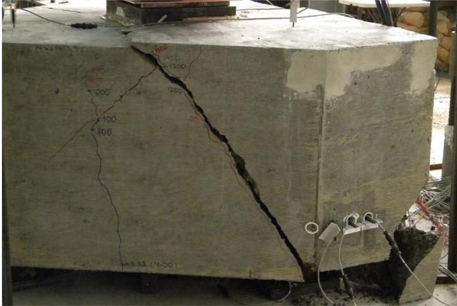
Figure 4.5: Failure of Pile Cap #3
