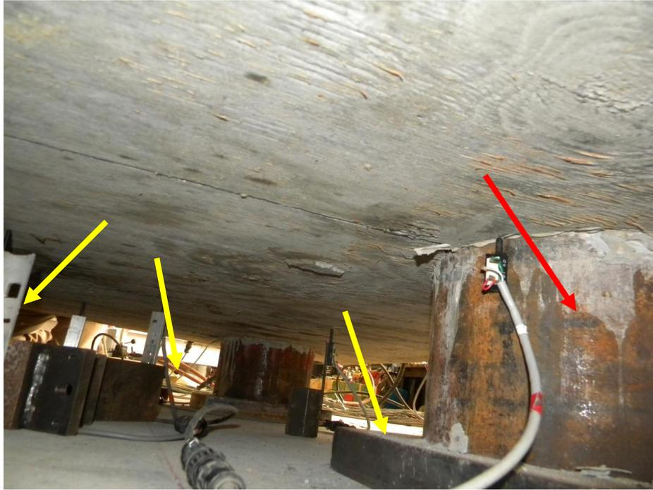
Figure 3.2.3 Example vertical displacement measurements of specimen relative to strong floor (yellow arrows) and pipe motion relative to concrete (red arrow)
