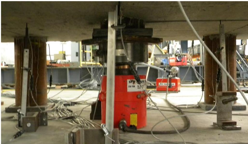
Figure 3.3.4: Hydraulic Cylinder and Load cell for center pile control with specimen #5
