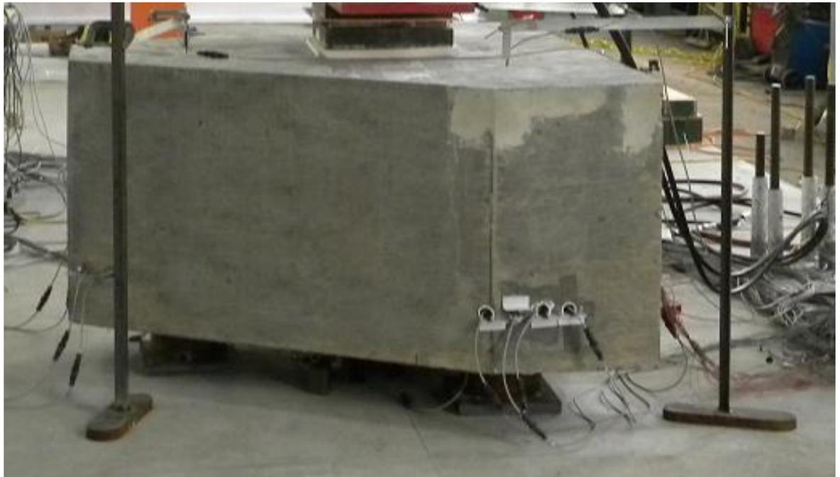
Figure 3.1.2d: Elevation view of completed specimen on strong floor – Pile Cap #3
