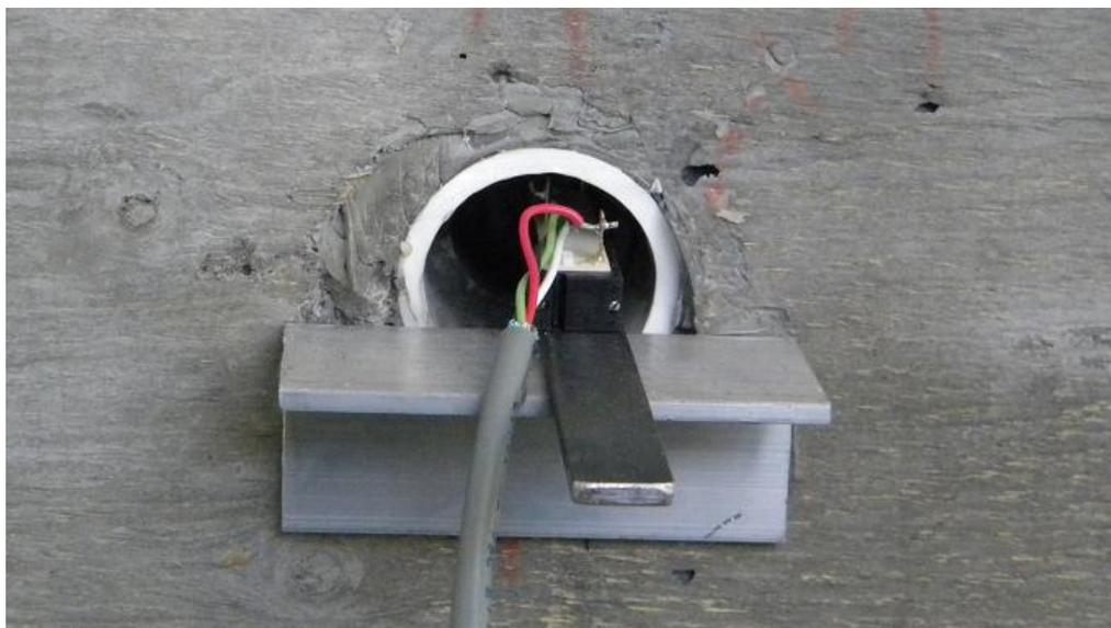
Figure 3.2.2: Example reinforcing steel slip displacement sensor
