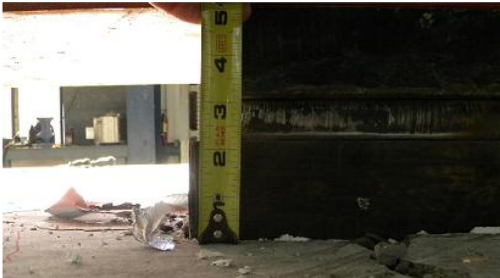
Figure 4.11b: Punching of 3 in. thick bearing plate at failure of Pile Cap #4
