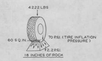
An example of a truck's weight distribution is: If a truck's wheel has a load of 4,222 pounds and a tire contact area of 60 square inches, it applies a force of 70 pound per square inch to the road surface—be it rock or soil (dirt). If the road had an 18-inch layer of rock over the soil, the truck applies a force of 2.2 pounds per square inch to the soil. The truck would exert less force to the soil surface than a 200-pound man standing on soil.
