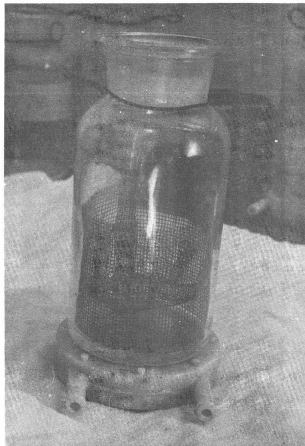
Figure 2. Respiratory chamber with cage and stirring motor.
