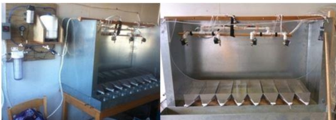
Figure 1 - Overhead leaching apparatus used to evaluate the effects of BMP procedures on copper migration from ACZA, CA or ACQ treated wood.
