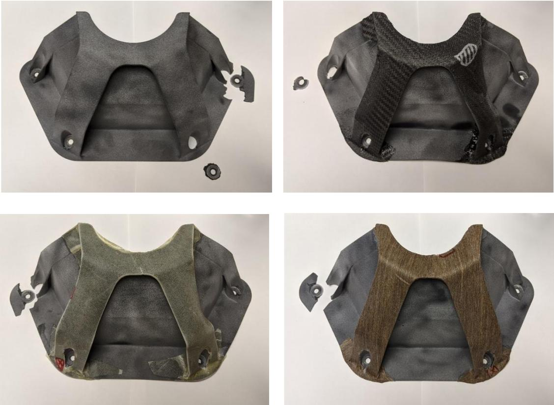
Figure 3.14 – As-printed (top left), carbon fiber (top right), fiberglass (bottom left), and flax reinforced (bottom right) picker body samples after failure [6].
