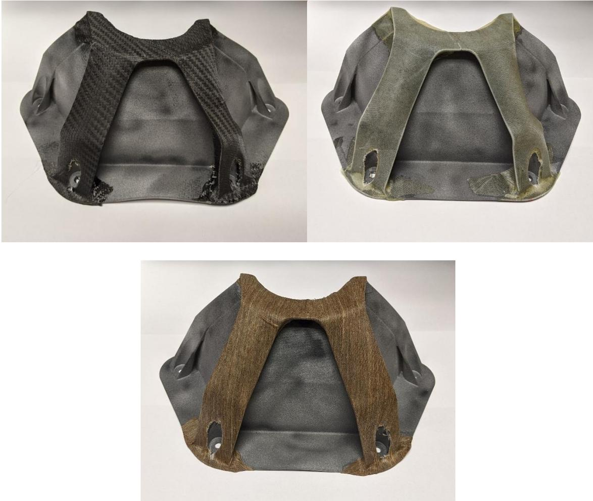
Figure 3.10 – Warped picker bodies reinforced with carbon fiber (top left), fiberglass (top right), and flax (bottom) [6].
