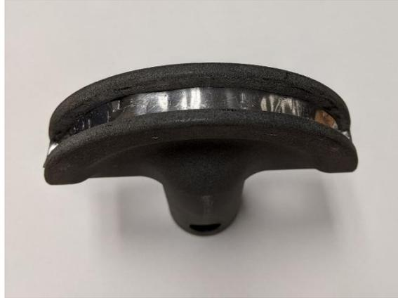
Figure 2.7 – Reinforced picker body testing fixture.
