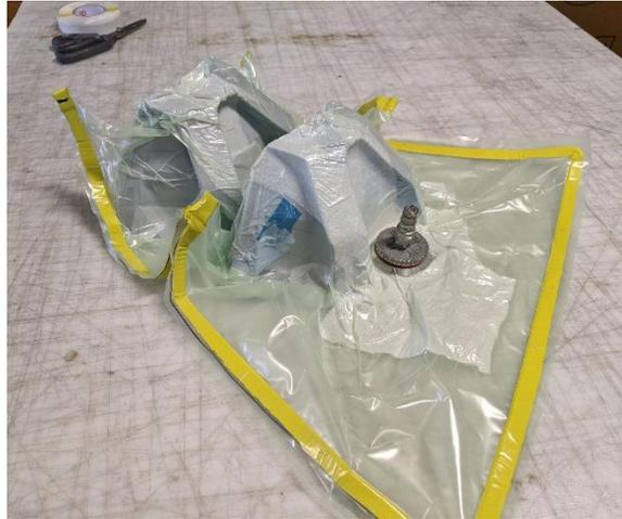
Figure 2.5 – Envelope bag vacuum sealed picker body components [6].
