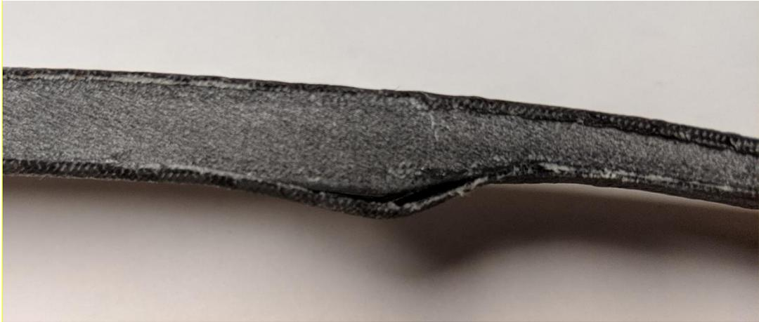
Figure 3.7 – Fiber and matrix debonding is shown after testing in the CFRP linkage arm [6].
