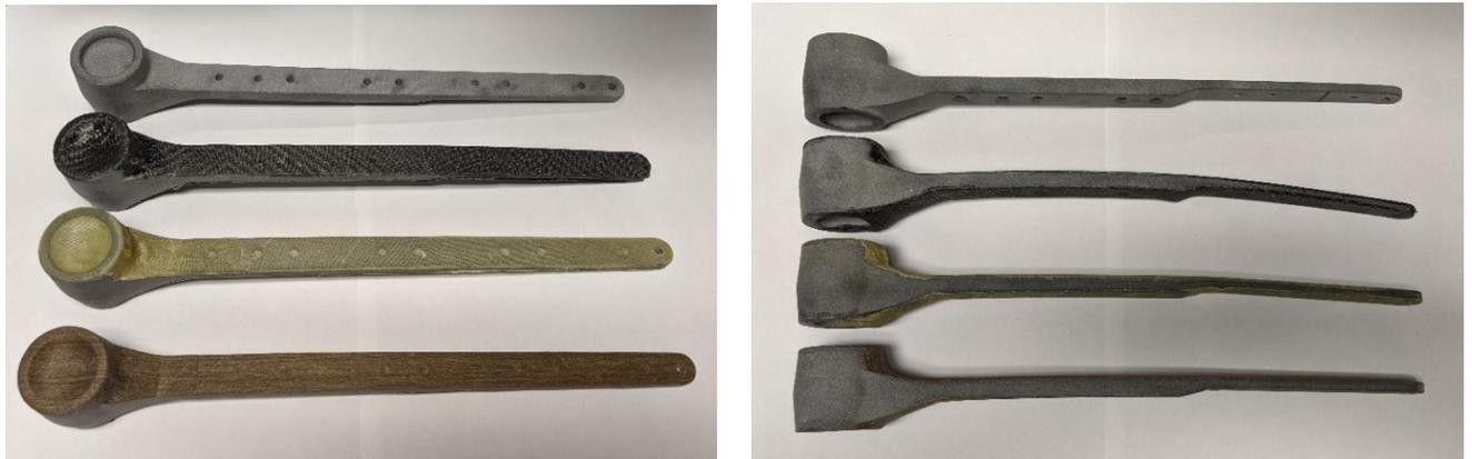
Figure 3.5 – The order of components from top to bottom is as-printed, CFRP, GFRP, and flax fiber reinforcement [6]. Warpage in the CFRP and GFRP is evident.
