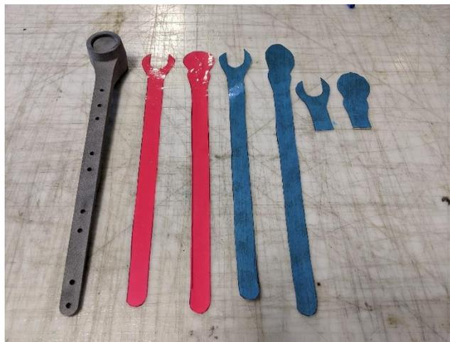
Figure 2.1 – Linkage arm prepreg film [6].
