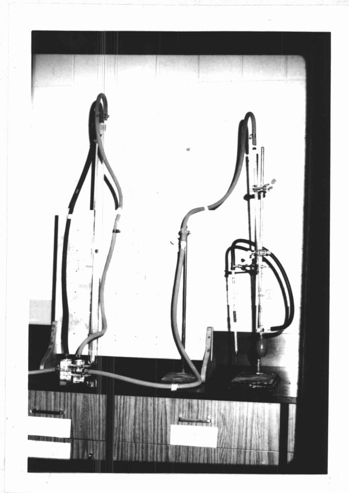
Figure 2. Apparatus for measuring the rate of longitudinal air flow through the wood samples.
