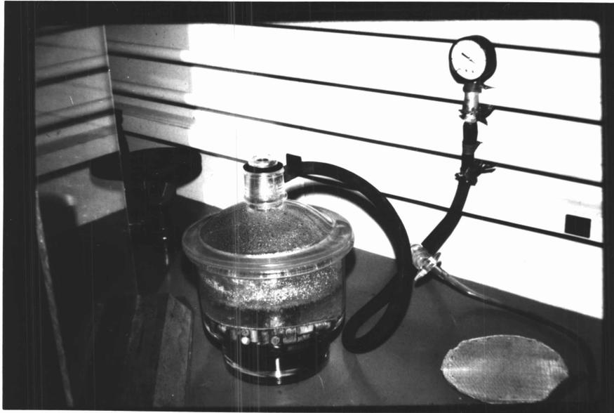
Figure 1. Apparatus for sink-float test.
