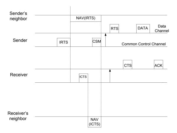
Figure 3.3: Sequence diagram for *iMAC* protocol.
