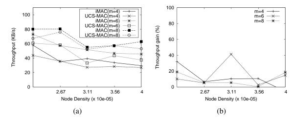
Figure 4.4: (a) Throughput with *iMAC* and UCS-MAC, and (b) throughput gain of *iMAC* over UCS-MAC, as a function of N and hence the node density for different values of m.  $\eta = 0.471$ , A = 1500m  $\times$  1500m, average hop length is between 4 and 5.
