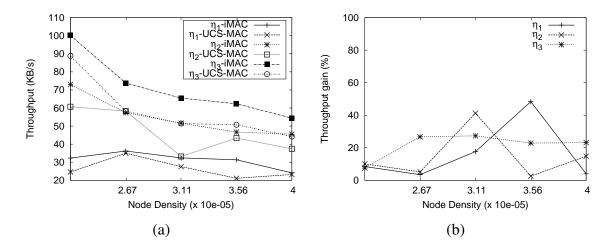
Figure 4.3: (a) Throughput with iMAC and UCS-MAC, and (b) throughput gain of iMAC over UCS-MAC, as a function of N and hence the node density for different values of  $\eta$ . m = 6,  $A = 1500 \, \mathrm{m} \times 1500 \, \mathrm{m}$ , average hop length is between 4 and 5. of load in the range (0,1), and in each case consider three different values for m—4, 6, and 8.
