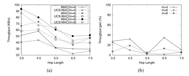
Figure 4.6: (a) Throughput with iMAC and UCS-MAC, and (b) throughput gain of iMAC over UCS-MAC, as a function of average hop lengths for different values of m.  $\eta = 0.471$ , A and N are varied for every hop length.
