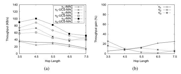
Figure 4.5: (a) Throughput with iMAC and UCS-MAC, and (b) throughput gain of iMAC over UCS-MAC, as a function of average Hop Length for different values of  $\eta$ . m = 6, A and N are varied for every hop length.
