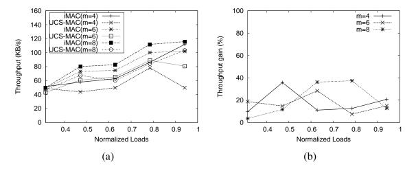
Figure 4.2: (a) Throughput with *iMAC* and UCS-MAC, and (b) throughput gain of *iMAC* over UCS-MAC, as a function of  $\eta$  for different values of m. N = 50, A = 1500m  $\times$  1500m, average hop length is between 4 and 5.
