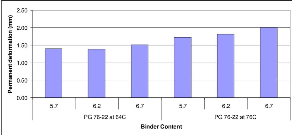
Figure 4.16 Effect of Binder content in permanent deformation
