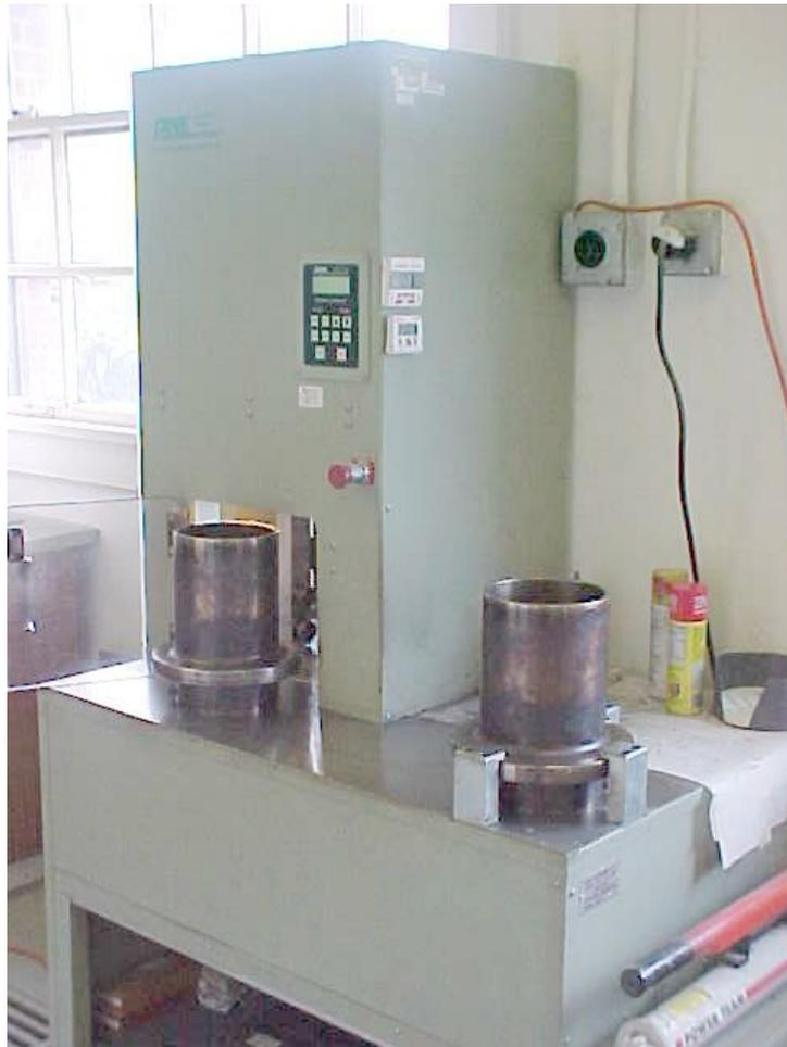
Figure 5.1 Superpave Gyratory Compactor
