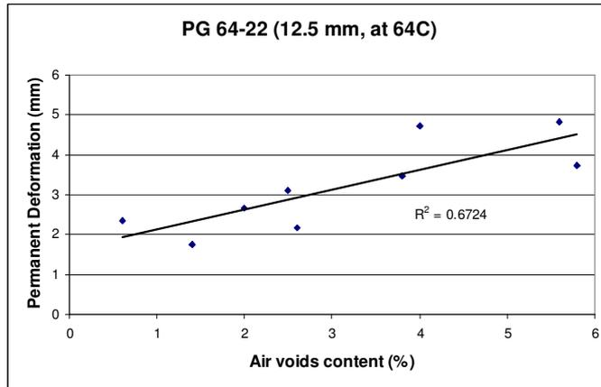
Figure 3.15 Effect of air voids on permanent deformation
