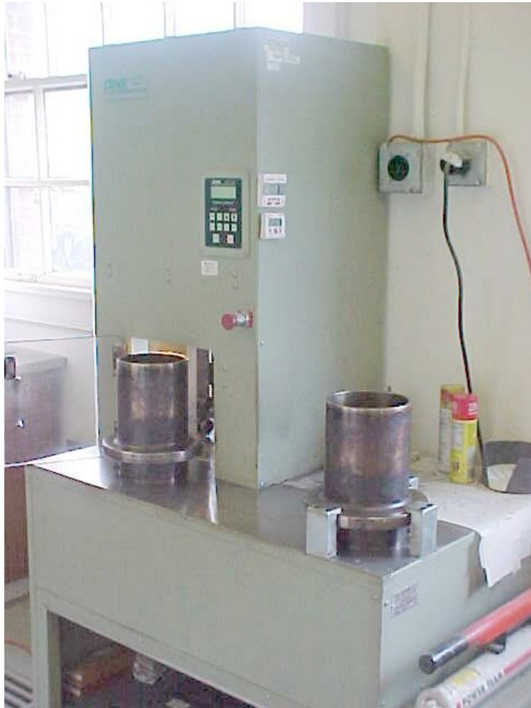
Figure 4.1 Superpave Gyratory Compactor
