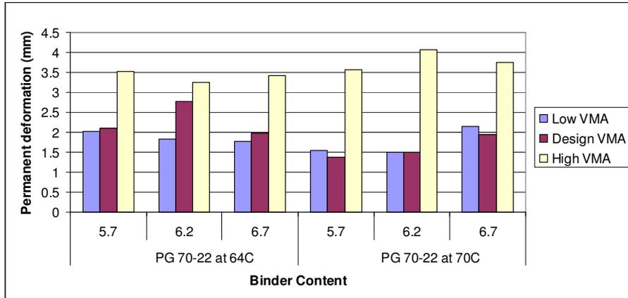
Figure 4.13 Effect of Binder content and VMA in permanent deformation
