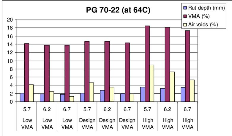
Figure 4.2 Effect of VMA and air voids on permanent deformation
