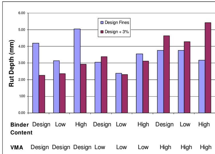
Figure 3.28 Effect of fines content on mean APA rut depths in 19.0 mm mixes
