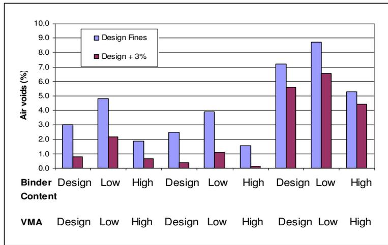
Figure 3.29 Effect of fines content on mean air voids in 19.0 mm mixes
