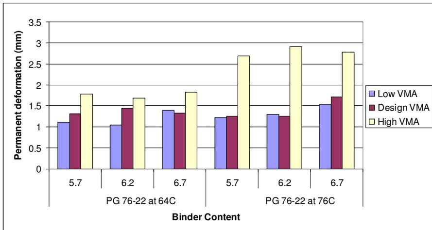
Figure 4.17 Effect of Binder content and VMA in permanent deformation
