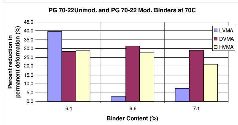
Figure 5.6 Effect of the PG 70-22 Modified asphalt binder in permanent deformation
