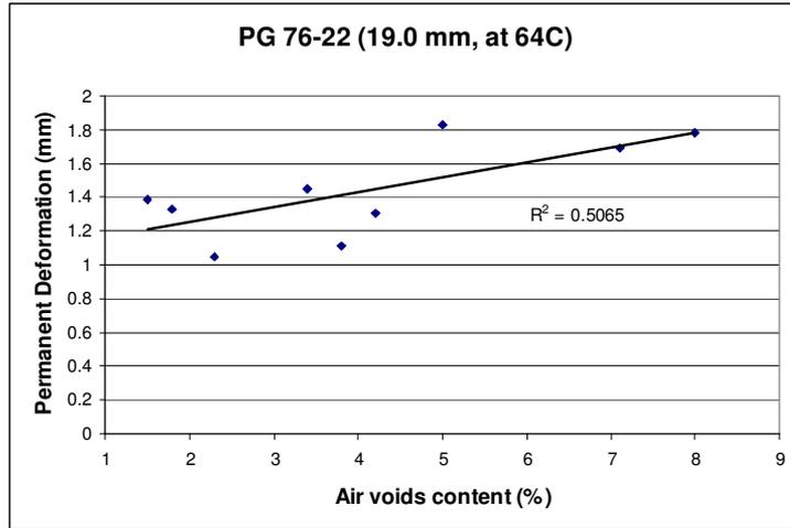
Figure 3.11 Effect of air voids on permanent deformation
