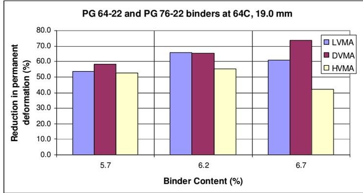
Figure 3.13 Effect of binder type in mixes
