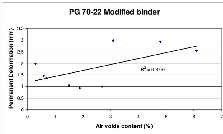
Figure 5.5 Effect of air voids on permanent deformation
