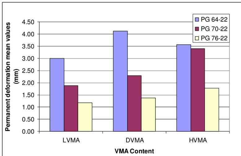
Figure 3.31 Effect of VMA in permanent deformation for 19.0 mm
