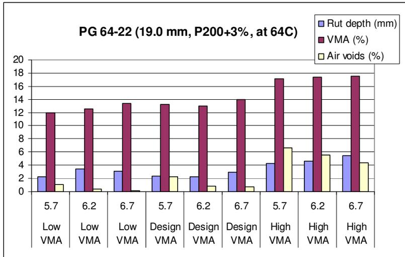
Figure 3.22 Effect of VMA and air voids on permanent deformation
