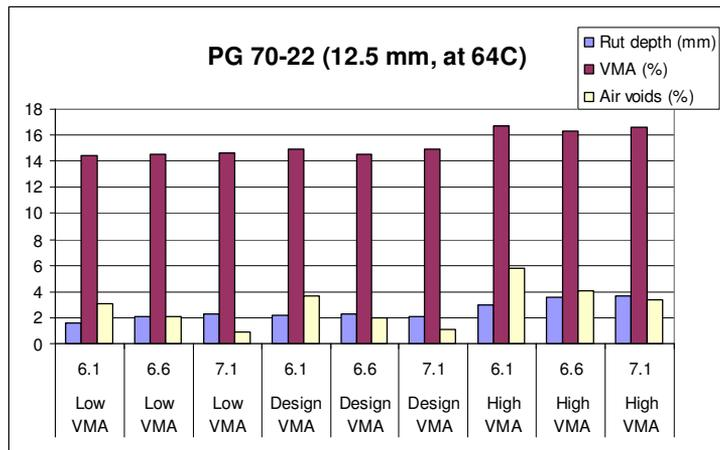
Figure 3.16 Effect of VMA and air voids on permanent deformation
