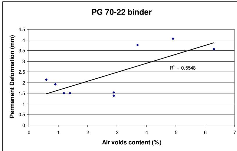
Figure 5.3 Effect of air voids on permanent deformation
