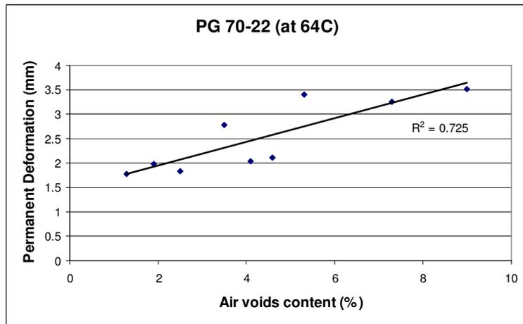
Figure 4.3 Effect of air voids on permanent deformation
