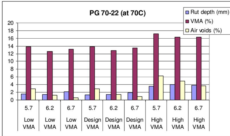
Figure 4.4 Effect of VMA and air voids on permanent deformation
