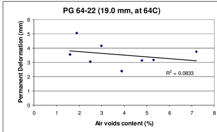
Figure 3.7 Effect of air voids on permanent deformation
