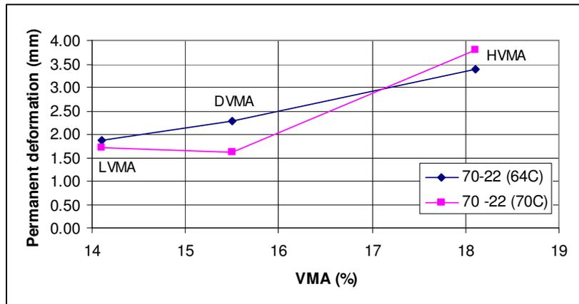
Figure 4.10 Effect of VMA and Test temperature on permanent deformation
