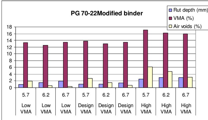
Figure 5.4 Effect of VMA and air voids on permanent deformation
