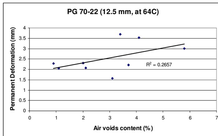
Figure 3.17 Effect of air voids on permanent deformation
