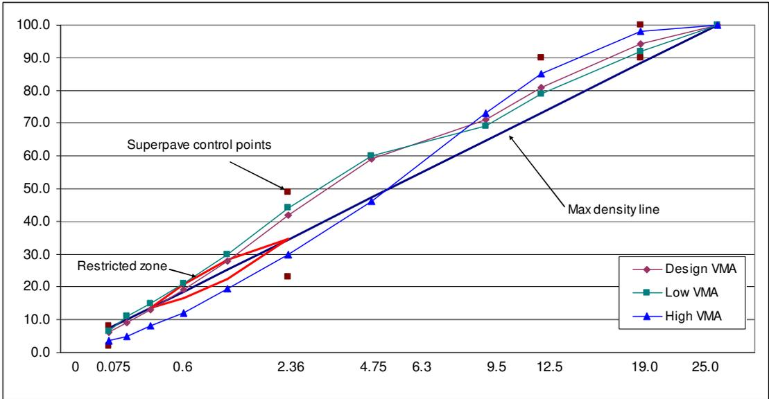
Figure 3.1 Aggregate gradation for the 19.0 mm mixes (Target P200)
