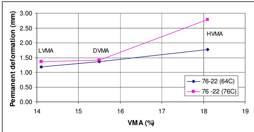
Figure 4.14 Effect of VMA and Test temperature on permanent deformation
