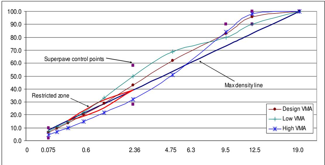
Figure 3.3 Aggregate gradation for the 12.5 mm mixes (Target P200)
