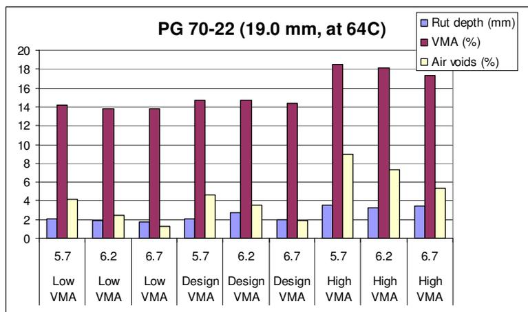
Figure 3.8 Effect of VMA and air voids on permanent deformation
