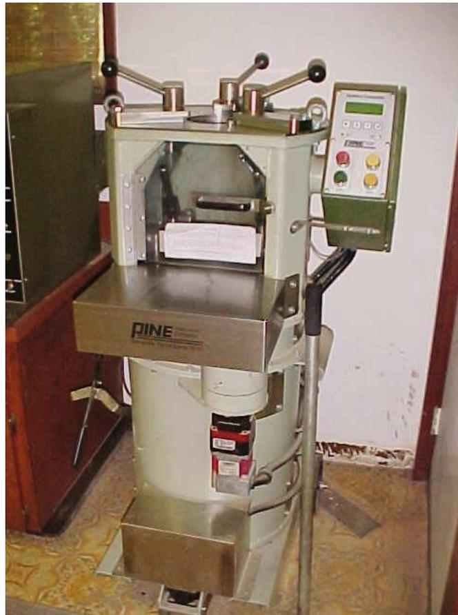
Figure 3.5 Superpave Gyratory Compactor
