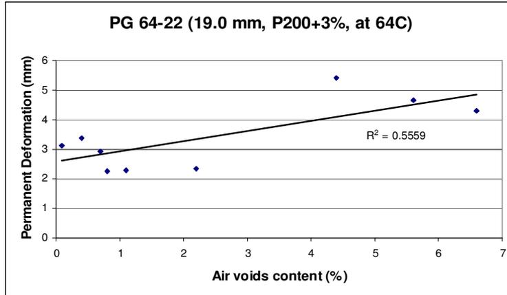
Figure 3.23 Effect of air voids on permanent deformation
