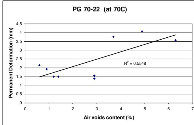
Figure 4.5 Effect of air voids on permanent deformation
