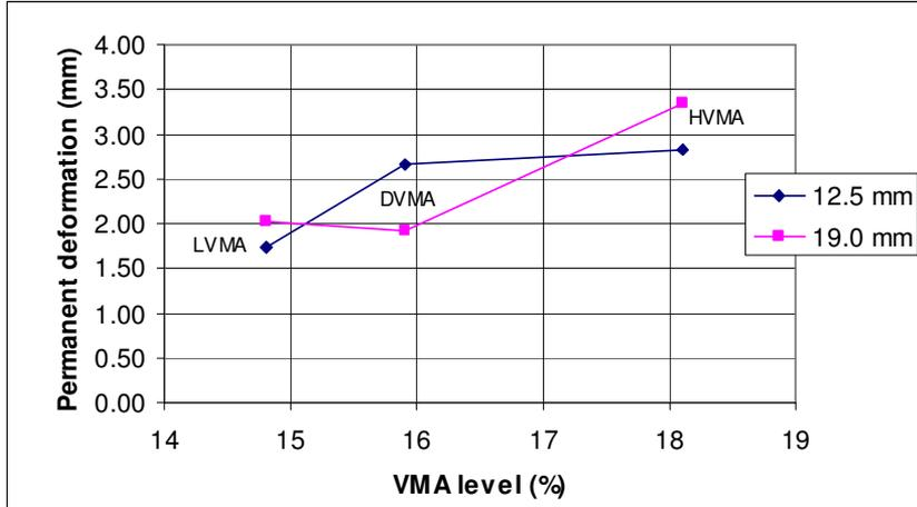
Figure 3.30 Effect of VMA and aggregate size on permanent deformation
