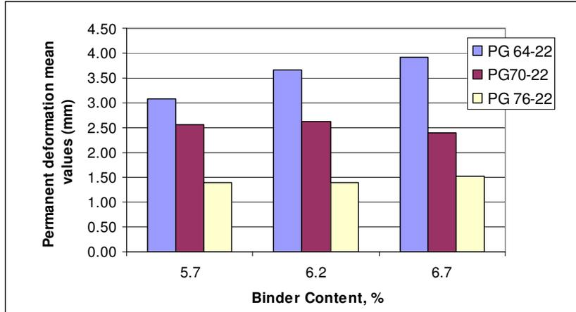
Figure 3.26 Effect of Binder content in permanent deformation for 19.0 mm mixes
