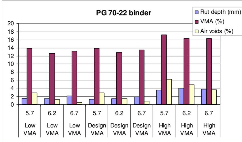
Figure 5.2 Effect of VMA and air voids on permanent deformation
