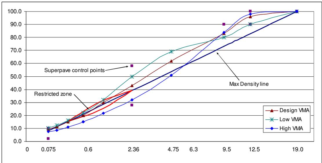
Figure 3.4 Aggregate gradation for the 12.5 mm mixes (Target P200 + 3%)
