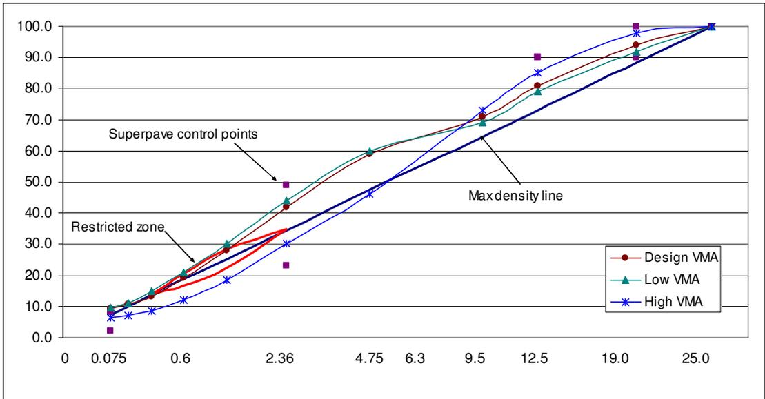
Figure 3.2 Aggregate gradation for the 19.0 mm mixes (Target P200 + 3%)
