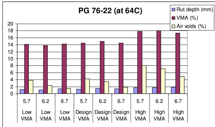
Figure 4.6 Effect of VMA and air voids on permanent deformation
