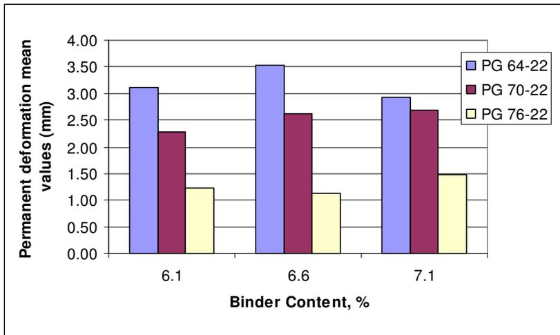
Figure 3.27 Effect of Binder content in permanent deformation for 12.5 mm
