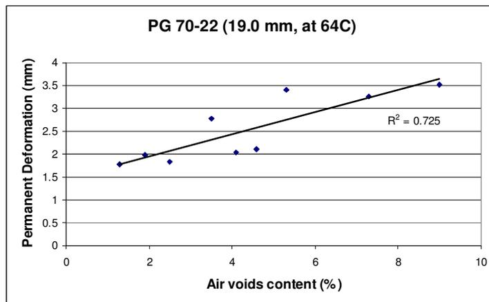
Figure 3.9 Effect of air voids on permanent deformation
