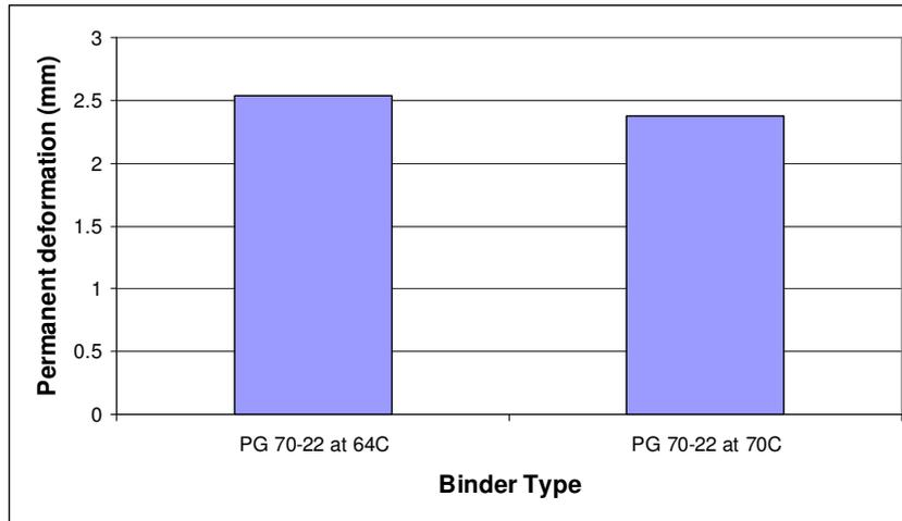
Figure 4.11 Effect of Test temperature on permanent deformation
