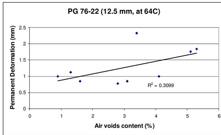
Figure 3.19 Effect of air voids on permanent deformation
