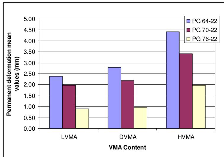
Figure 3.32 Effect of VMA in permanent deformation for 12.5 mm.
