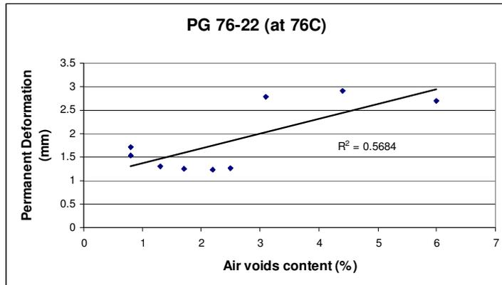
Figure 4.9 Effect of air voids on permanent deformation
