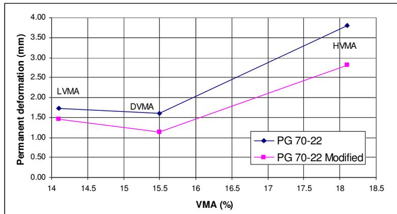
Figure 5.7 Effect of VMA and Test temperature on permanent deformation
