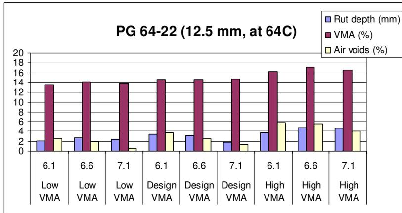
Figure 3.14 Effect of VMA and air voids on permanent deformation
