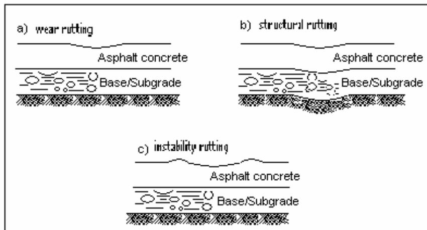
Figure 2.1 Types of permanent deformation (after Dawley et al., 1990)
