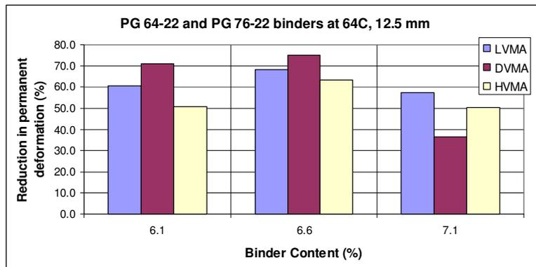
Figure 3.21 Effect of the PG 76-22 asphalt binder
