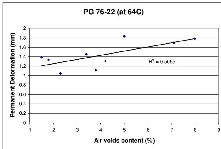
Figure 4.7 Effect of air voids on permanent deformation
