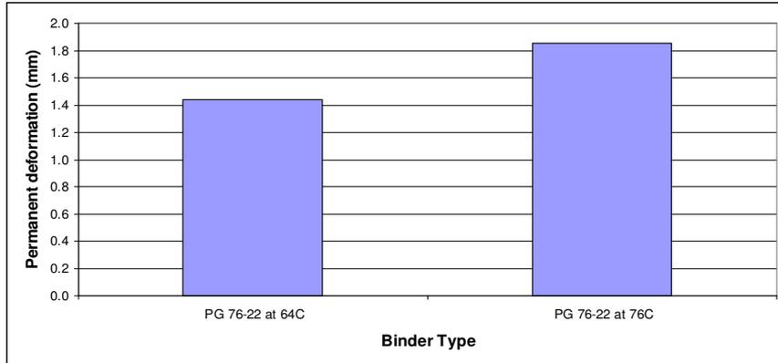
Figure 4.15 Effect of Test temperature on permanent deformation
