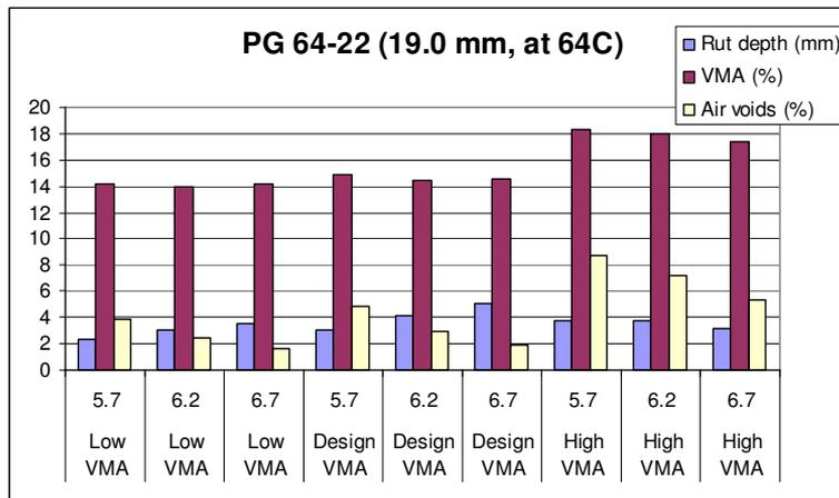
Figure 3.6 Effect of VMA and air voids on permanent deformation
