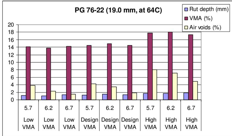
Figure 3.10 Effect of VMA and air voids on permanent deformation
