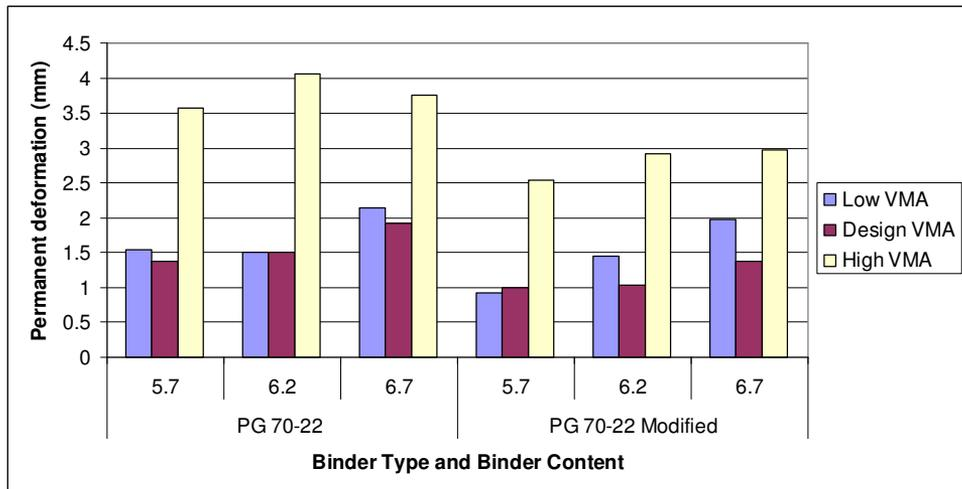
Figure 5.10 Effect of Binder content and VMA on permanent deformation
