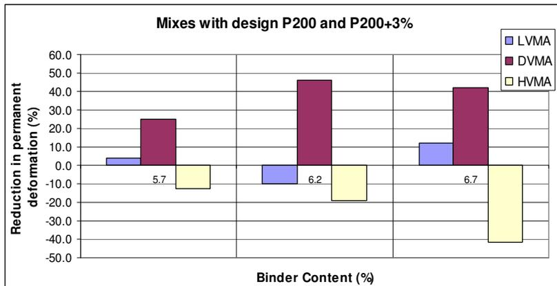
Figure 3.24 Effect of extra P200 on permanent deformation
