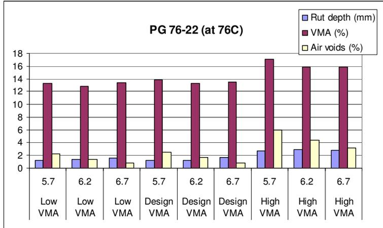
Figure 4.8 Effect of VMA and air voids on permanent deformation
