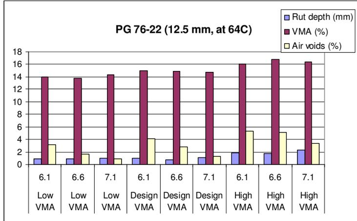
Figure 3.18 Effect of VMA and air voids on permanent deformation
