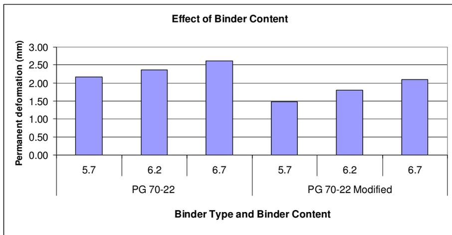
Figure 5.9 Effect of Binder content in permanent deformation
