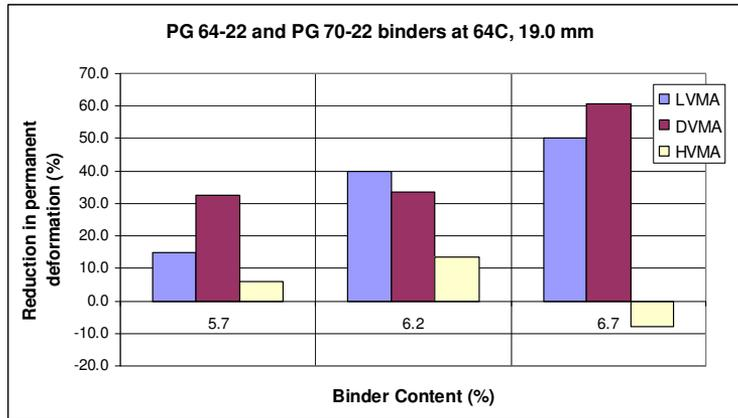
Figure 3.12 Effect of binder type in mixes
