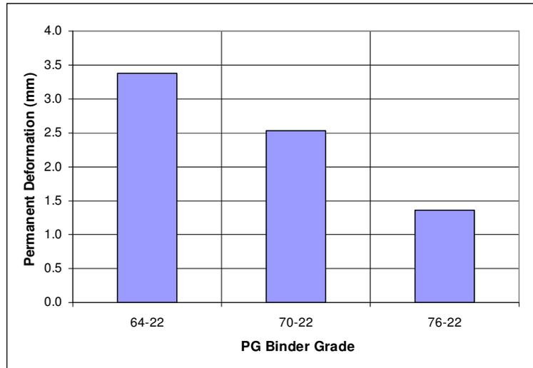
Figure 3.25 Effect of Binder type on permanent deformation
