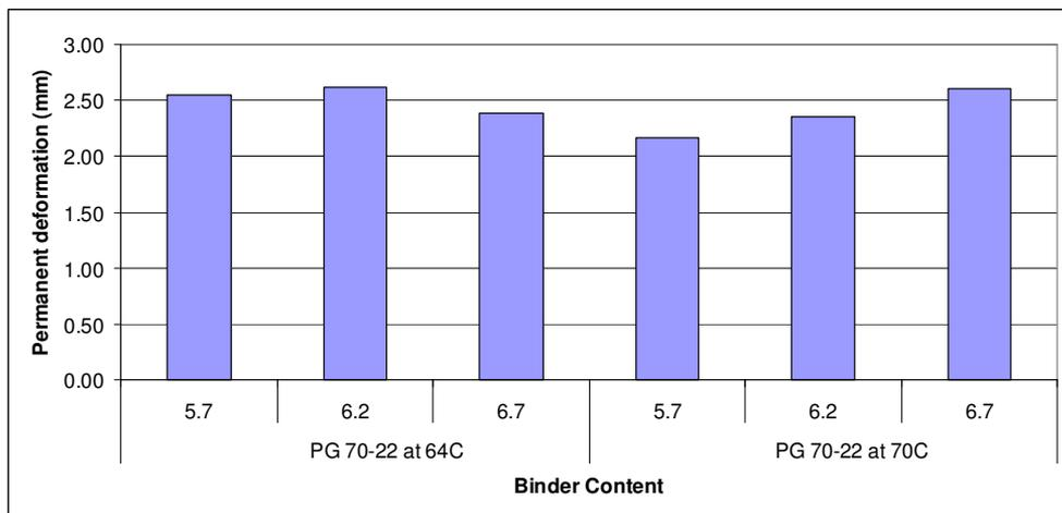
Figure 4.12 Effect of Binder content in permanent deformation
