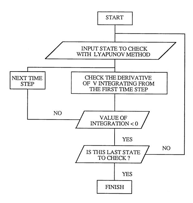
Figure 4.1 Flow Chart for Numerical Procedures.
