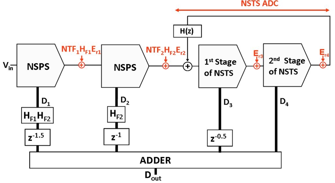
Figure 5.8: Modeling inter-stage errors in the proposed architecture
