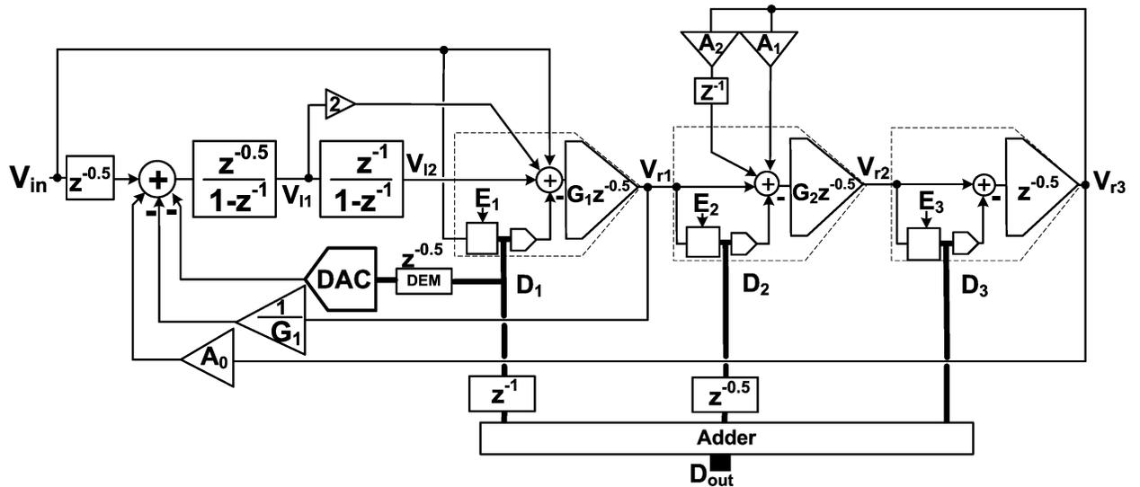
Figure 3.11: The implemented third order HDSP modulator
