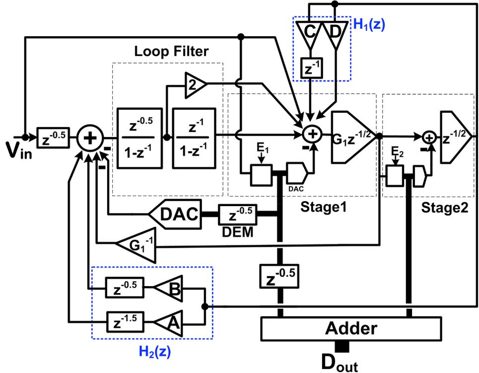
Figure 4.20: The detailed realization of the enhanced HDSP ADC
