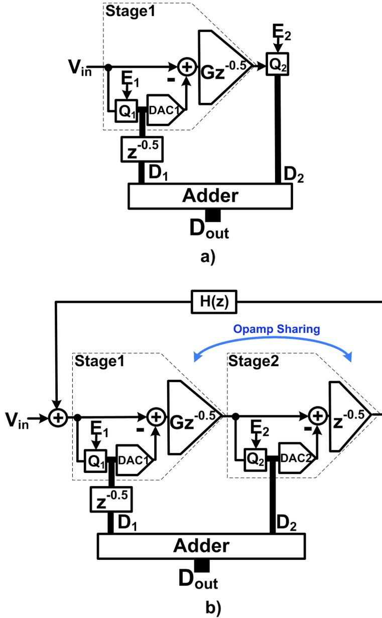
Figure 4.1: a) Traditional two-step quantizer b) The proposed NSTS quantizer
