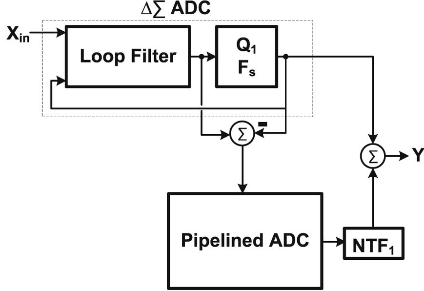
Figure 2.3: The cascaded  $\Delta\Sigma$ -pipelined ADC
