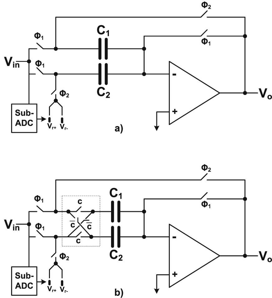
Figure 2.7: a) Traditional flip-around pipeline MDAC b) The flip-around pipeline MDAC with mismatch shaping scheme
