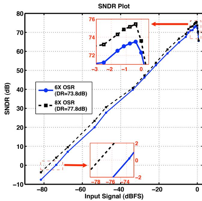
Figure 5.18: The SNDR plot for 8X and 6X OSR
