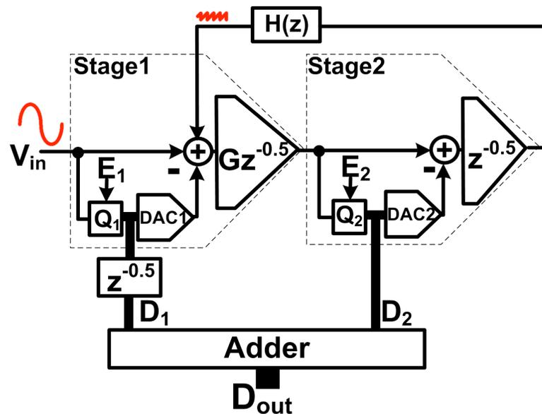
Figure 4.3: The NSTS ADC with the simplified signal addition
