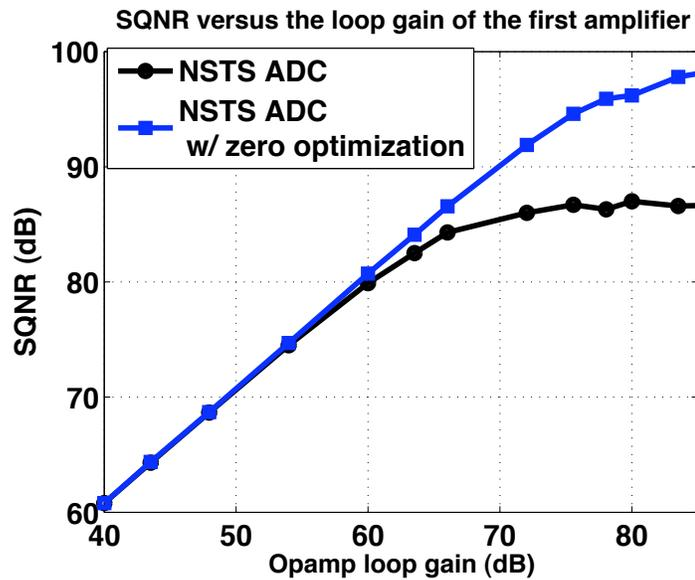
Figure 4.16: The SQNR plot versus the loop gain of the amplifier in the front-end NSTS ADC
