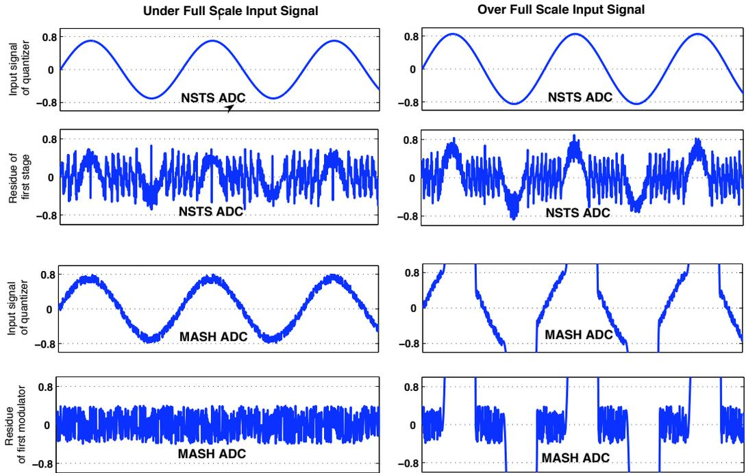
Figure 4.9: The swing of the internal nodes of the MASH and the NSTS ADCs for under and over full scale input signals
