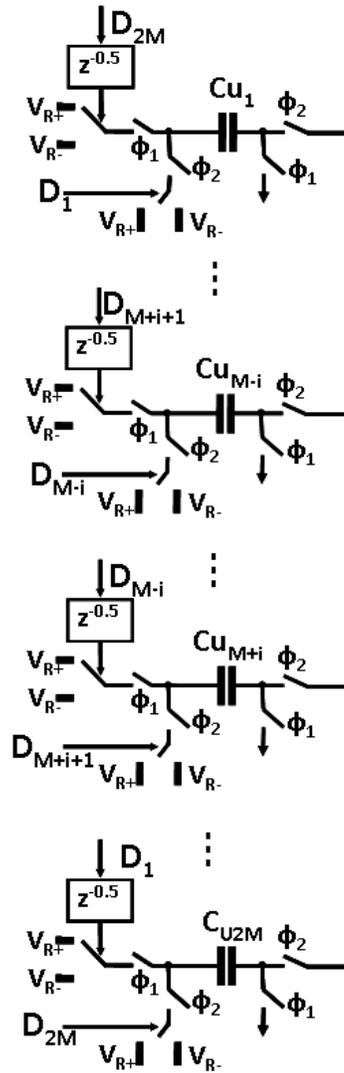
Figure 5.11: The common centroid selection of DAC unit elements
