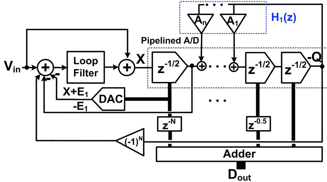
Figure 4.18: The conventional Hybrid Delta-Sigma/Pipelined (HDSP) ADC
