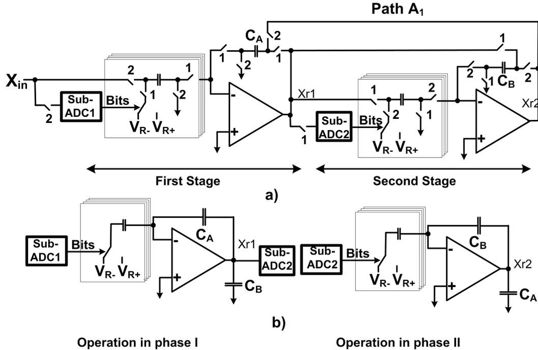
Figure 4.4: The potential circuit realization of the NSTS ADC
