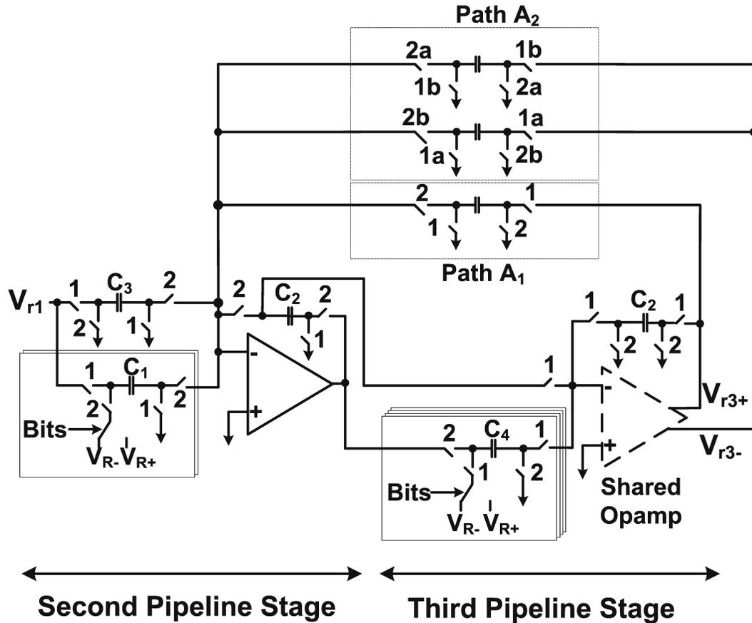
Figure 3.14: The switched-capacitor realization of the second and the third pipelined stages
