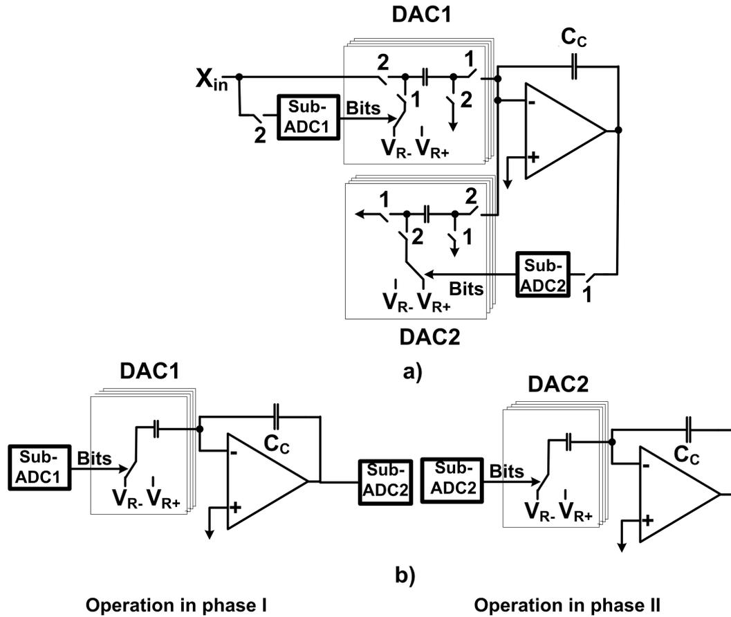
Figure 4.5: The simplified circuit realization of the NSTS ADC
