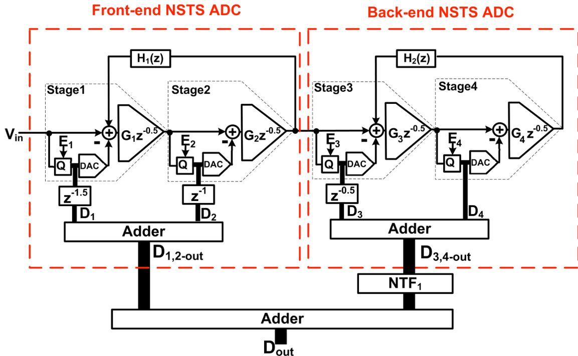
Figure 4.12: The proposed cascaded NSTS ADC
