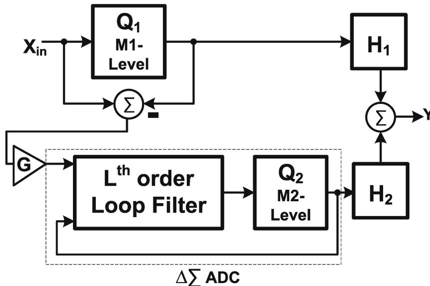
Figure 2.4: The 0- $\Delta\Sigma$  MASH modulator
