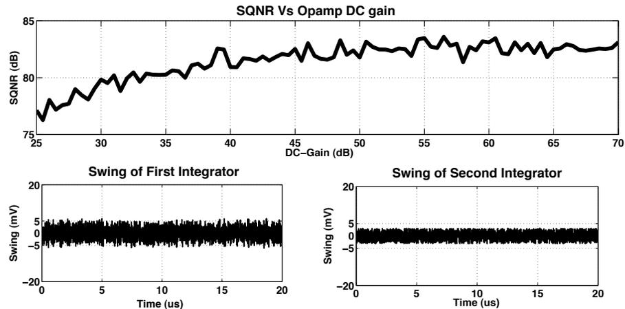
Figure 3.7: The gain and swing requirements of the loop filter integrators (Full scale =  $\pm 800\text{mV}$ )
