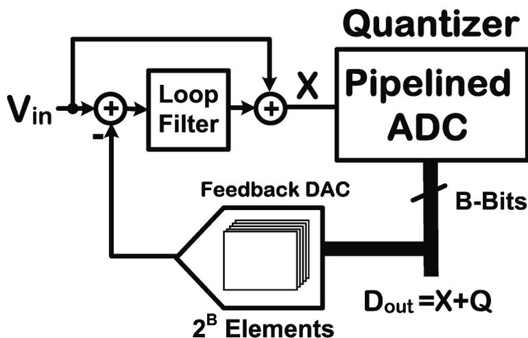
Figure 3.1: A potential/problematic DSM with a pipelined ADC as quantizer
