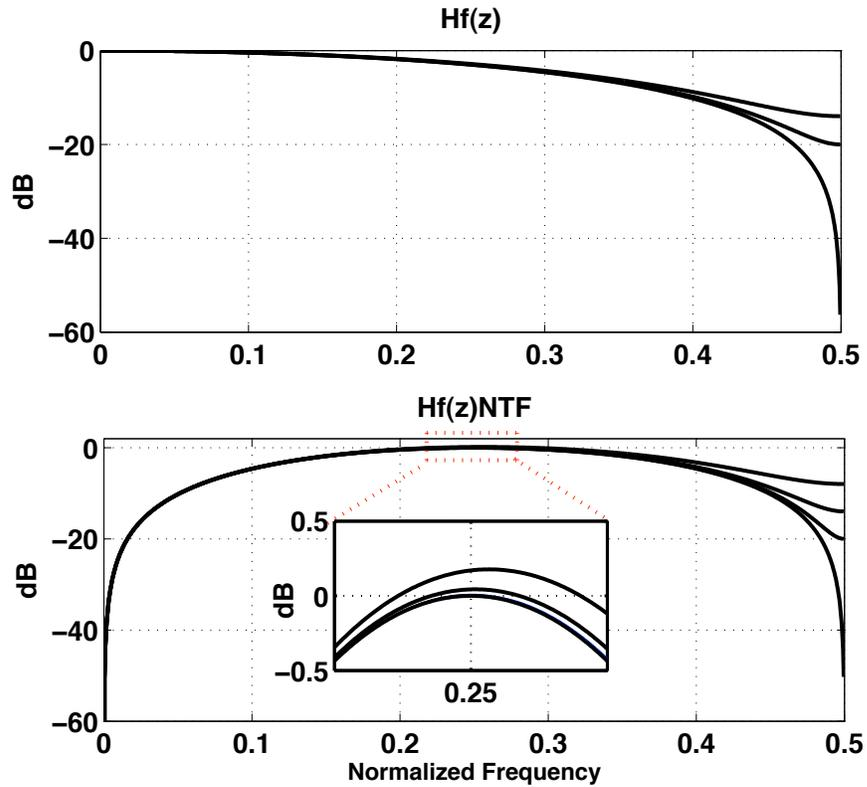
Figure 5.6: Effect of mismatch between filter coefficients on the filter transfer function and the transfer function of NSPS output residue
