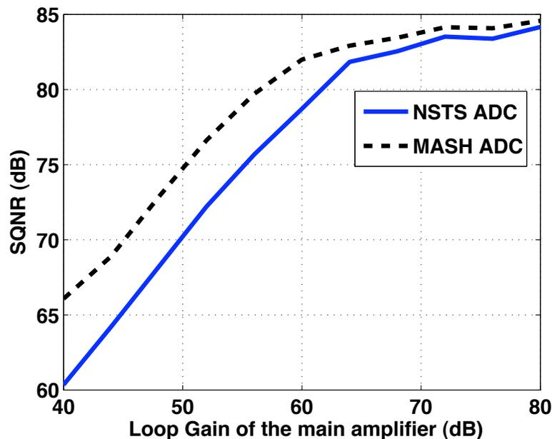
Figure 4.11: The SNDR plot versus the gain of the first integrator in the MASH ADC and the gain of the amplifier in the NSTS ADC
