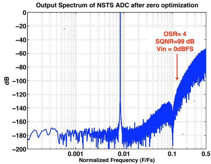
Figure 4.14: The spectrum of the cascaded NSTS ADC after zero optimization
