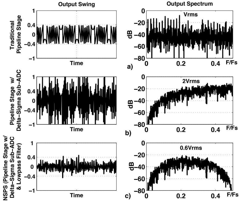
Figure 5.2: The MDAC output voltage and spectrum: a) Traditional pipeline stage; b) Pipeline stage w/ delta-sigma sub-ADC and without low-pass filter c) The proposed NSPS utilizing both delta-sigma sub-ADC and low-pass filter
