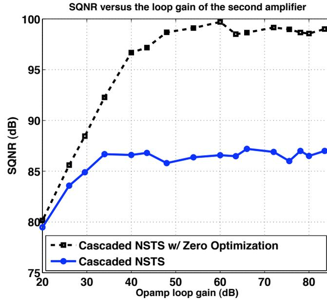
Figure 4.17: The SQNR plot versus the loop gain of the amplifier in the back-end NSTS ADC
