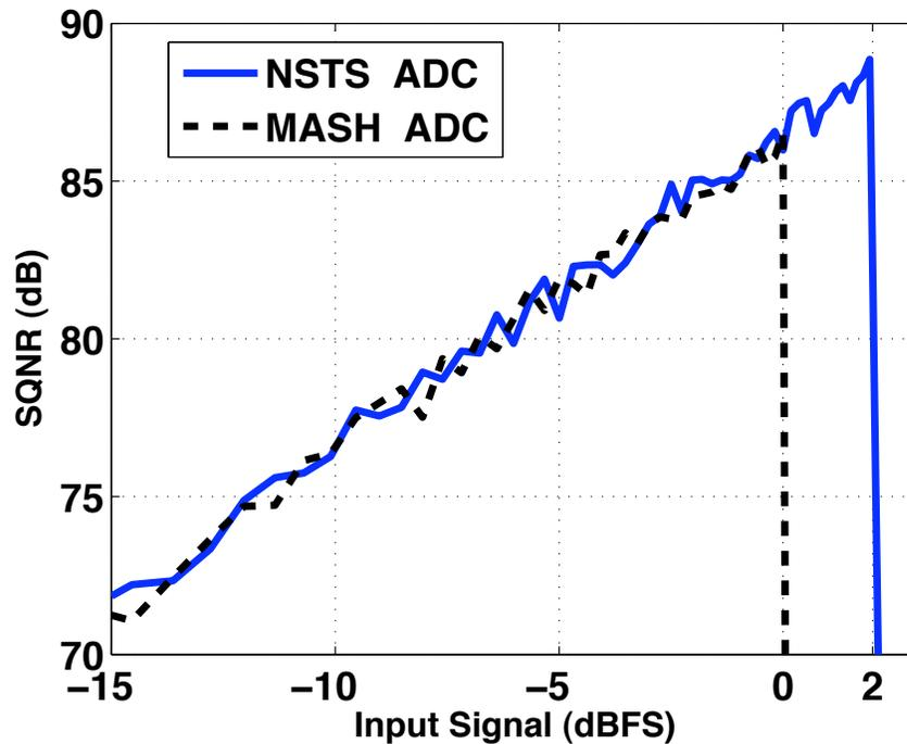
Figure 4.10: The SNDR plot versus the input signal in the MASH and the NSTS ADCs
