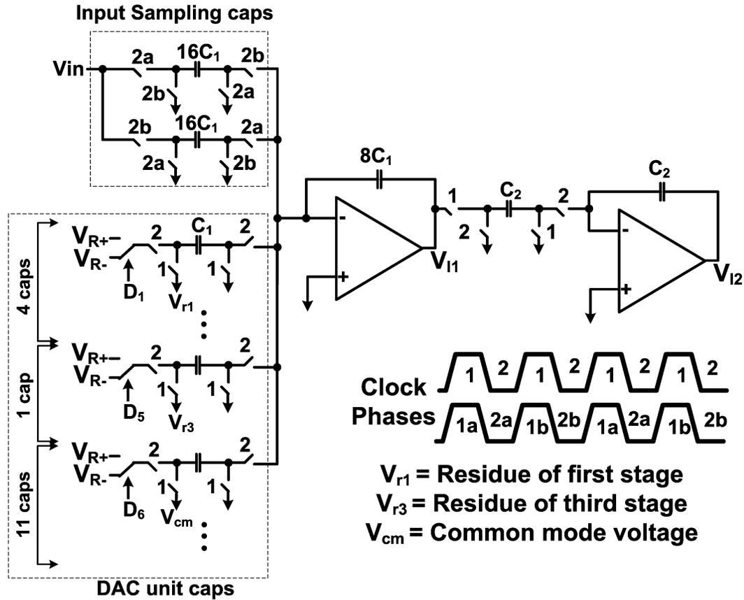
Figure 3.12: The switched-capacitor realization of the loop filter
