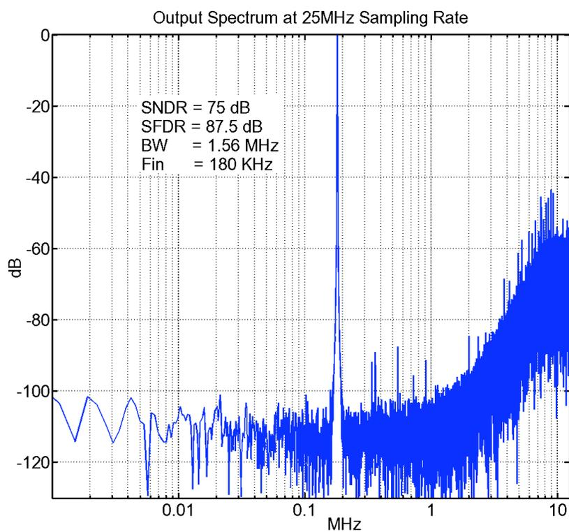
Figure 4.23: The output spectrum of the ADC
