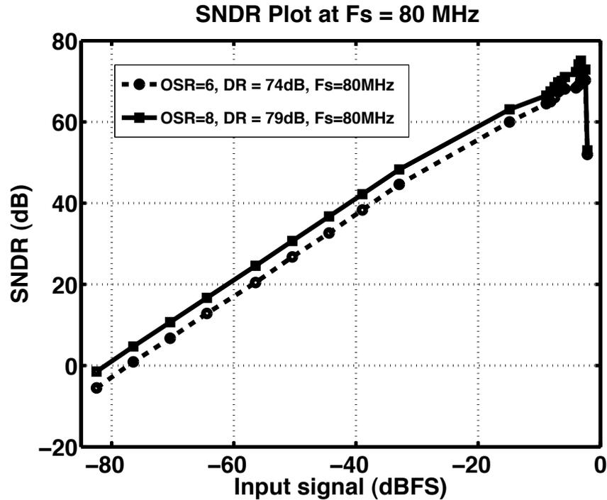
Figure 3.18: SNDR plot at 80 MHz sampling rate
