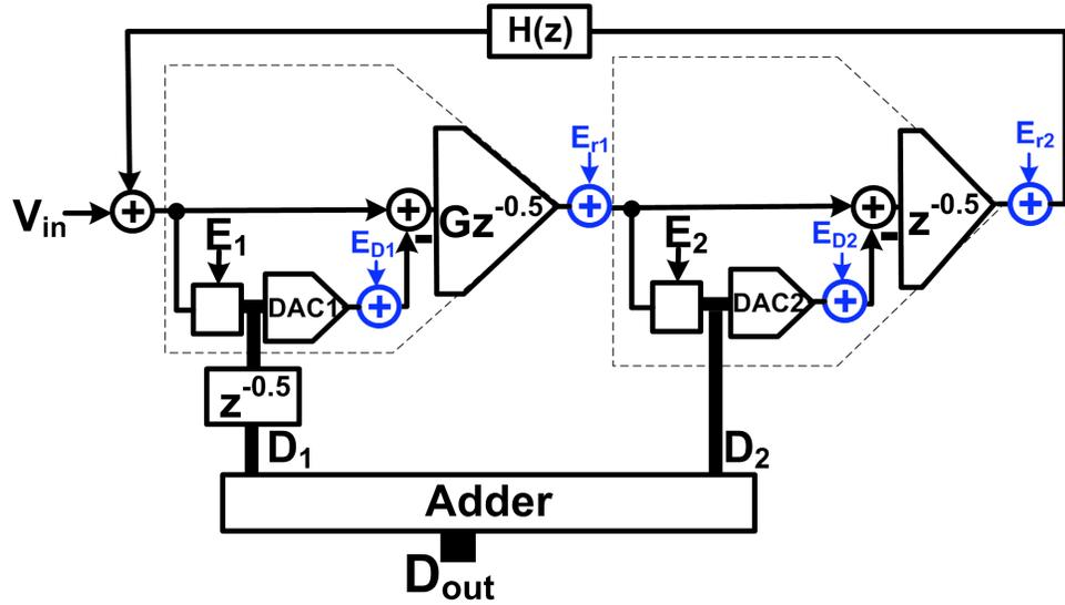
Figure 4.2: Opamp and DAC error modeling in NSTS ADC
