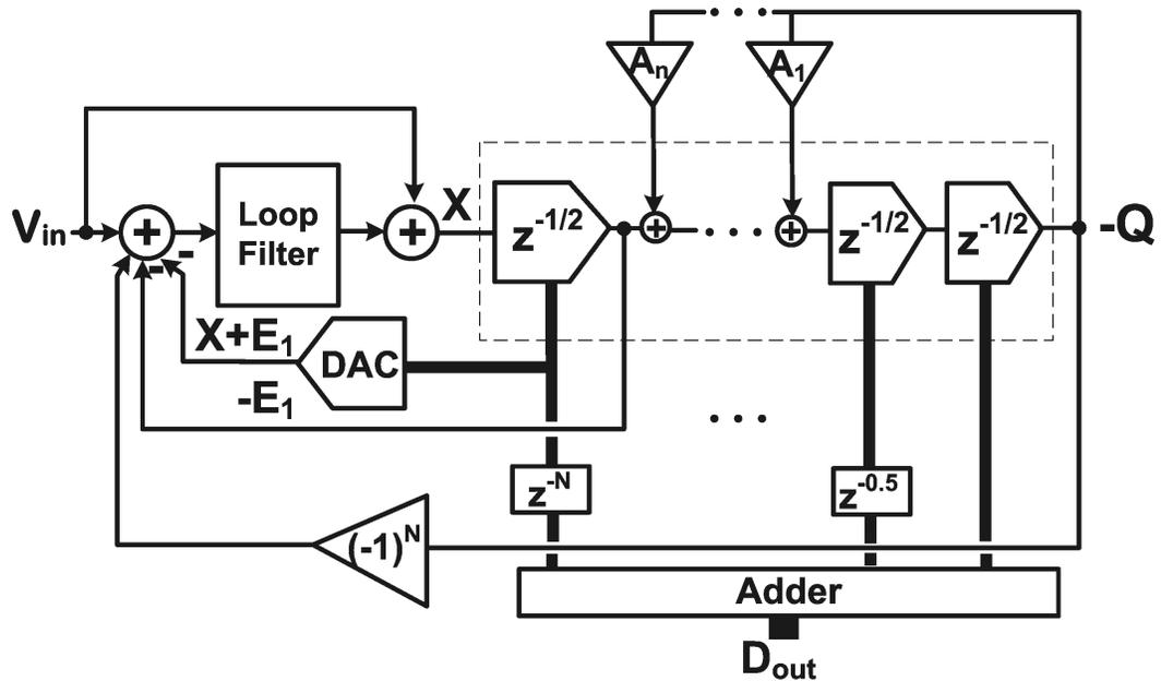
Figure 3.5: The proposed Hybrid Delta-Sigma/Pipelined (HDSP) Modulator
