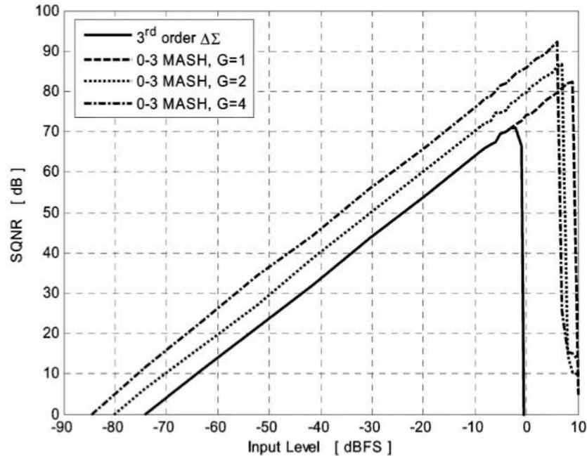
Figure 2.5: The SNDR plot of 0-3 MASH modulator with various inter-stage gains (1,2 and 4)
