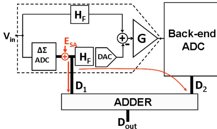
Figure 5.5: Modeling sub-ADC errors in NSPS
