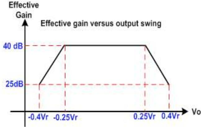
Figure 5.4: Gain of the opamp used in Fig. 5.3 vs output swing of the opamp
