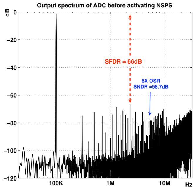
Figure 5.16: The output spectrum of the ADC before activating the NSPS
