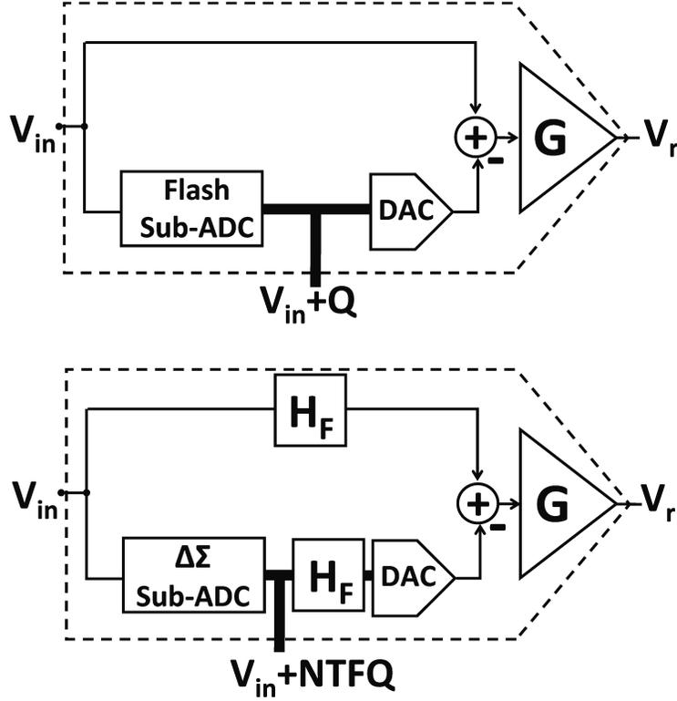
Figure 5.1: Front-end stages in a pipelined ADC: a) conventional stage; b) the proposed noise-shaped pipeline stage (NSPS)
