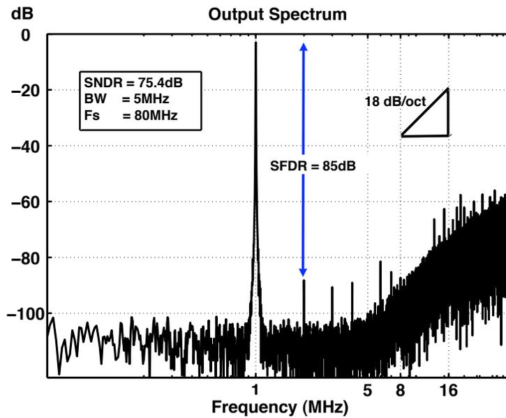
Figure 3.16: The output spectrum at 80 MHz sampling rate (32K points FFT)
