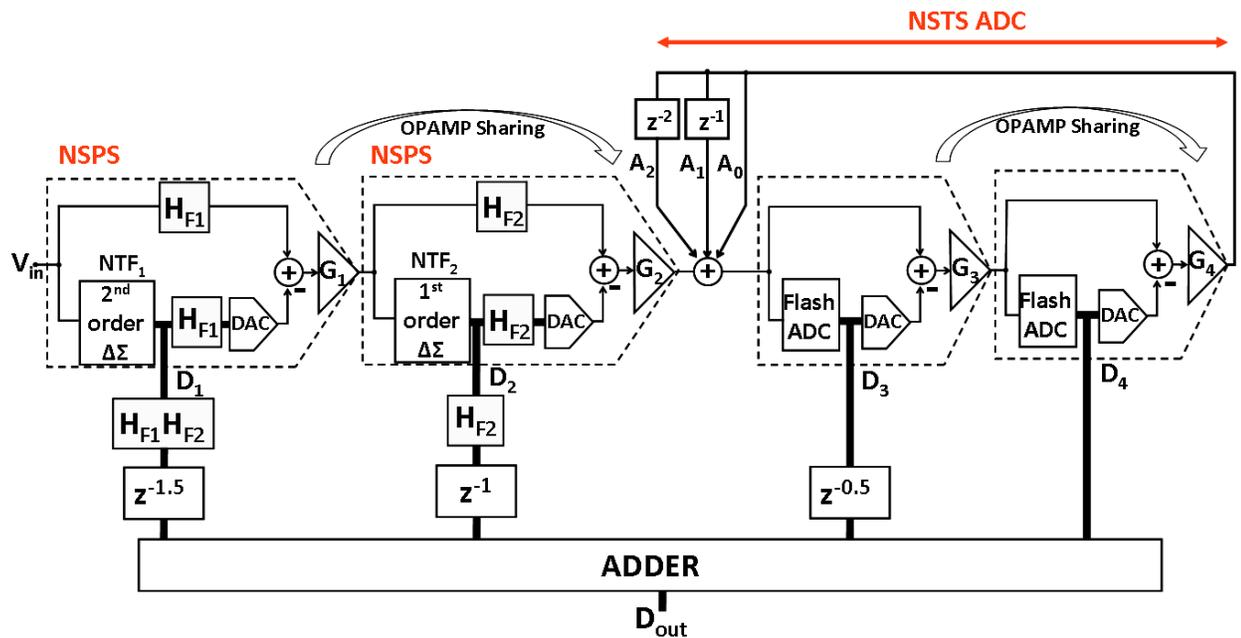
Figure 5.7: The proposed noise-shaped pipelined ADC
