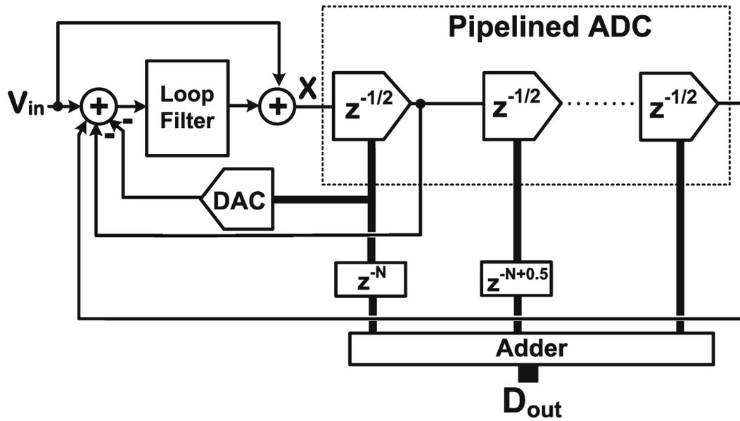
Figure 3.4: Latency in the  $\Delta\Sigma$  modulator with a pipelined ADC as quantizer
