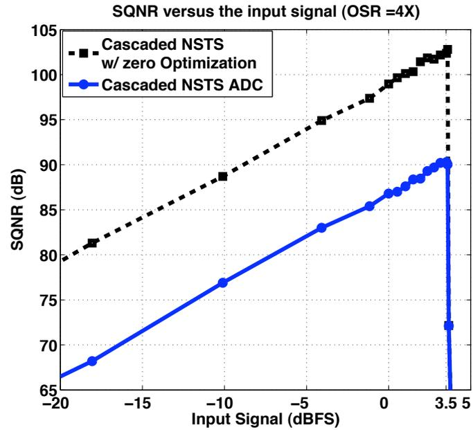
Figure 4.15: The SQNR plot of the cascaded NSTS ADC versus input signal (dBFS)
