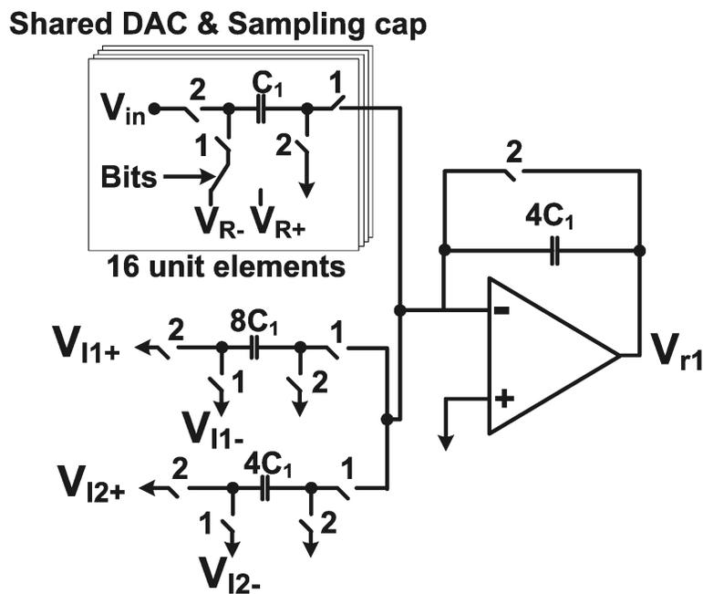
Figure 3.13: The switched-capacitor realization of the first pipelined stage
