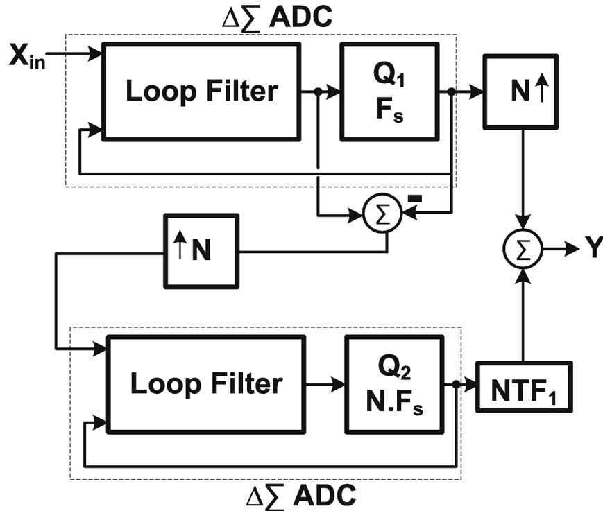
Figure 2.6: The multi-rate MASH modulator
