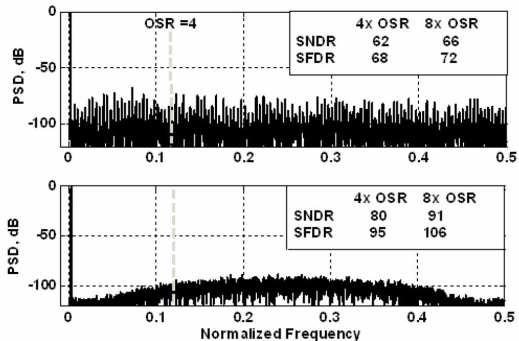
Figure 5.3: Output spectrum of ADC with traditional and NSPS front-end stages (Nonlinear gain is assigned to opamp)
