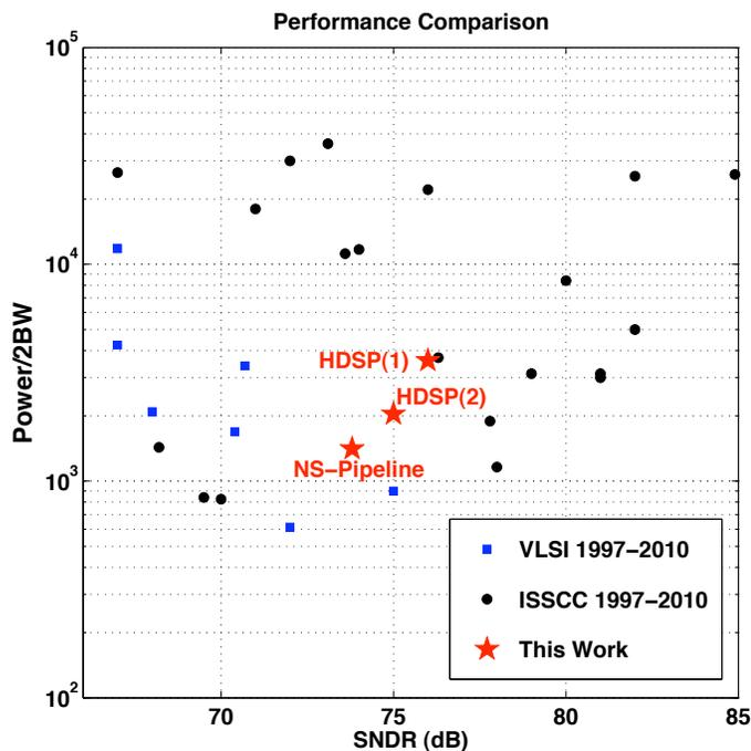
Figure 6.1: Comparing performance of the proposed architectures with the state of the art ADCs ( $\frac{Power}{2BW}$  vs SNDR)
