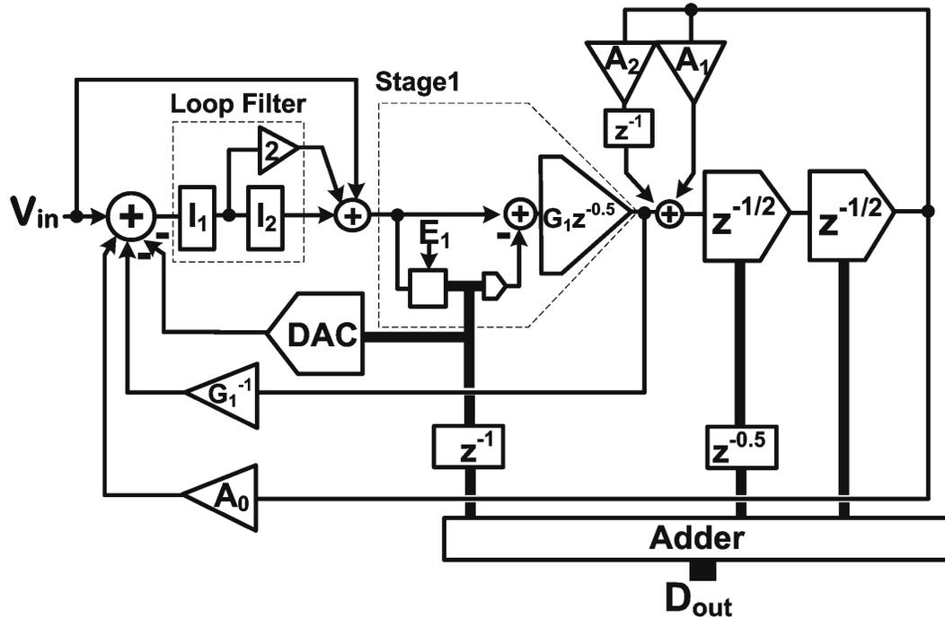
Figure 3.9: Third order HDSP modulator using second order loop filter and three stage pipelined quantizer
