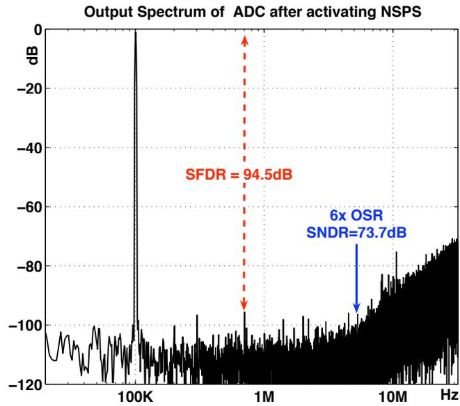
Figure 5.17: The output spectrum of the ADC after activating the NSPS
