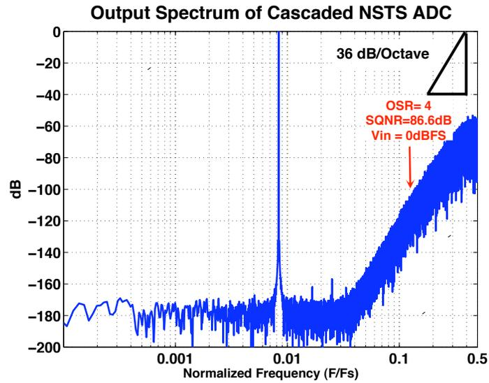
Figure 4.13: The spectrum of the cascaded NSTS ADC
