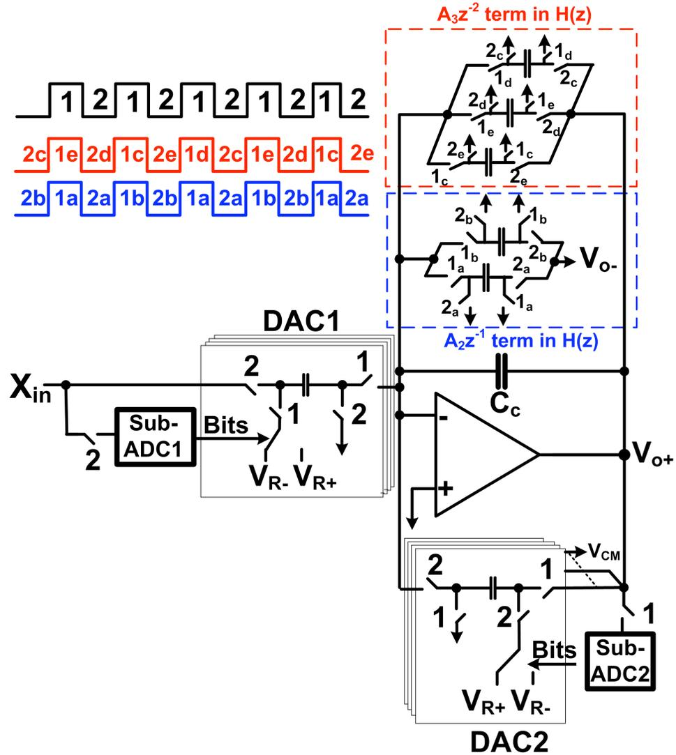
Figure 4.7: The circuit realization of the third-order NSTS ADC
