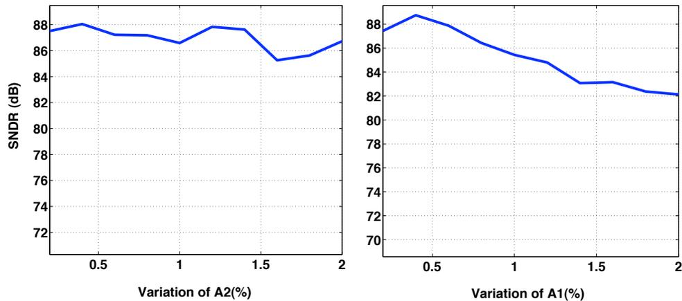
Figure 3.6: Sensitivity to the analog feedback coefficients,  $A_1$  and  $A_2$  in ( 3.11)
