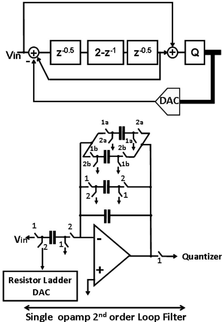
Figure 5.13: The system level and circuit level realization of the second-order delta-sigma sub-ADC
