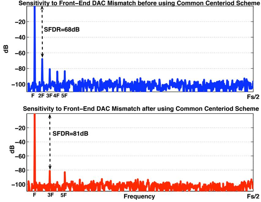
Figure 5.12: The DAC nonlinearity suppression achieved by using common centriod scheme
