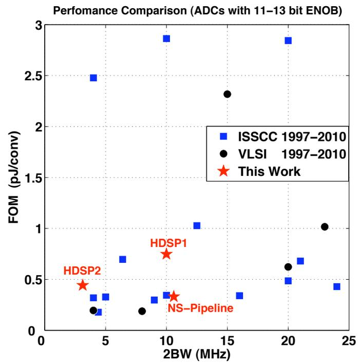
Figure 6.2: Comparing performance of the proposed architectures with the state of the art ADCs (FOM vs. BW)
