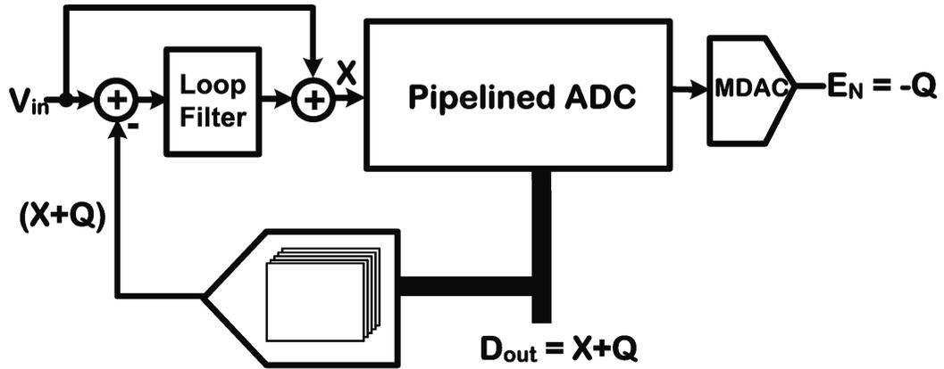
Figure 3.2: Extracting the pipelined quantization noise  $Q$  in analog form
