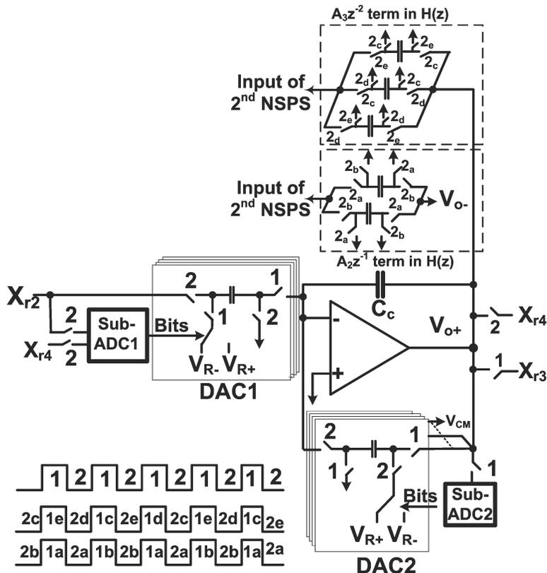
Figure 5.14: The circuit realization of the back-end NSTS ADC
