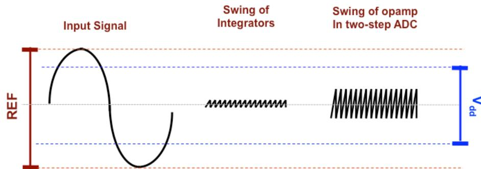
Figure 4.21: The swing of internal nodes of the enhanced HDSP modulator
