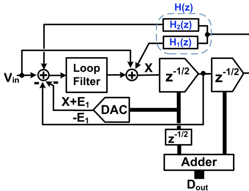
Figure 4.19: The enhanced HDSP ADC using the NSTS quantizer
