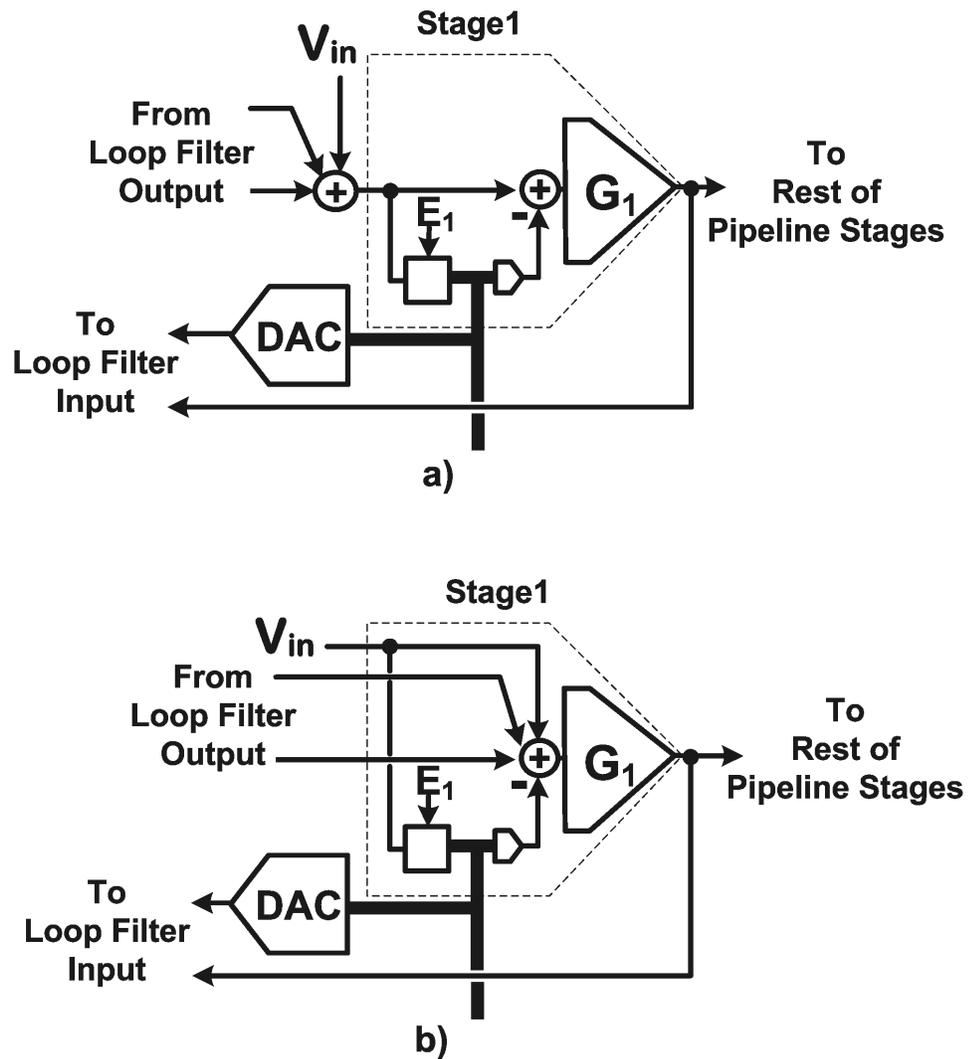
Figure 3.10: a) Signal addition at input of both sub-ADC and the residue amplifier
