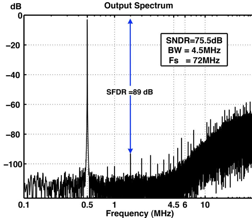
Figure 3.17: The output spectrum at 72 MHz sampling rate (64K points FFT)
