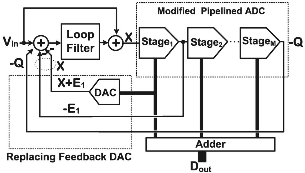
Figure 3.3: Replacing the feedback DAC in DSM with a pipelined ADC as quantizer
