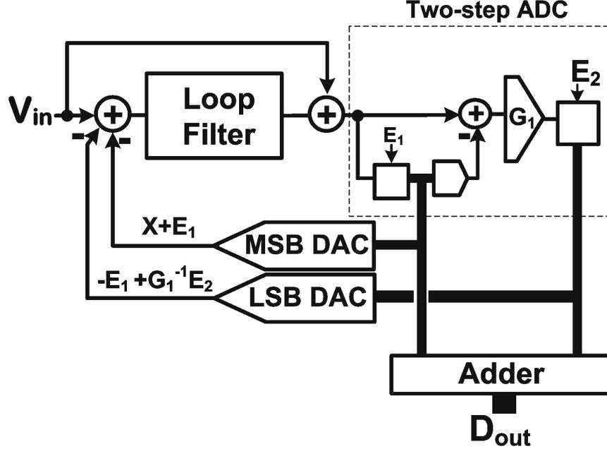
Figure 2.1: The single-loop  $\Delta\Sigma$  ADC with Two-Step quantizer
