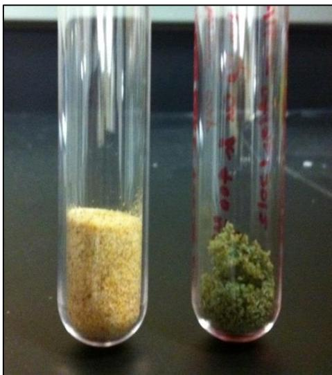
**Figure . Sieved Apatite II<sup>TM</sup> media before (left) and after column experiment (right)**
