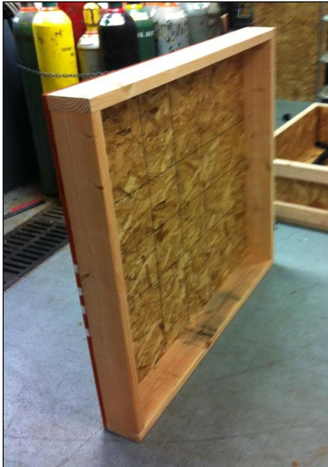
**Figure . Constructed filter lid**
