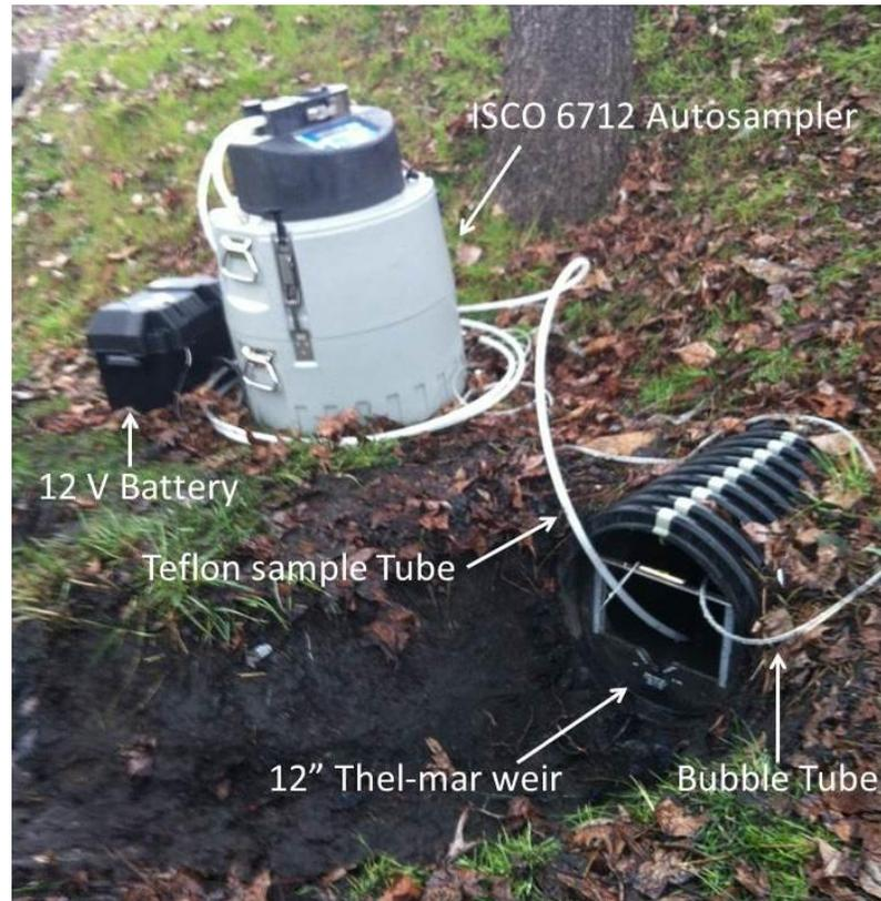
**Figure . Highway 22 sampling installation**
