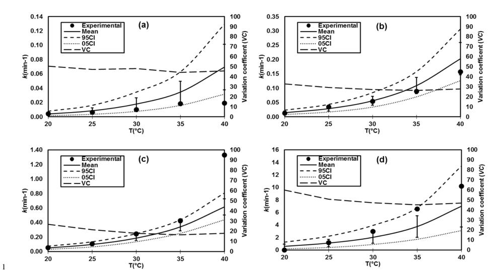
Figure 1. Simulation of PME inactivation rate constants with the Monte Carlo method: (a) 100 MPa; (b) 200 MPa; (c) 300 MPa; (d) 500
