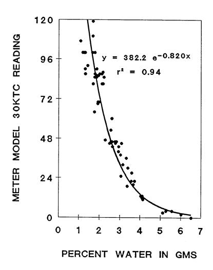
Figure 4. Soil drying GMS. Relationship of GMS resistance recorded with meter model 30KTC to percent water in GMS during a drying cycle in field soil.
