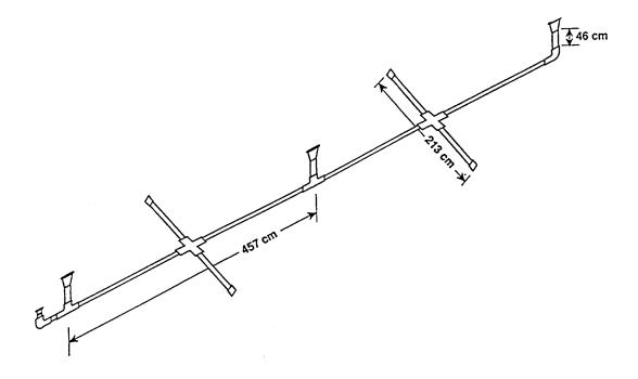
Figure 1. Assembled plot sprinkler apparatus. The schematic view of an assembled portable plot sprinkler shows the relationships among the components listed on Table 1.
