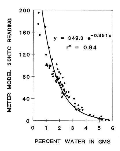
Figure 3. Oven drying GMS. Relationship of GMS resistance recorded with meter model 30KTC to percent water in GMS during an oven drying cycle.
