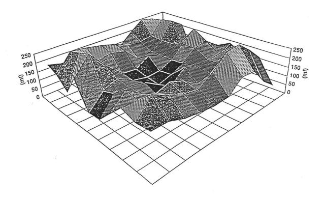
Figure 2. 836C distribution pattern. Water distribution from a single 836C square-pattern sprinkler head located in the center of a grid of 100 catchcans. Each square in the diagram represents a catchcan, darker shading indicates less water.
