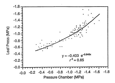
Figure 9. Leaf press and pressure chamber. Relationship of leaf press and pressure chamber estimates of leaf water potential for 124 potato leaflet pairs.
