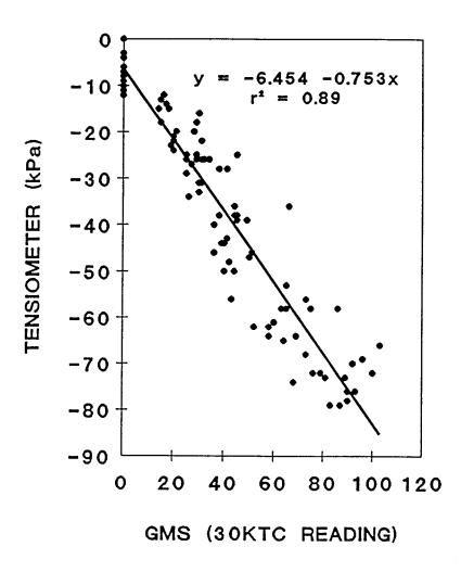
Figure 5. GMS compared to tensiometers. Relationship of GMS meter model 30KTC readings to tensiometer readings from devices installed 15 cm apart in the root zone of potato grown in a silt loam.
