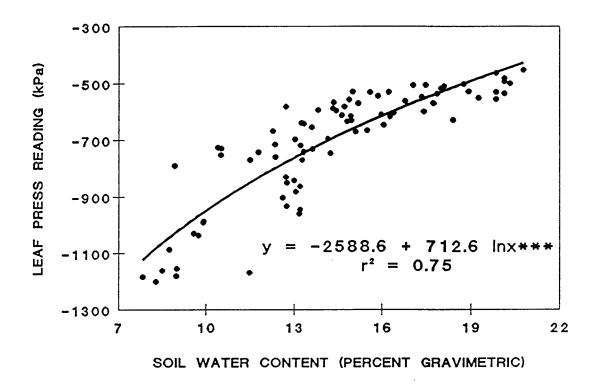
Figure 8. Leaf press and gravimetric. Relationship of leaf press estimates of potato water status to gravimetric soil water percentage.
