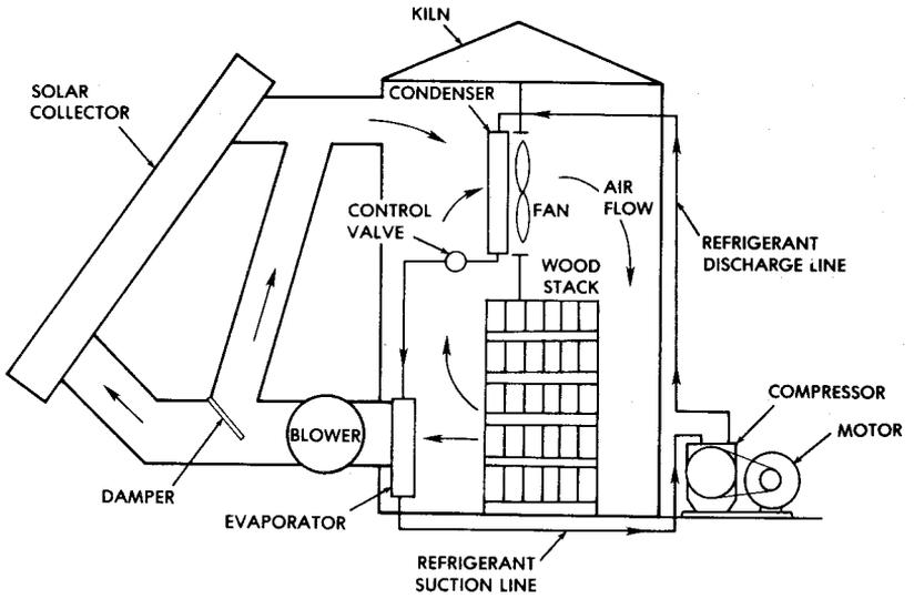
Figure 1.--Solar-dehumidification lumber drying kiln.
