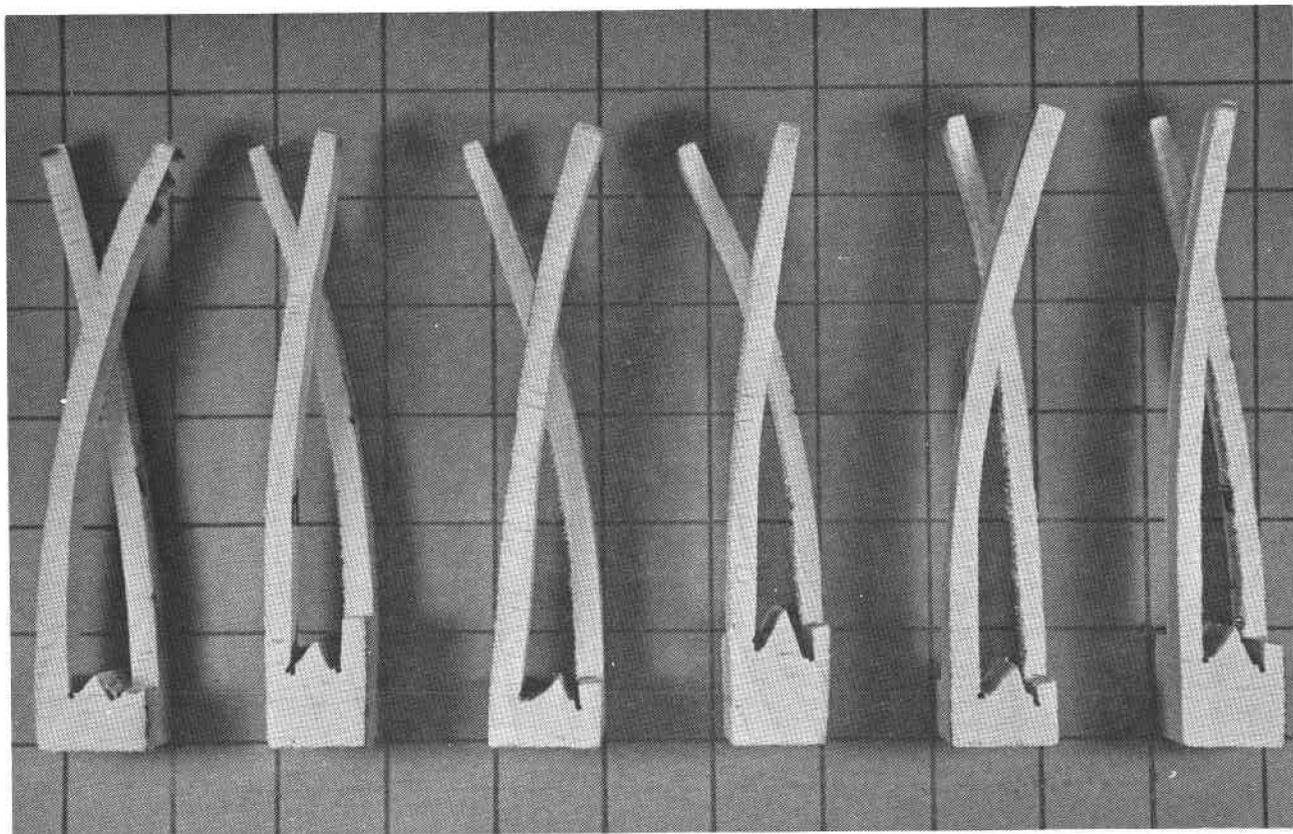
Figure 3.--Demonstration of internal stresses remaining in solar-dehumidifier dried lumber.
