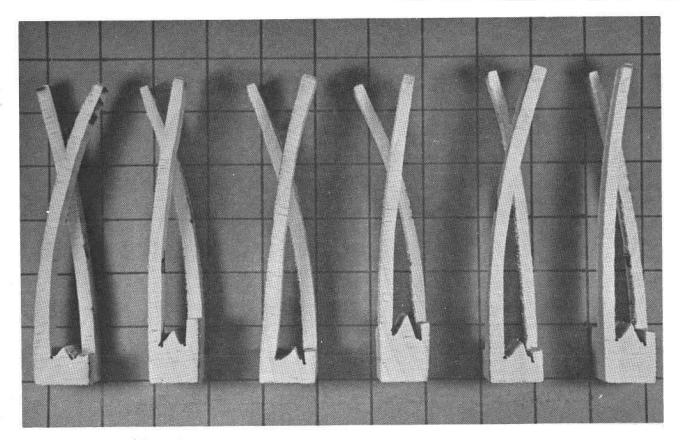
Figure 3.--Demonstration of internal stresses remaining in solar-
