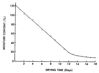
Figure 2.--Drying curve for solar-dehumidification drying of 4/4 yellowpoplar during December 1979 in southern Illinois.
