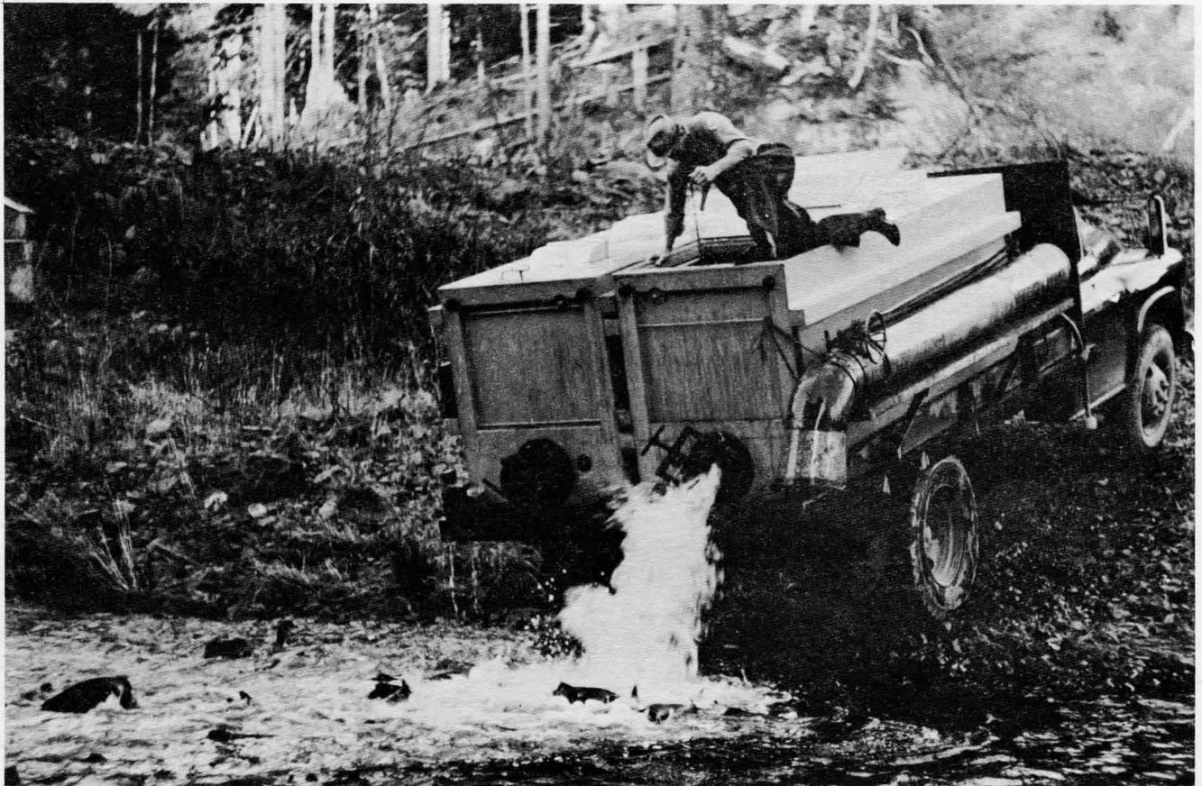
George Smalley won a suggestion award for developing a multiple use liberation tank which counts out smolts by the displacement method. In above picture, the tank is being used to transport and release adult coho.
