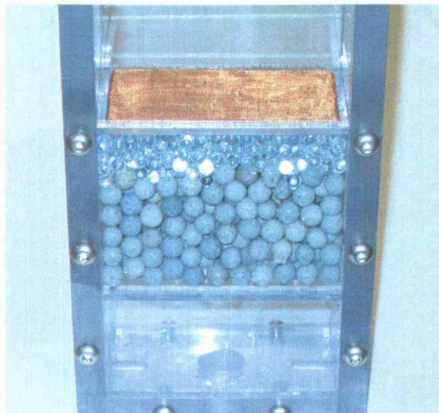
Figure 3.4 Close up of the calming zones and distributor plate.
