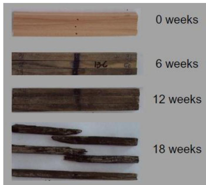
**Figure 4. Douglas-fir beams 0, 6, 12, and 18 weeks after inoculation with *P. placenta* at 35°C**
