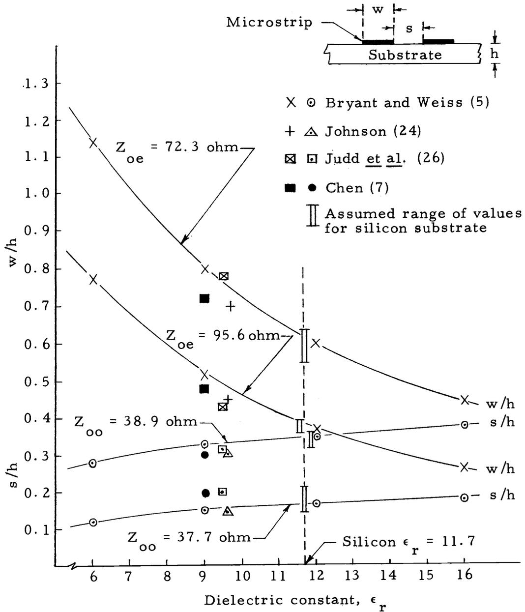
Figure 21. Width-to-height and spacing-to-height ratios for a coupled microstrip-lines with fixed even- and odd-mode impedances as a function of various dielectric constants for the substrate.
