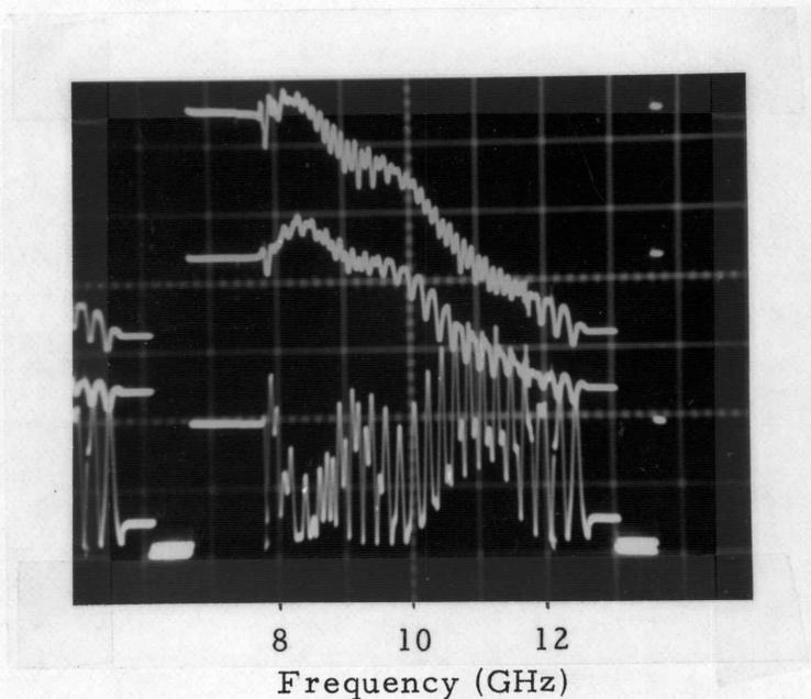
(a) Transmitted-powers, without 50-ohm microstrip (top), with 50-ohm microstrip (center), reflection at input terminal with 50-ohm microstrip (bottom).
