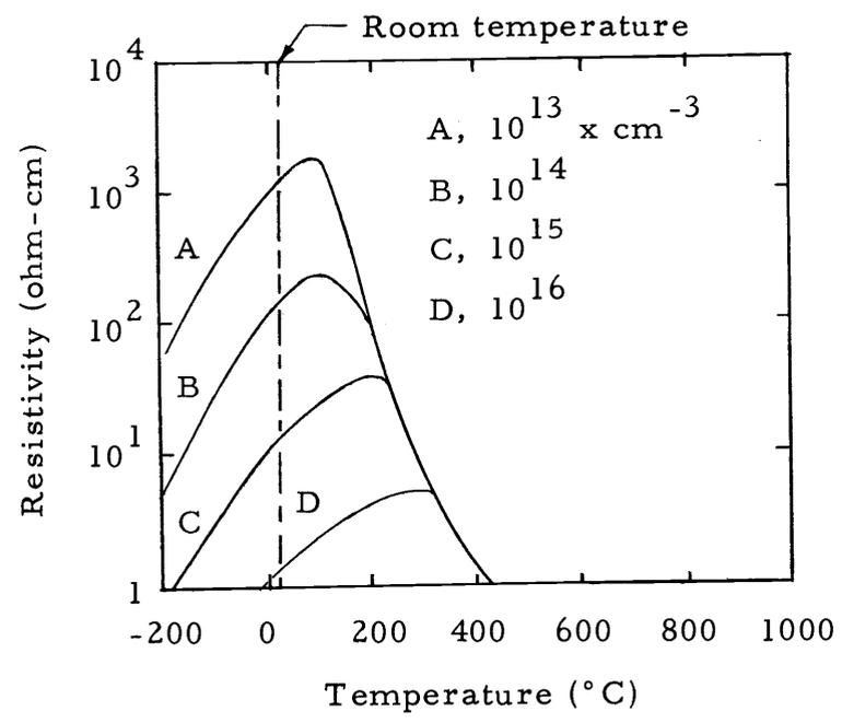
Figure 3. Resistivity versus temperature for boron-doped silicon (32, p. 168).
