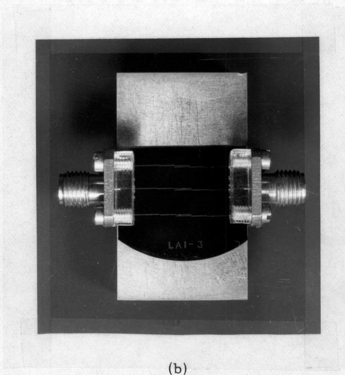
Figure 22. Parallel-coupled microstrip-lines band-pass filters. (a) Dimensions in detail. (b) Filters on the test fixture,  $f_0 = 10$  GHz (center),  $f_0 = 9$  GHz (top and bottom).
