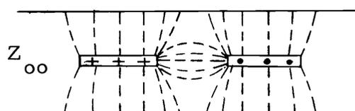
Figure 19. Shielded coupled-striplines. (a) Top-view. (b) Cross-sectional view of even-mode. (c) Cross-sectional view of odd-mode.
