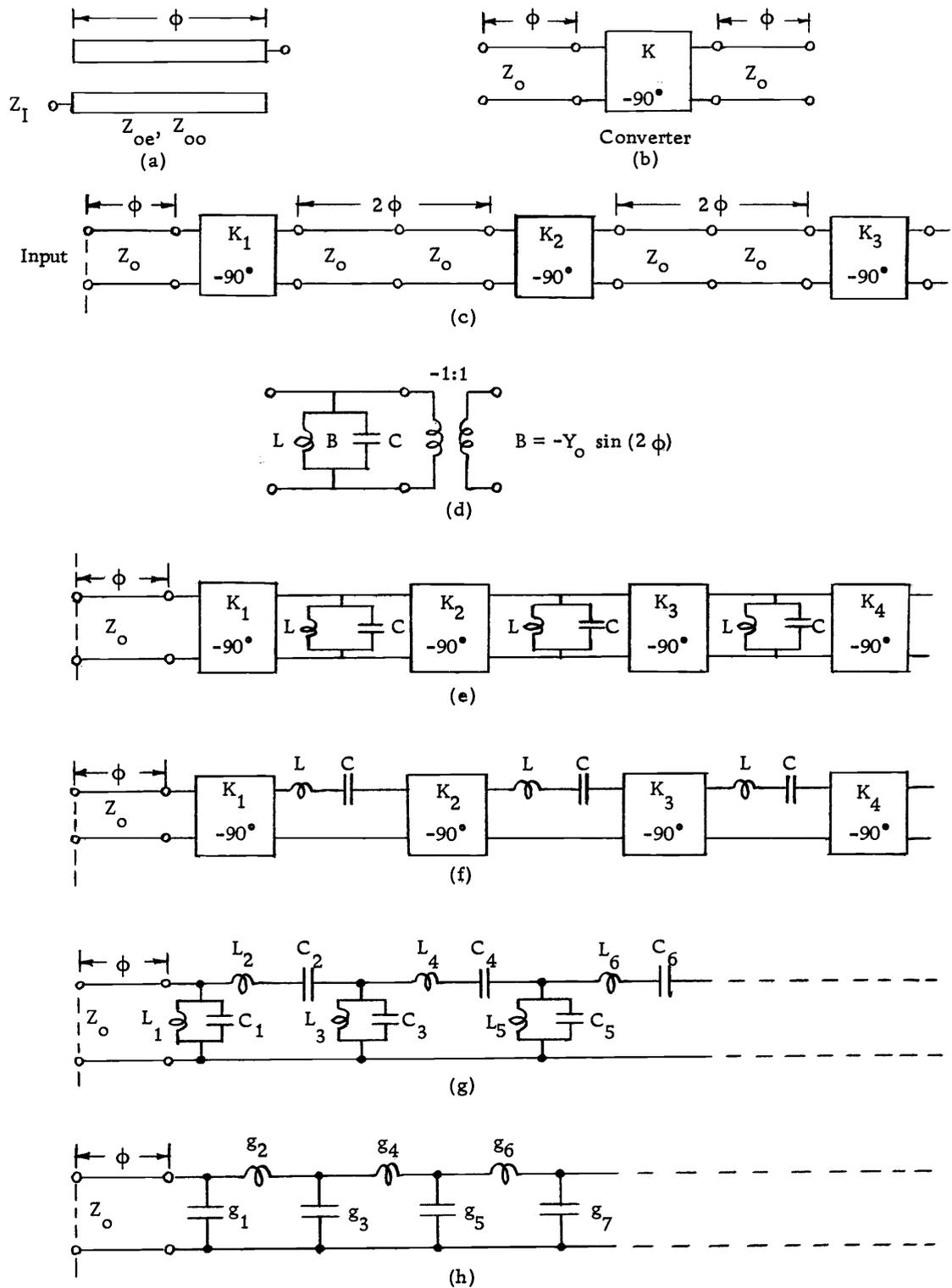
Figure 20. Development of equivalent circuit of the parallel coupled-stripline filter.
