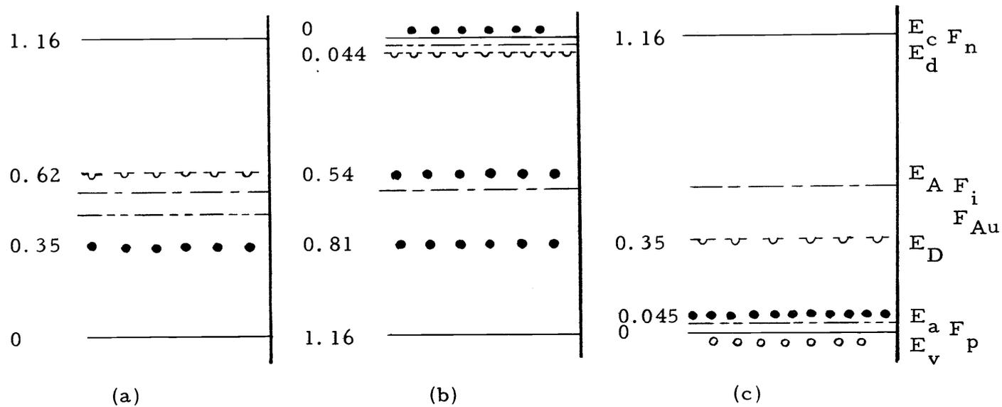
Figure 5. Energy band diagram for silicon doped with gold. (a) No other impurity present, (b) shallow donor present, (c) shallow acceptor present. In cases (b) and (c) it is assumed that the shallow impurity concentration is much greater than the gold concentration. Note that in case (c) the acceptor level does not exist since the donor levels are empty (6).
