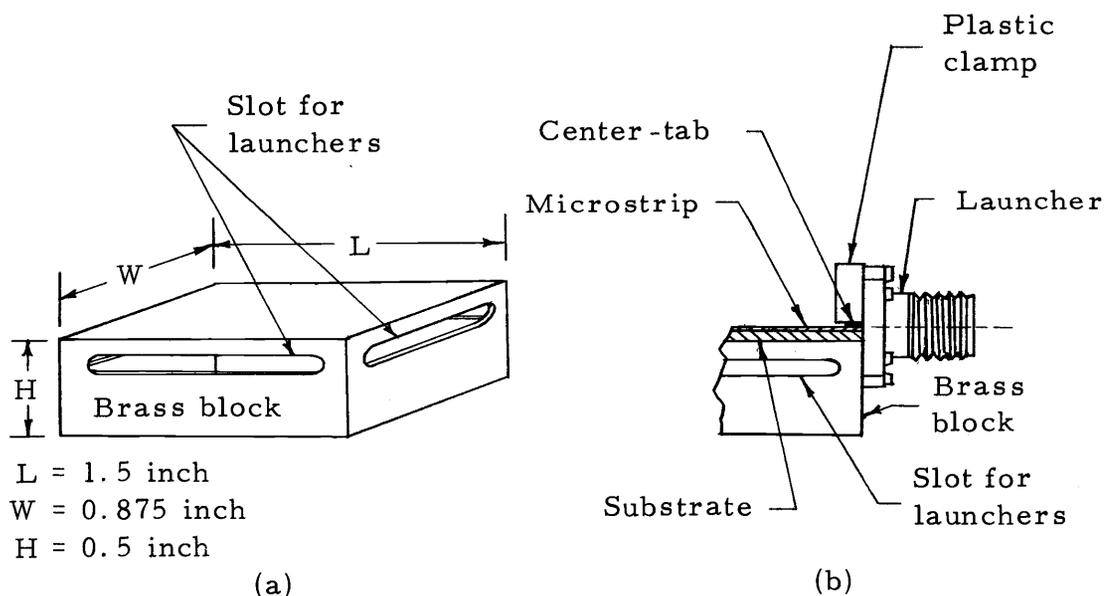
Figure 13. Test fixture for microstrips. (a) Main body of test frame. (b) Coaxial-to-microstrip transition.
