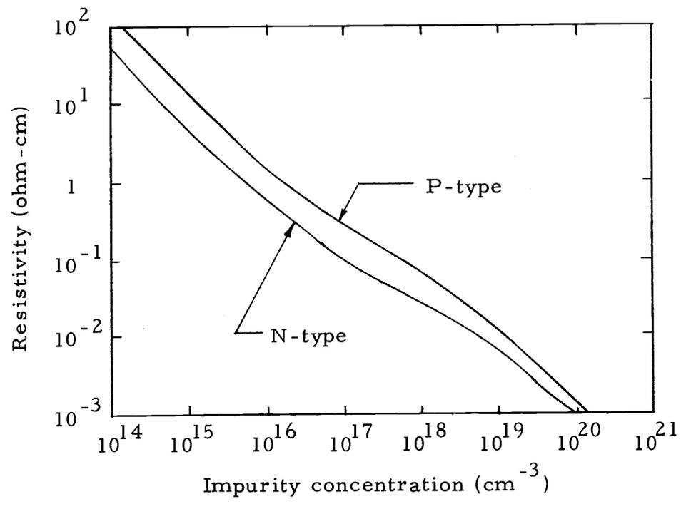
Figure 2. Resistivity of silicon at 27°C as a function of acceptor or donor concentration (24).
