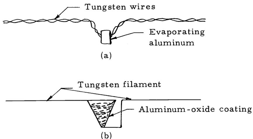
Figure 11. Filaments for evaporating metals. (a) For aluminum evaporation, (b) for gold evaporation.
