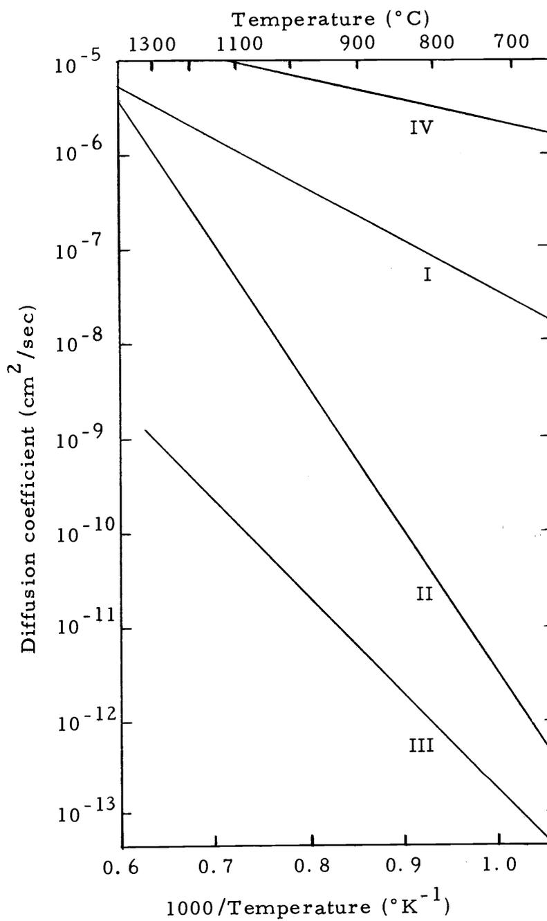
Figure 9. Diffusion coefficients calculated from experimental diffusion concentration profiles as a function of inverse temperature (Arrhenius plots). Curve I: interstitial controlled dissociative diffusion; Curve II: vacancy controlled dissociative diffusion; Curve III: substitutional diffusion; Curve IV: interstitial diffusion (40).
