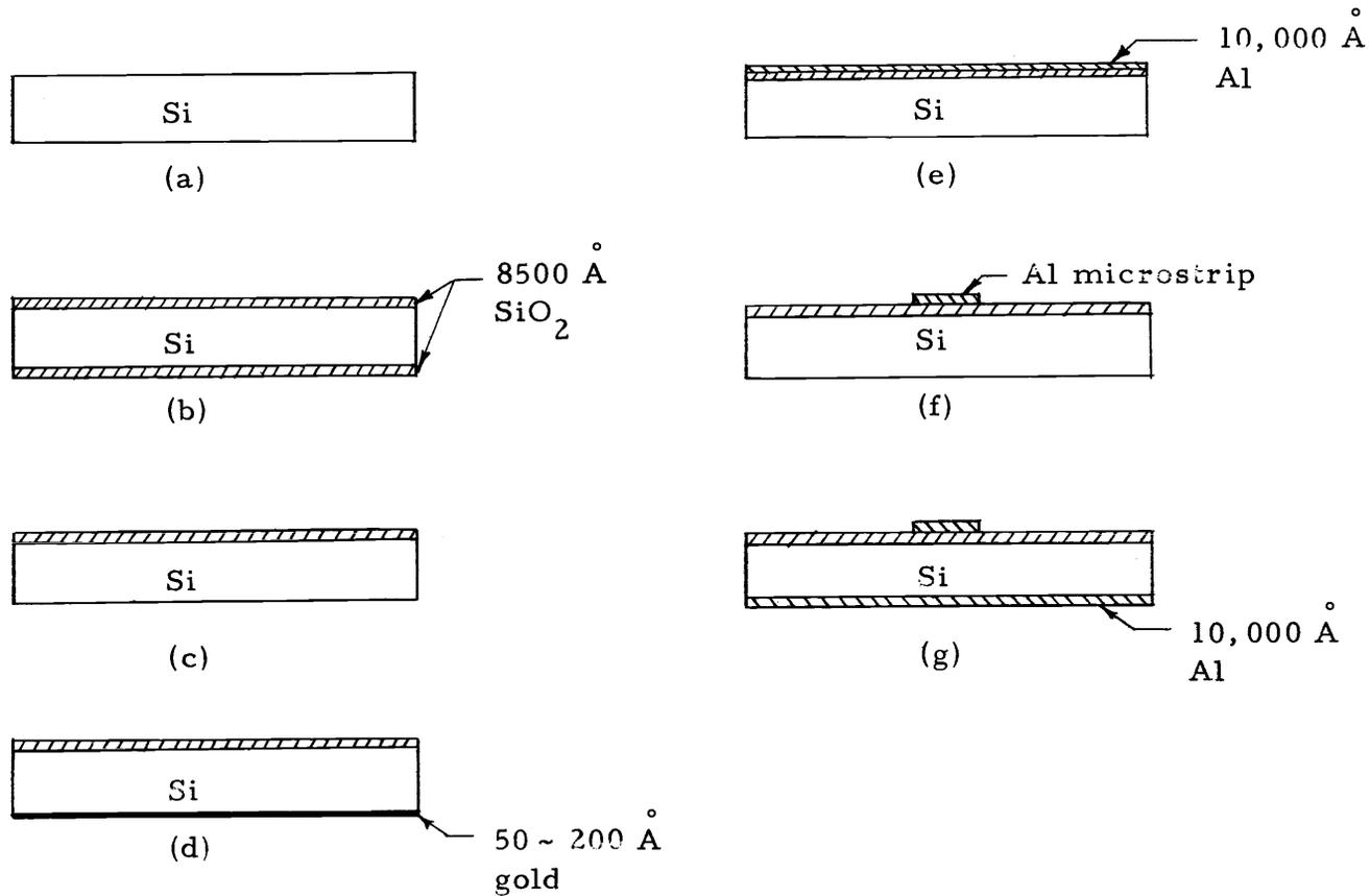
Figure 12. Schematic view of main process steps in microstrip fabrication on a gold-doped silicon substrate. (a) Wafer cleaning, (b)  $\text{SiO}_2$  growing, (c) back-side  $\text{SiO}_2$  etching, (d) gold deposition and diffusion, (e) aluminum deposition, (f) microstrip masking and etching, (g) aluminum ground-plane deposition.
