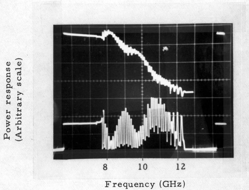
Figure 18. Responses of a system with only a straight coaxial-to-coaxial adapter. Transmitted-power (upper trace) and reflected-power (lower trace).
