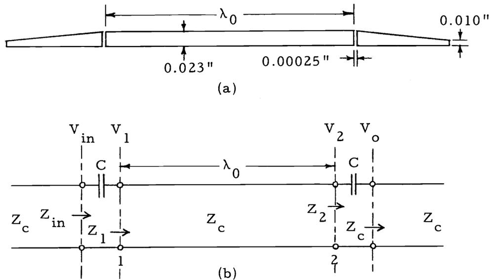
Figure 14. Microstrip for  $Q$ -measurement test. (a) Physical lay-out,  $\lambda_0 = 0.422$  inch for 10 GHz and  $\lambda_0 = 0.437$  inch for 9 GHz. (b) The equivalent circuit,  $Z_c = 25$  ohm.
