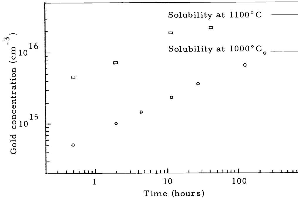
Figure 10. Gold concentration in the uniform concentration region versus time for diffusion into relatively thin, low dislocation, high resistivity p-type slices. Data are from Sprokel and Fairfield (36).
