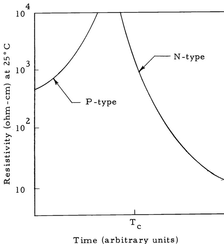
Figure 4. Behavior of high-resistivity silicon during high temperature processing.  $T_c$  is approximately six hours at 1100°C in O<sub>2</sub> ambient (3).
