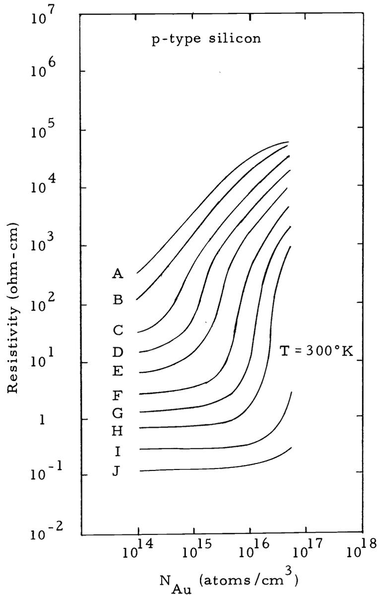
Figure 7. Resistivity versus gold concentration in boron-doped silicon at  $T = 300^\circ\text{K}$ . Primary boron concentrations ( $\text{cm}^{-3}$ ) assumed are: A,  $1 \times 10^{14}$ ; B,  $2 \times 10^{14}$ ; C,  $5 \times 10^{14}$ ; D,  $1 \times 10^{15}$ ; E,  $2 \times 10^{15}$ ; F,  $5 \times 10^{15}$ ; G,  $1 \times 10^{16}$ ; H,  $2 \times 10^{16}$ ; I,  $5 \times 10^{16}$ ; J,  $1 \times 10^{17}$  (32, p. 172).
