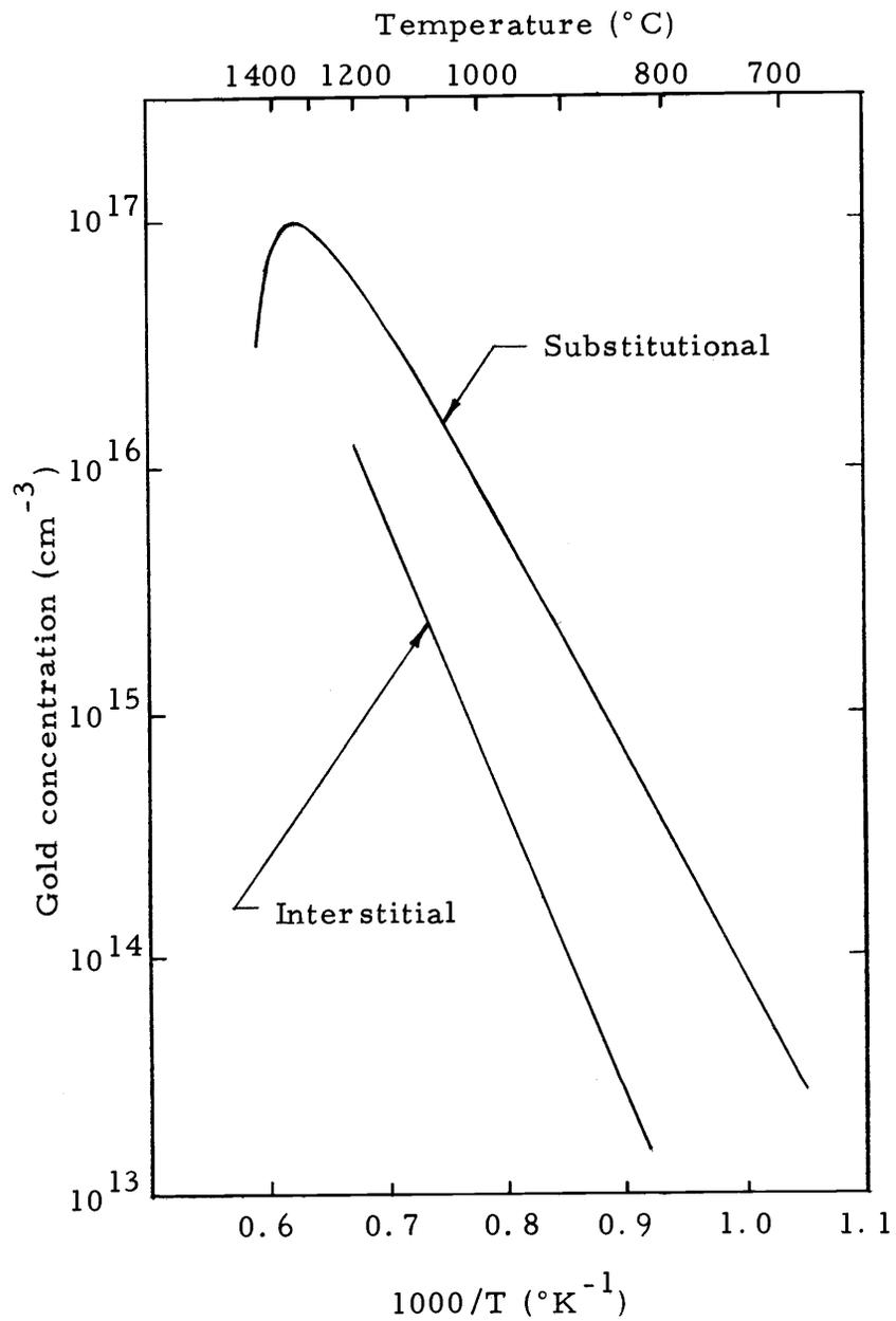
Figure 8. Solubility of gold in silicon. The substitutional curve is calculated by Wackwitz (6). The interstitial curve is calculated by Wilcox and LaChapelle (40).
