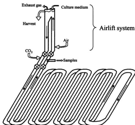
Figure 2.7.2 a: Tubular photobioreactor system (Molina et al., 2001).
