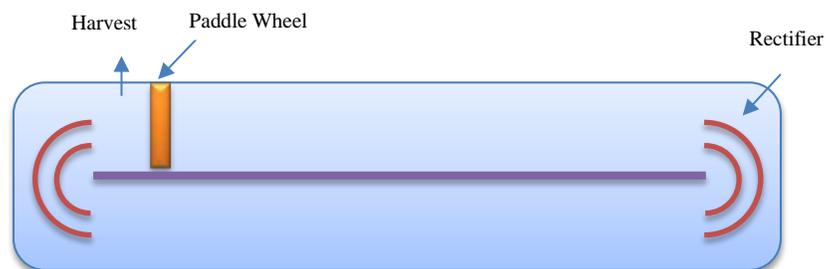
**Figure 2.7.1 a: Schematic open pond system for algae culture.**
