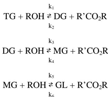
Several parameters can determine the reaction rate of transesterification, including impeller speed, temperature, and catalyst concentration. Two different methods are used to evaluate the kinetics of transesterification reaction, regarding catalyst concentration or not regarding catalyst concentration.
