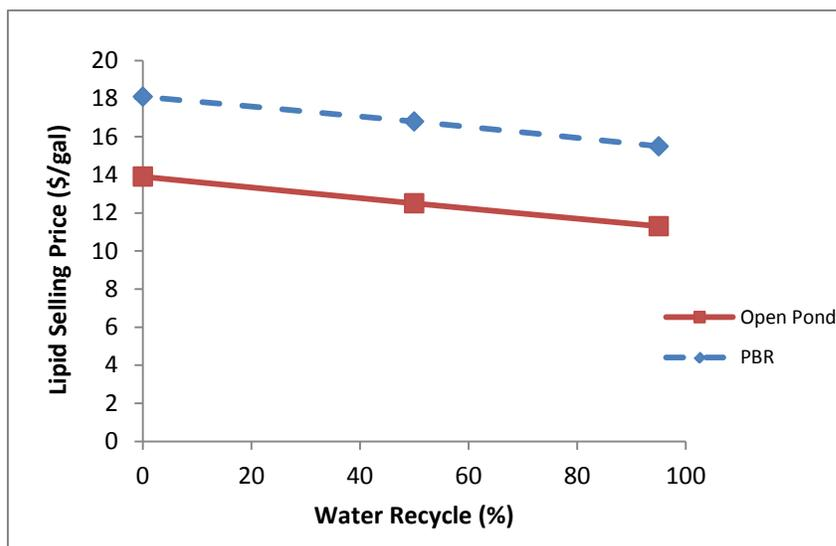
Figure 3.10.4 c: Algal lipid selling price as a function of medium recycle rate.
