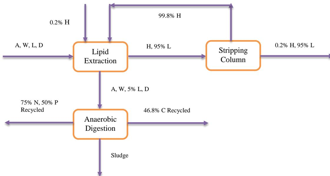
**Figure 3.7.3 a: Flowsheet of main components in extraction and anaerobic digestion process**
