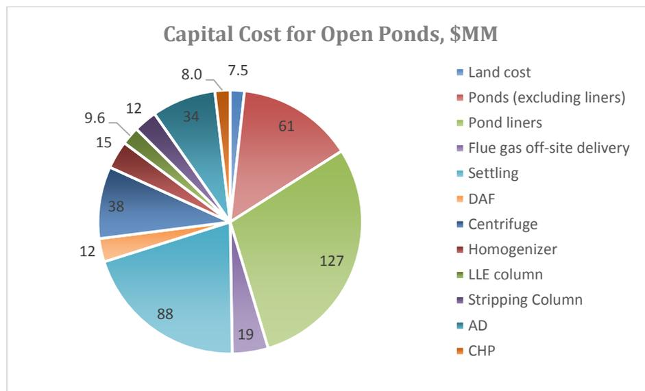
**Figure 3.10.1.3 a: Capital cost of an open pond algal lipid facility for 10 MGY lipid productions.**
