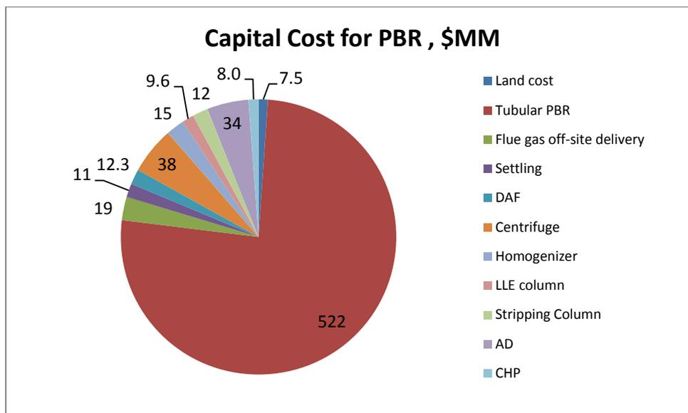
**Figure 3.10.1.3 b: Capital cost of a PBR algal lipid facility for 10 MGY lipid productions.**
