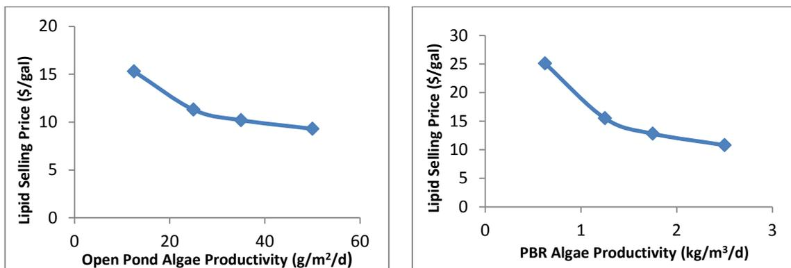
Figure 3.10.4 a: Algal lipid selling price as a function of algae productivity. The left plot is open pond system and the right plot is PBR system.
