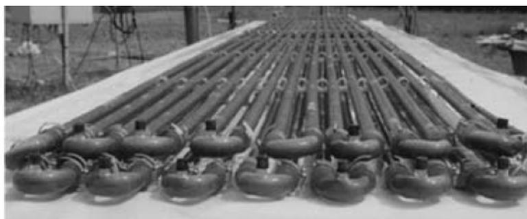
**Figure 3.3 a: two-plane reactor at the Centro di Studio dei Microrganismi Autotrofi of the CNR (Florence, Italy) (Tredici, 2004)**
