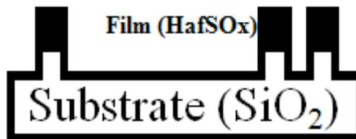
**Step 4: Substrate is etched with plasma, creating a pattern in the substrate.**
