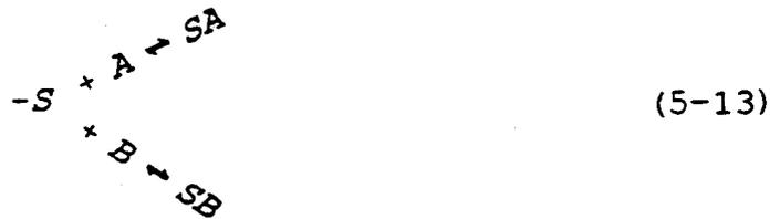
in which  $-S$  represents the unoccupied surface sites, and  $SA$  and  $SB$  represent the surface sites occupied by components  $A$  and  $B$ , respectively.
