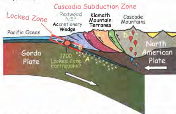
Figure 4-2: Did you feel that? There are four basic types and locations of earthquakes related to Gorda Plate subduction (x's on diagram). A) Earthquakes within the Gorda Plate. The upper portion of the Gorda Plate stays relatively cool (brittle) for some time as it subducts farther and deeper beneath North America. When it breaks, it can generate earthquakes to depths of about 30 miles (50 km) beneath the Coast Range and Klamath Mountains. These are commonly referred to as "subduction slab" earthquakes, such as the magnitude 6.8 Nisqually earthquake that occurred beneath the Seattle, Washington, area on February 28, 2001 [Preston, 2003]. B) "Mega thrust," or "locked zone," earthquakes. The earthquakes occur between the subducting Gorda Plate and the overriding North American Plate. The plates slip and suddenly grind past each other after being locked together for hundreds of years. The energy released generates extremely high magnitude earthquakes (fig 4-6), which can generate tsunamis (fig 5-2). This type of earthquake happened on March 27, 1964 off the coast of Alaska, registering a moment magnitude 9.2, and generating a tsunami that hit Crescent City, California, less than 5 hours later. C) Those within the North American Plate. As the edge of the continent is crumpled (like a rug) by the Gorda plate, inland areas experience compression and reverse faulting at shallow depths. These small-to-moderate size earthquakes are common in the Seattle and Portland areas. D) Shallow rumbles from rising magma beneath the Cascade volcanoes. The magma "jostles" rock out of its way, generating small earthquakes. Such earthquakes can at times be used to track the rise of magma prior to volcanic eruptions.
