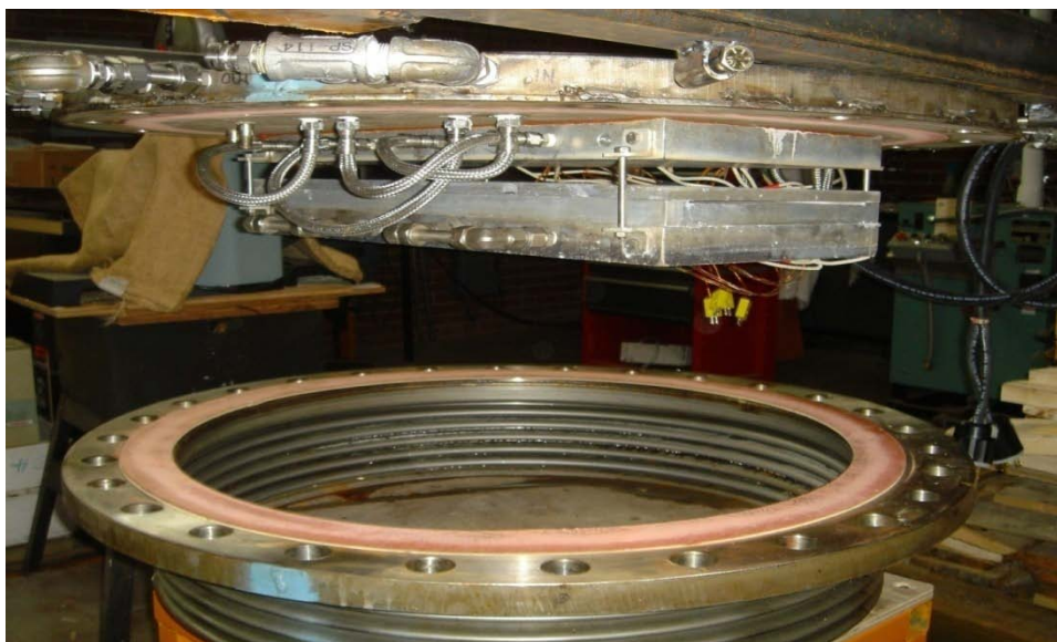
Figure 4.1.5 VTC device shown with the lid opened. Independently-heated platens are attached to the inside of the lid.
