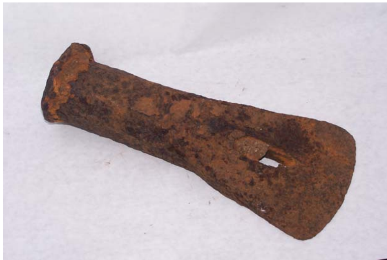
Figure 8.10: Splitting maul used with dynamite
