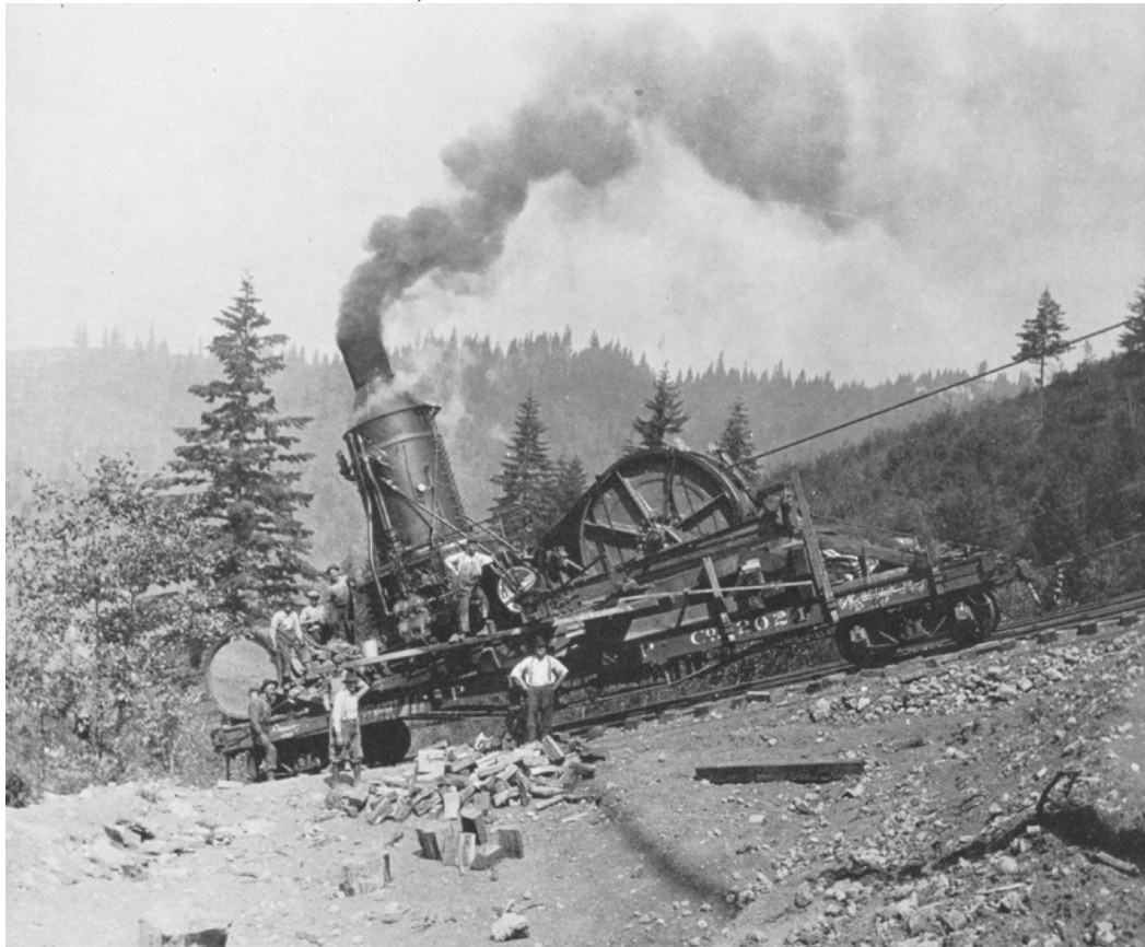
Figure 6.8: Lowering donkey on the steep pull up the incline to Camp 1 (Willamette Iron and Steel Works 1925:70).
