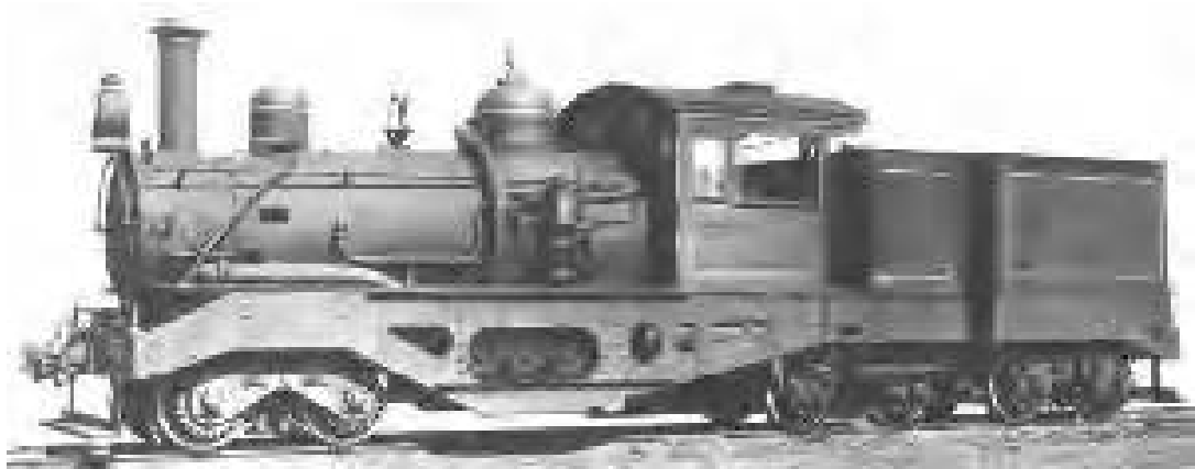
Figure 5.9: Example of “Shay-type” oil-burning rod-driven engine manufactured by Baldwin (Bryant 1923:188)
