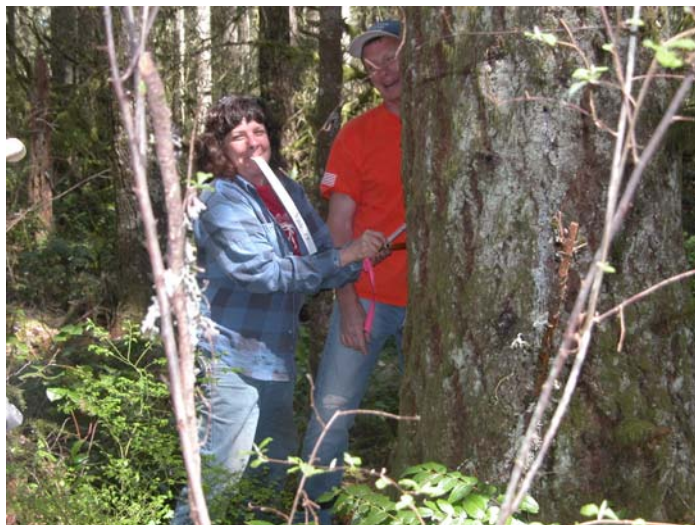
Figure 7.2: The author extracting a tree core from the increment borer.
