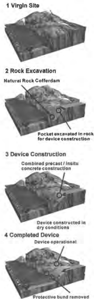
Fig. 3 Construction Sequence of the Limpet
