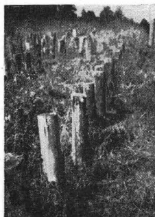
Round, Douglas-fir posts treated by the salt method in 1928. None had failed in 1947 although tops showed rot. Similar untreated posts lasted 7 years.
