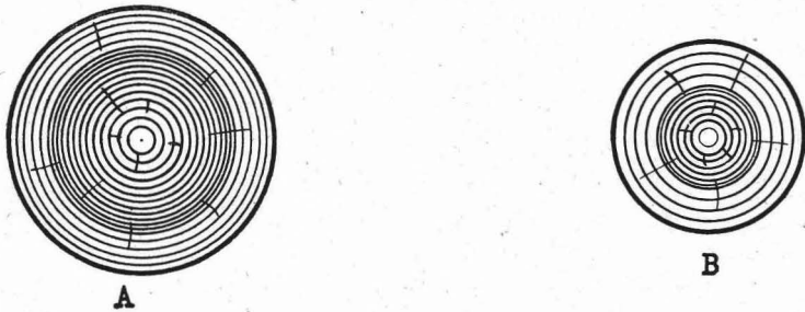
Figure 2. Post A has a greater percentage of heartwood than B, therefore is more desirable as a fence post.
