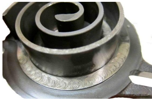
Fig. 39: Extensive wear to orbiting scroll caused by insufficient lubrication.
