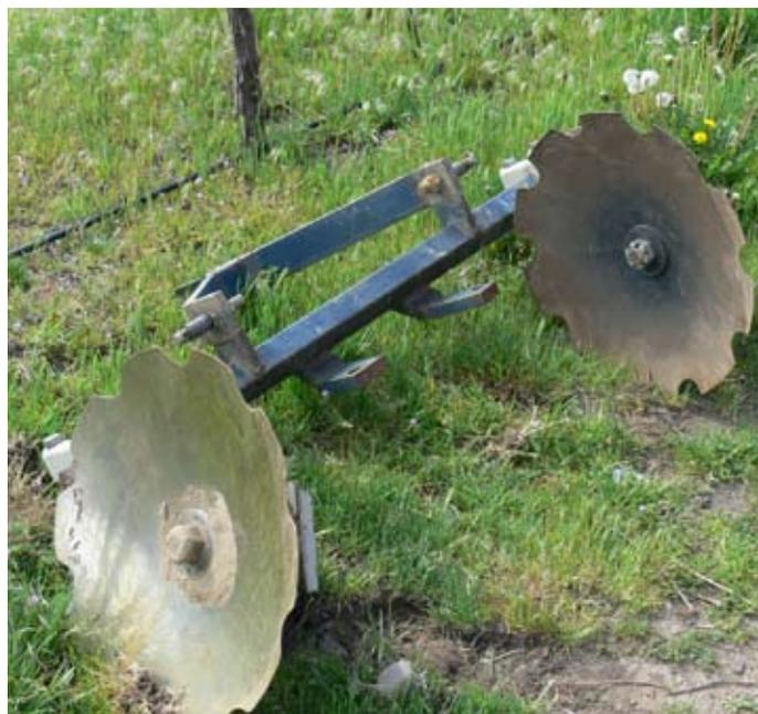
**Figure 9. Plough with angled blades for cutting a 4-inch V-trench.**
