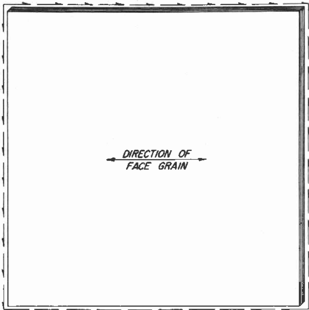
Figure 1.—Plywood panel subjected to uniformly distributed edgewise shear stresses.
