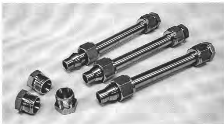
FIGURE 1.5. Stainless steel tubes used for sample heating
