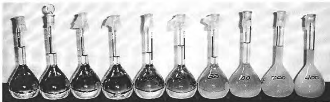
FIGURE A-1. Increasing alpha-acid concentrations, pH 5.2
