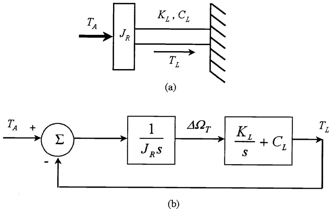
**Figure 1.4** Simplified wind turbine (a) mechanical model and (b) block diagram, typically utilized for determination of mechanical system resonances and responses
