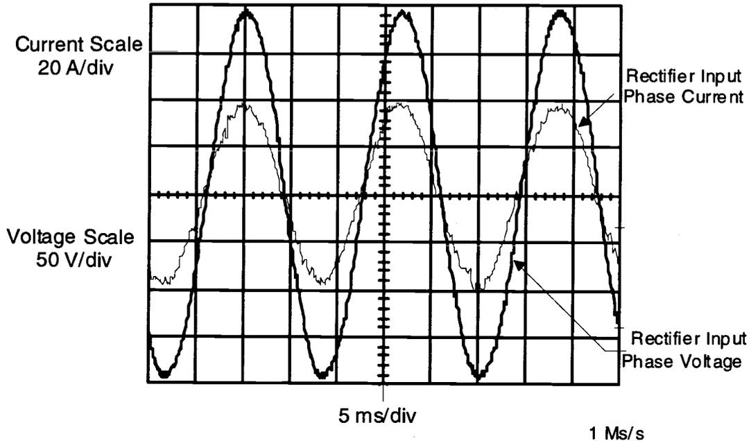
**Figure 3.7** Unity power factor operation of the sensor-based rectifier controller.
