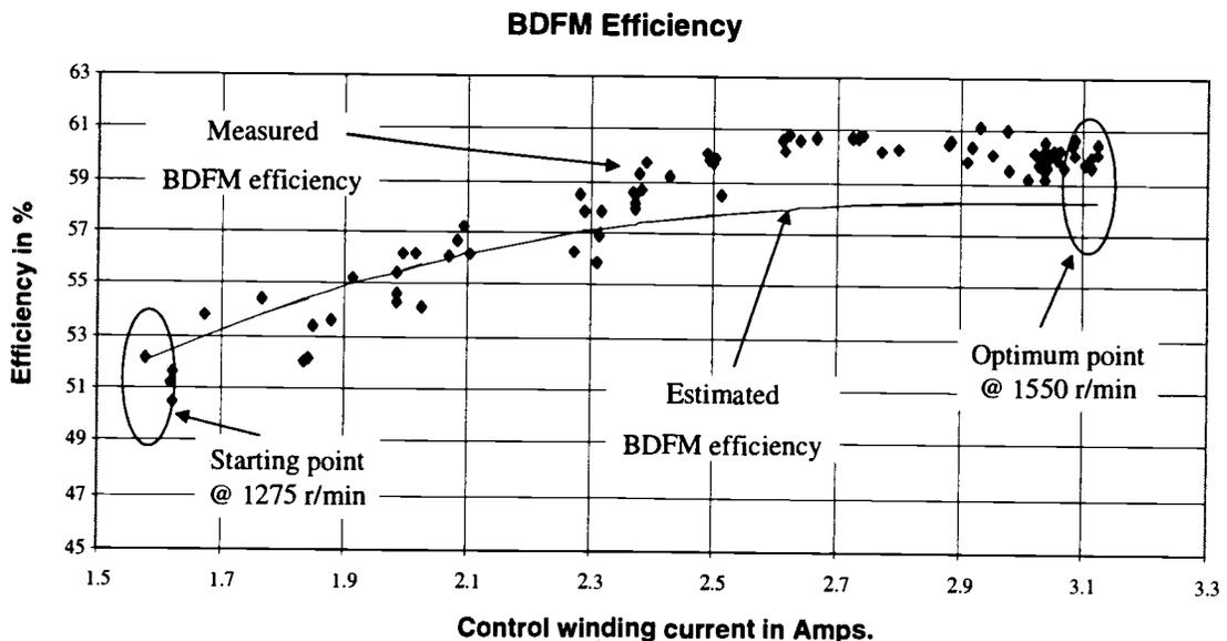
**Figure 5.2** Maximum efficiency point tracking by the performance optimization controller.
