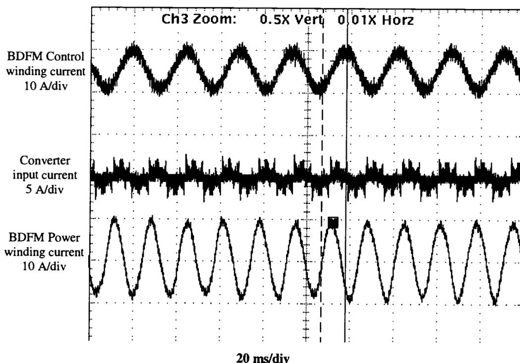
**Figure 5.6** Representative current waveforms of the converter and the BDFM approximately at the maximum power point ( $P_{wt} \approx 1150$  watts, shaft speed = 1525 r/min).
