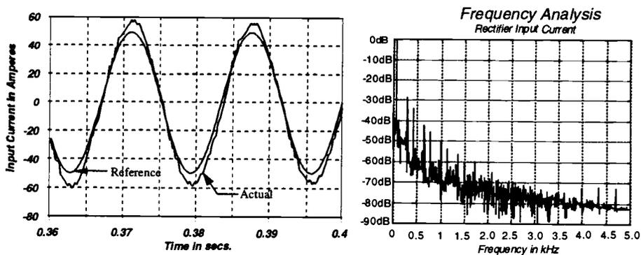
**Figure 3.14** Time and frequency domain simulation result of rectifier input current with the proposed model based current controller under unity p.f. condition.
