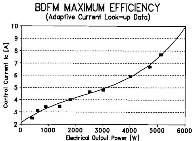
**Figure 2.5** Optimal control winding current requirements to ensure maximum efficiency for a 7.5kW BDFM.
