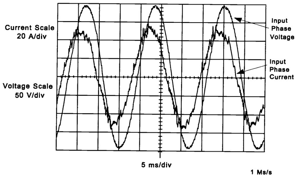
**Figure 3.8** Leading 0.85 p.f. operation.  $V_{dc} = 390$  V
