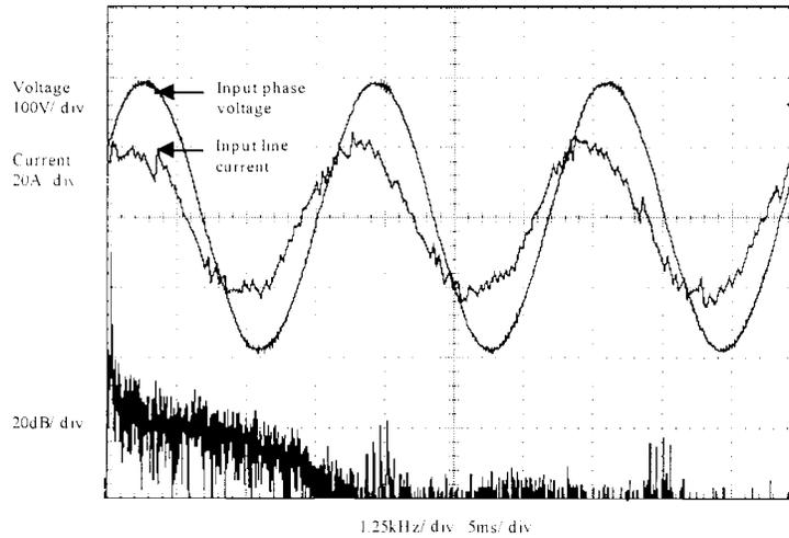
**Figure 3.17** Leading power factor operation of the sensorless controller.
