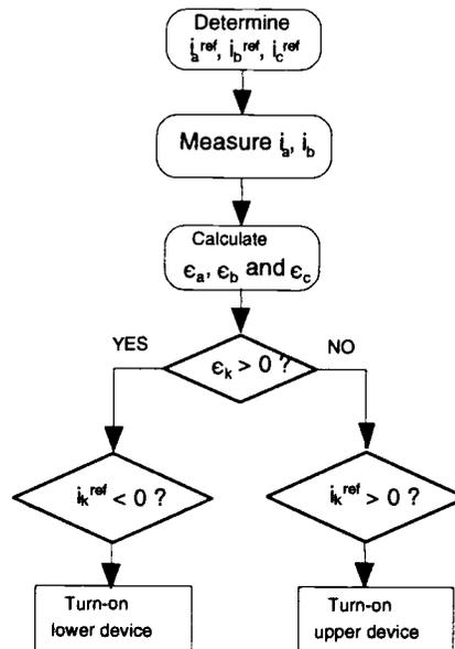
Figure 3.4 Switching logic of the rectifier.
