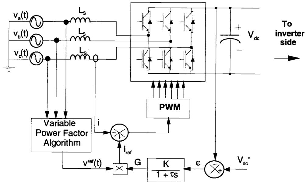
**Figure 3.2** Sensor-based controller representation.
