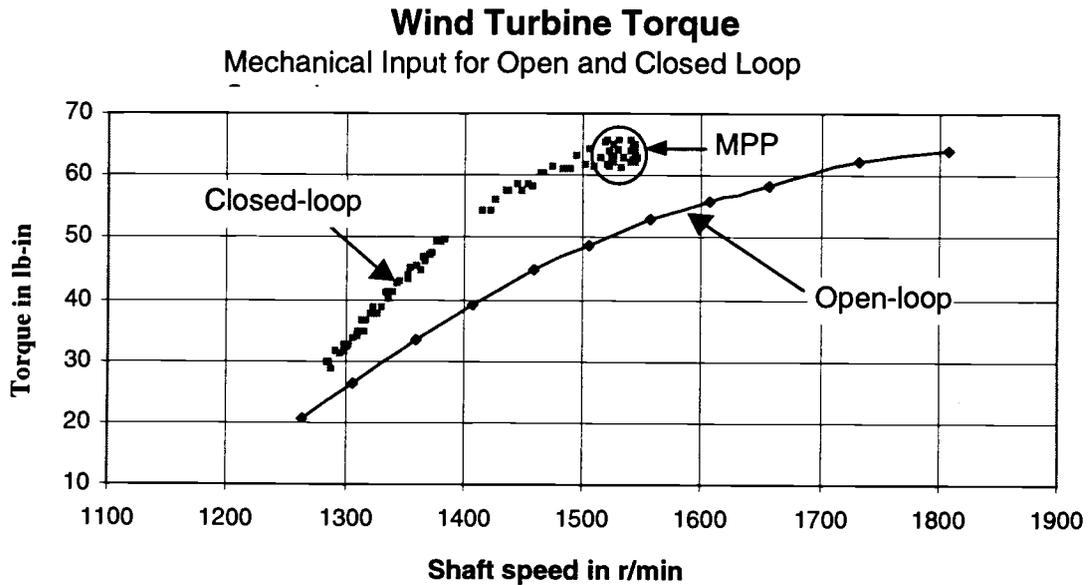
**Figure 4.6** Measured turbine model torque. Closed-loop operation illustrates the effectiveness of the optimization controller and turbine convergence at the set MPP.
