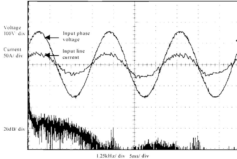
**Figure 3.18** Rectifier operation with an (-)20% grid voltage error.
