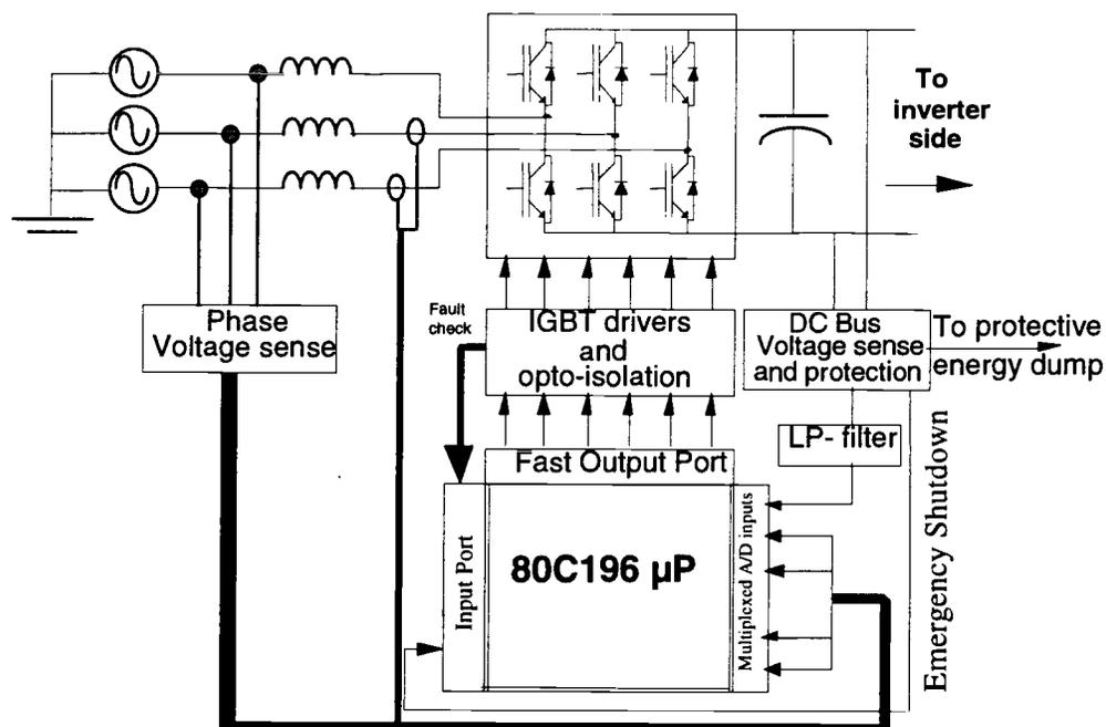
**Figure 3.5** Sensor-based rectifier controller implementation
