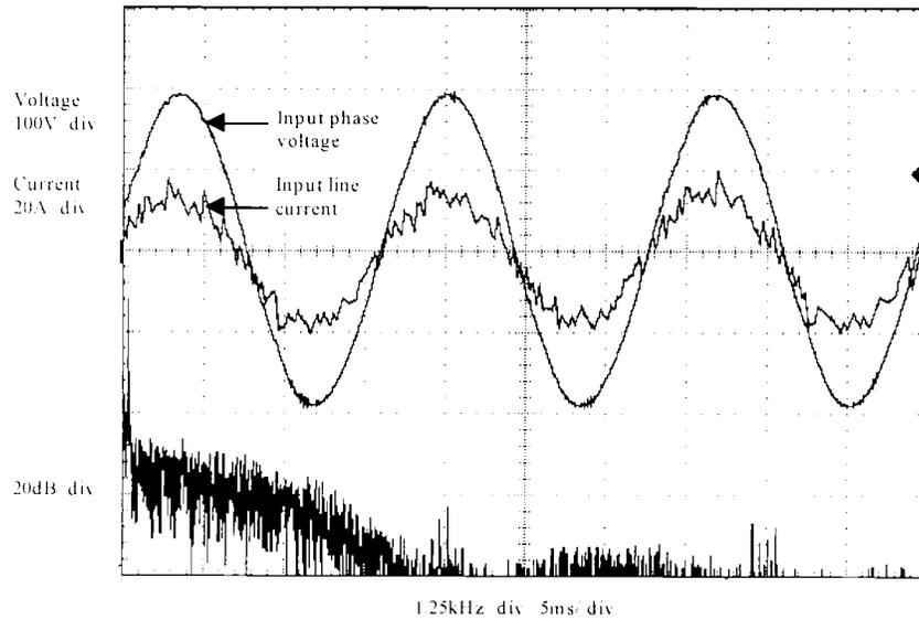
**Figure 3.20** Rectifier operation with (-)21% line reactor inductance error.
