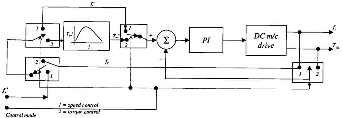
**Figure 4.2** DC machine based wind-turbine model controller.
