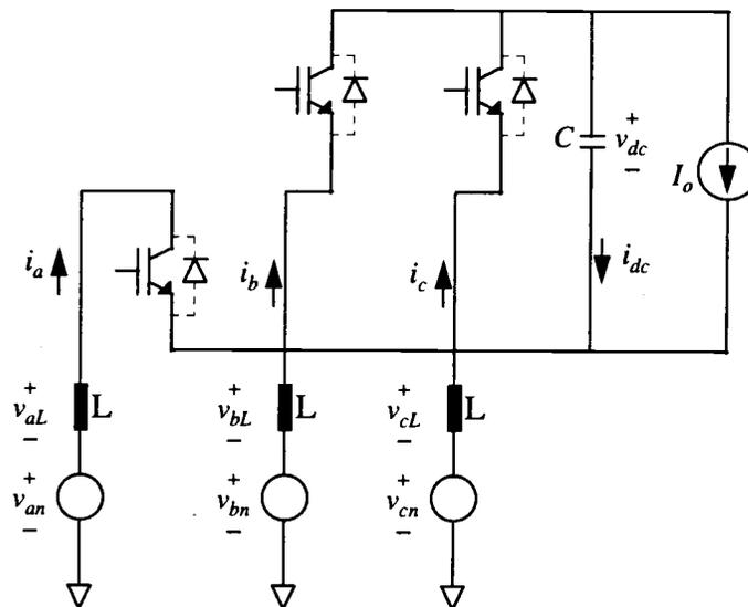
**Figure 3.12** Lumped circuit representation of a switching state of the rectifier
