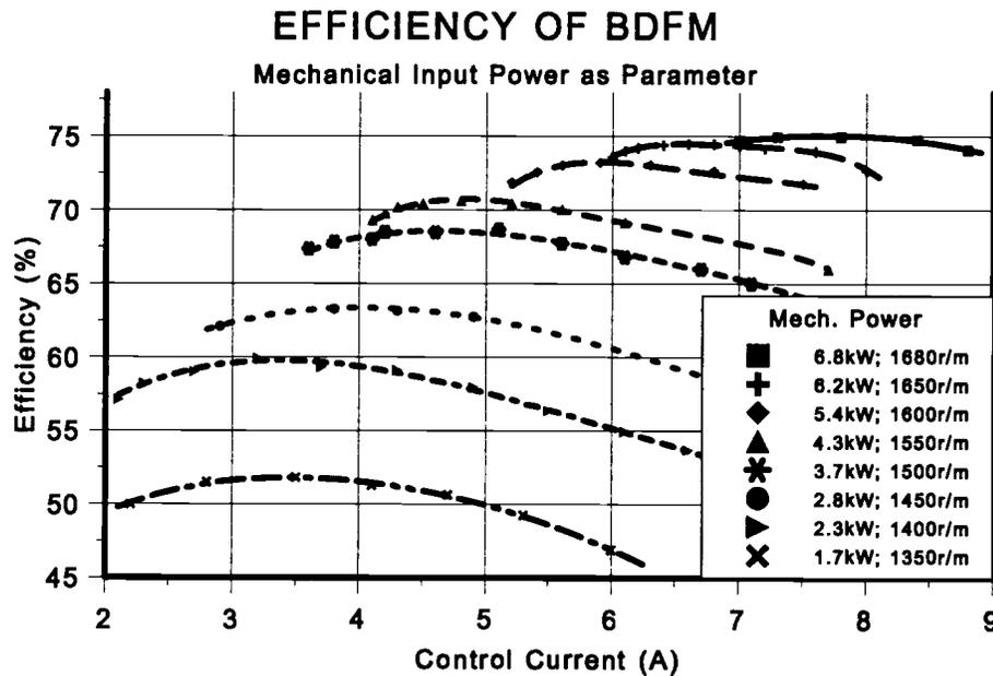
**Figure 2.6** Maximum efficiency point characterization of a 230 V, 7.5 kW prototype BDFM with input mechanical power as a parameter.
