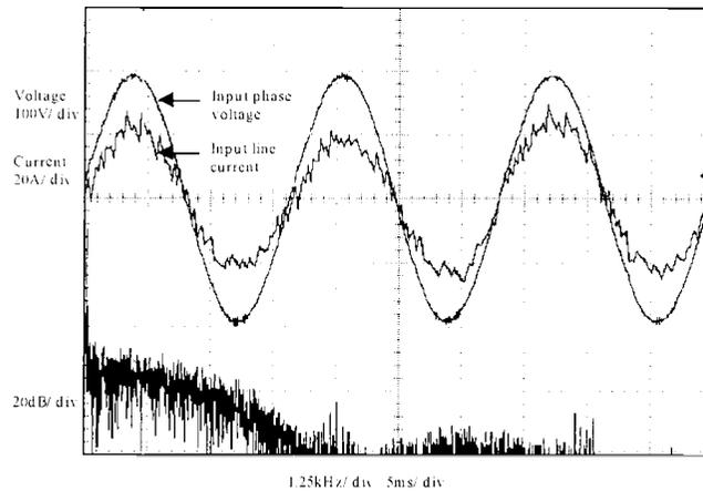
**Figure 3.16** Unity power factor operation of the sensorless controller.
