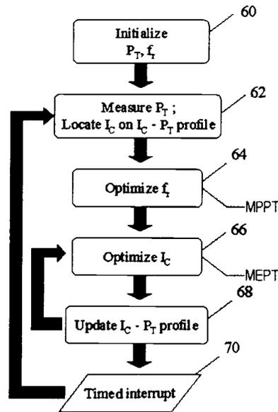
**Figure 2.3** Generalized flowchart representation of the proposed optimization algorithm
