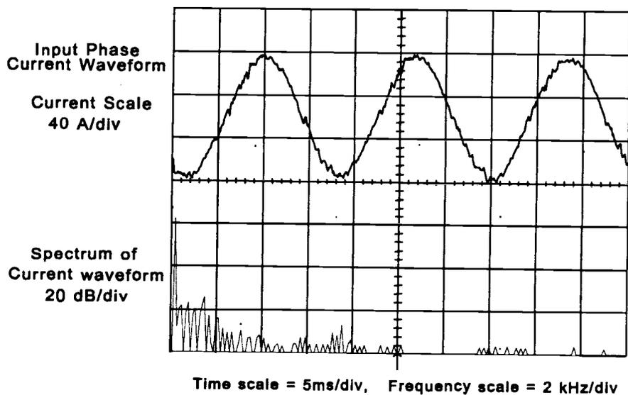
**Figure 3.9** Leading 0.85 p.f. operation.  $V_{dc} = 450$  V,  $V_{ac} = 230$  V, load = 10 kW.
