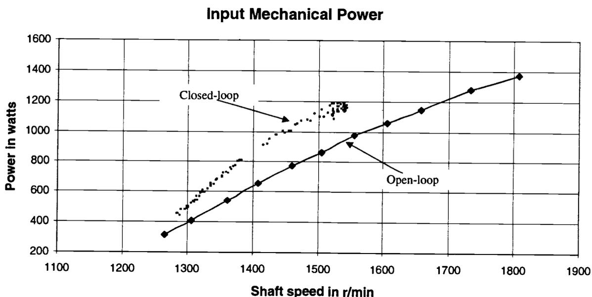
**Figure 5.3** Turbine output power for open and closed loop operation.
