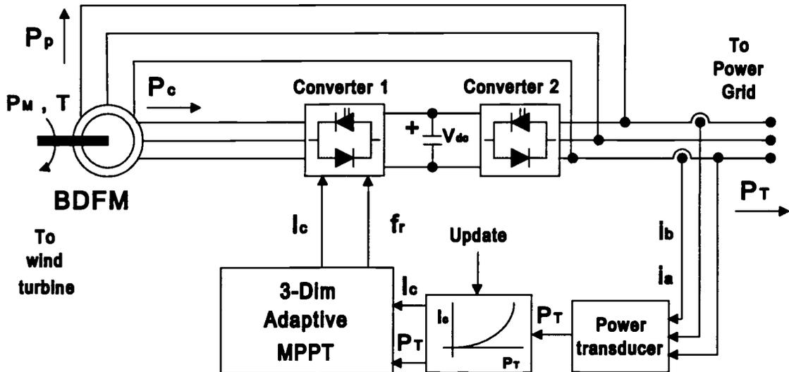
**Figure 2.2** Block diagram representation of the controller in a wind generation application.
