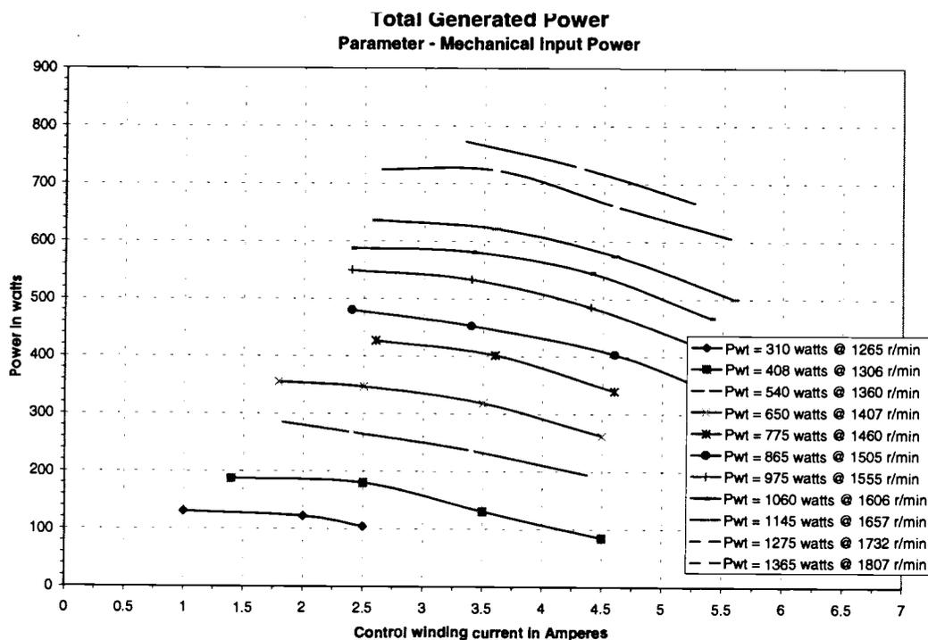
**Figure 4.7** Variation of generated power with varying of control winding current for different input mechanical power.
