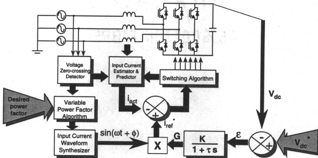
Figure 3.11 Sensorless version of the rectifier controller.
