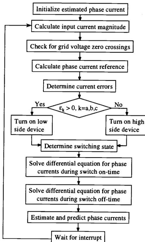
**Figure 3.13** Simplified flowchart of the sensorless version of the rectifier controller
