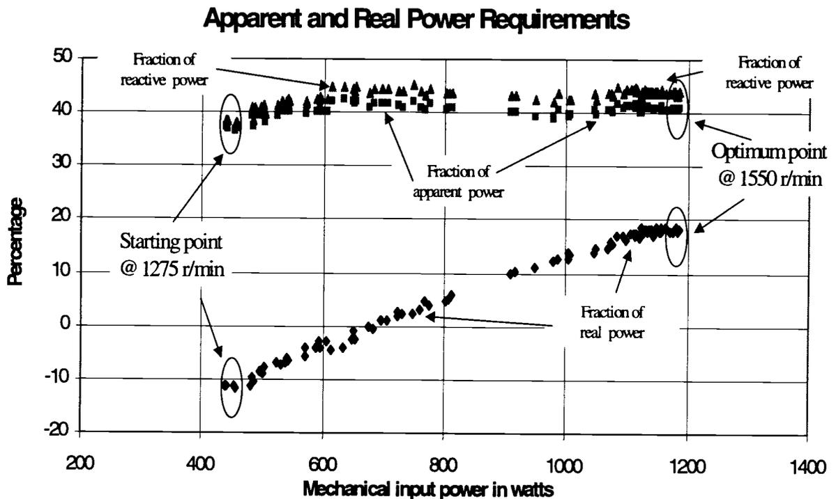
**Figure 5.5** Power flow through the inverter as percentage of total apparent, real and reactive power.
