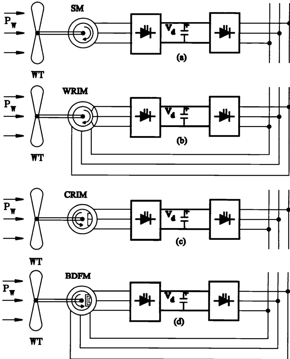
**Figure 1.3** Energy conversion systems for variable speed generation: (a) synchronous, (b) wound rotor induction, (c) cage rotor induction and (d) brushless doubly-fed.
