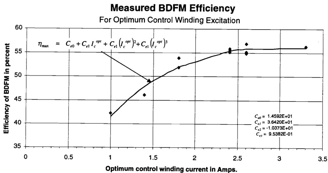
**Figure 4.9**  $\eta_{max} - I_c^{opt}$  profile of the prototype BDFM as implemented in the adaptive MPPT controller
