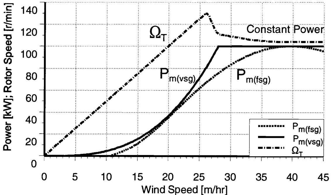
Figure 1.2 Variable and fixed speed power and speed characteristics of a 100 kW turbine.
