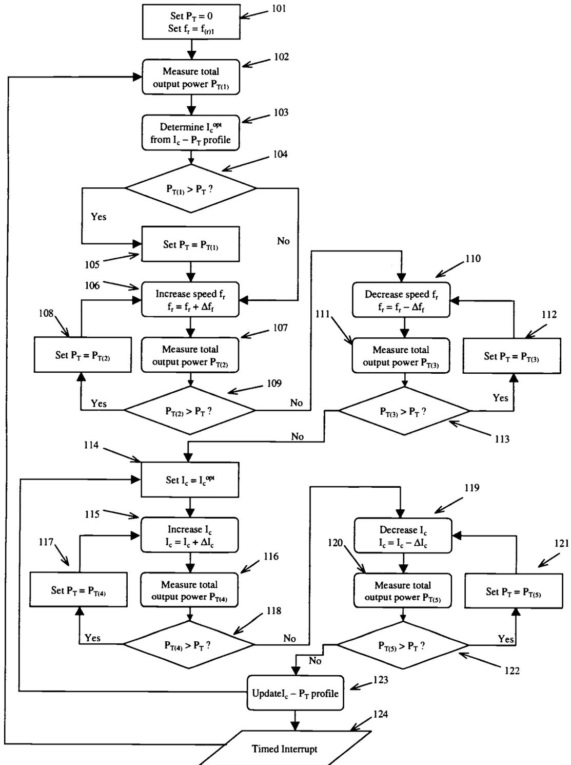
Figure 2.4 Perturbation based search algorithm for maximum power point tracking.
