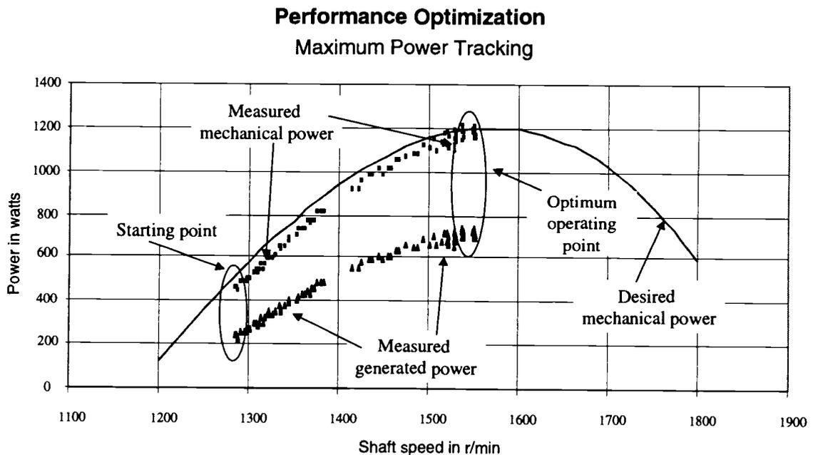
**Figure 5.1** Closed loop operation of the performance optimization controller.
