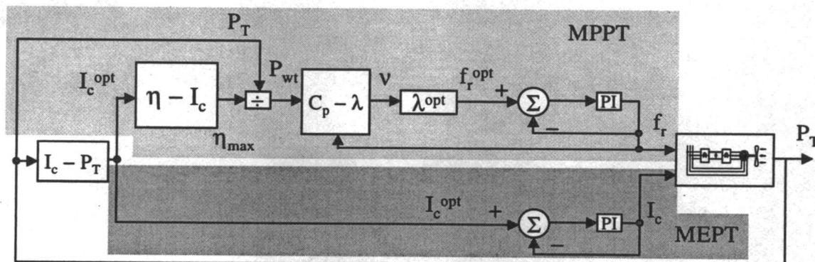
**Figure 4.11** Block diagram of the performance optimization system controller as implemented in the laboratory VSG system.
