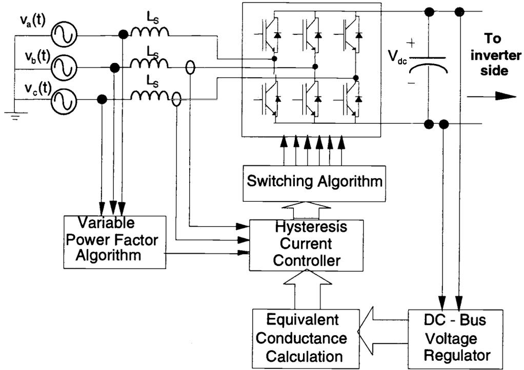
**Figure 3.1** Block diagram representation of the sensor-based rectifier controller.
