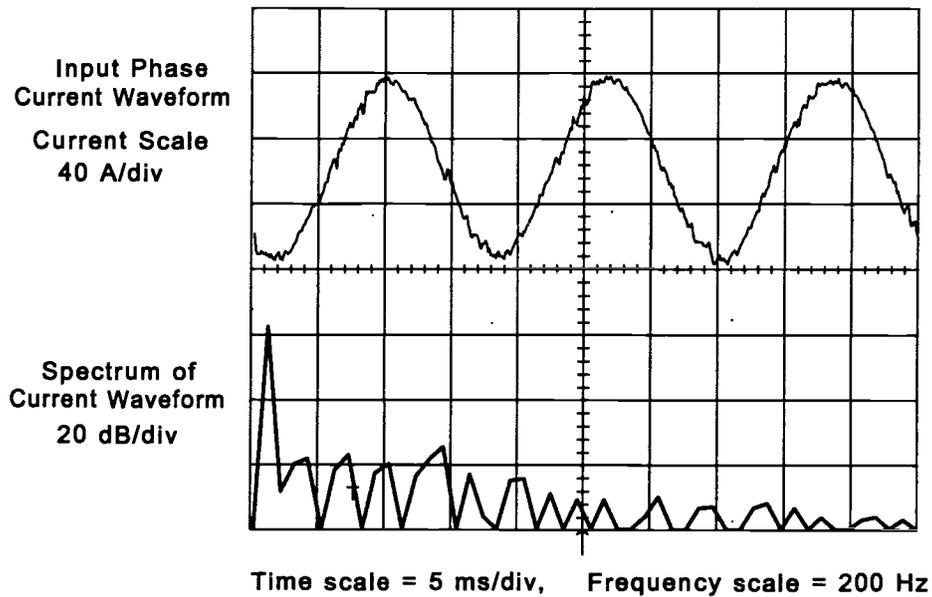
**Figure 3.10** Expanded view of the Fourier spectrum as shown in Fig. 3.9.
