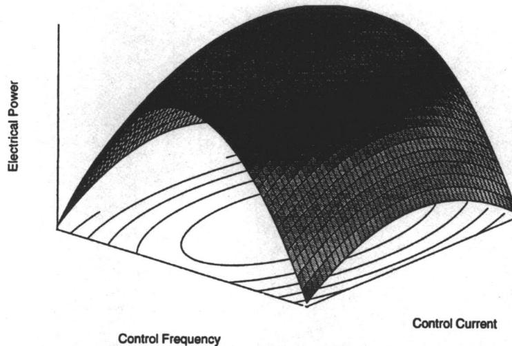
**Figure 2.1** Conceptual representation of the VSG optimization controller as a three-dimensional problem.
