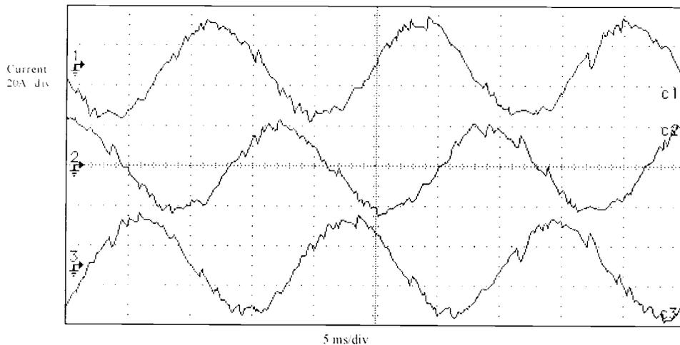
**Figure 3.21** Three phase current waveforms for 0.85 leading p.f. operations. Conditions similar to that of Fig. 3.17.
