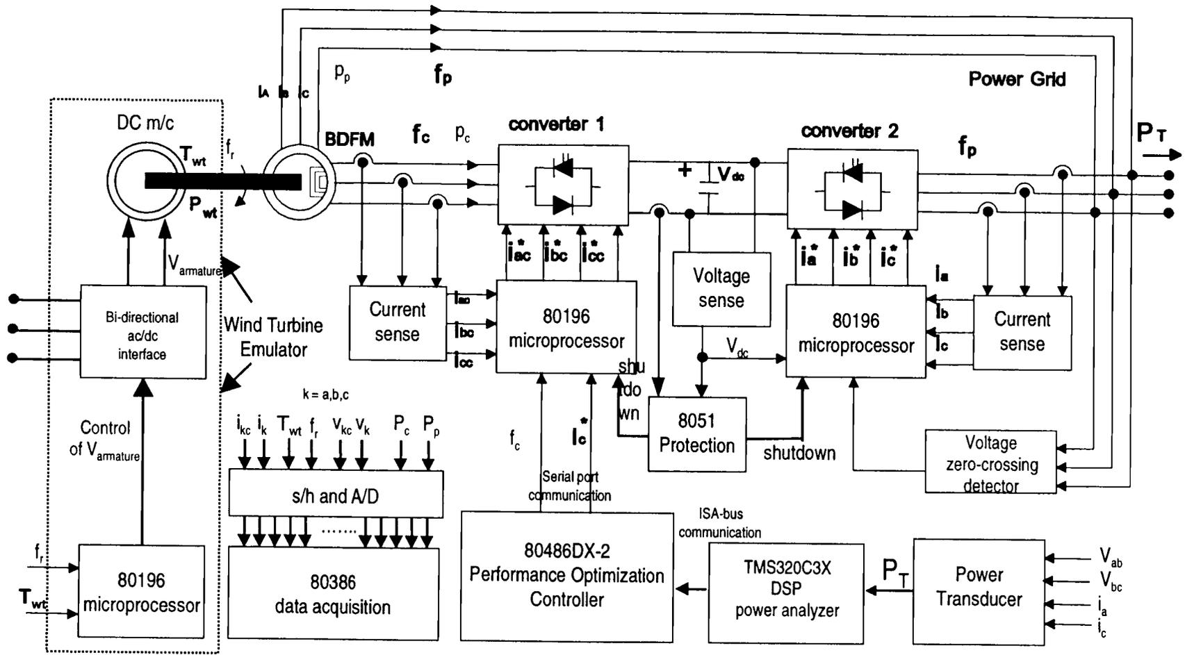
Figure 4.1 Laboratory VSG wind power generation system implementation
