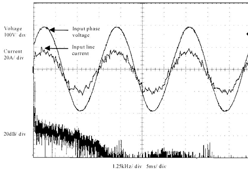
**Figure 3.19** Rectifier operation with an imposed (+)17% grid voltage error.
