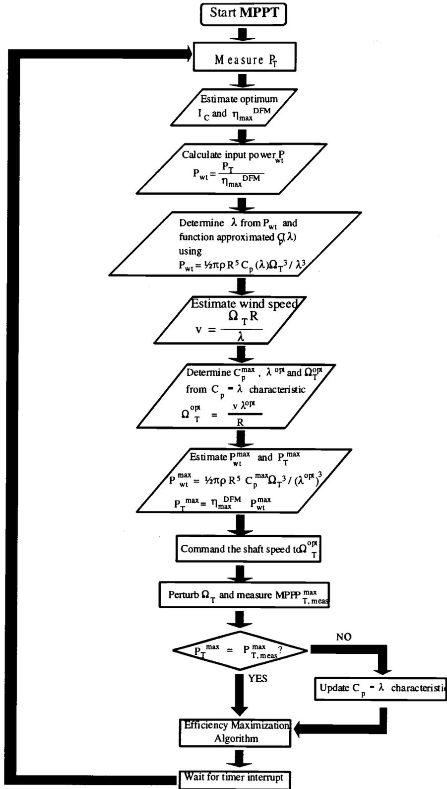
Figure 2.7 Maximum power point tracking based on estimated wind speed.
