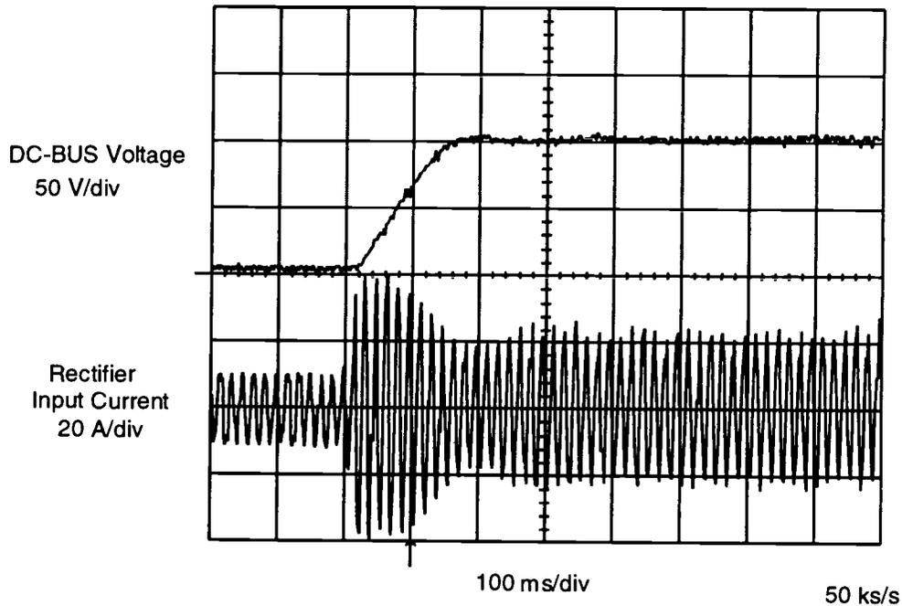
**Figure 3.6** Rectifier controller response to a 40% (280 V- 390V) step change in commanded dc-bus voltage. DC-bus capacitance = 2400  $\mu$ F
