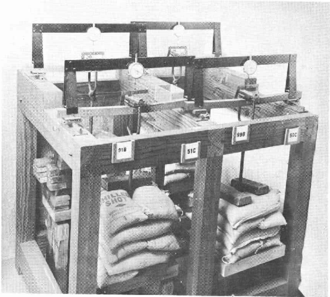
Figure 4.--A typical test frame containing four creep specimens under constant load. The load was applied through an iron stirrup that terminated in a wood platform holding the load of bars or bags of shot. The beams were simply supported on steel knife-edges and rollers. Deflections were shown directly on dial indicators. Not shown is the free-standing protective frame surrounding the stand.
