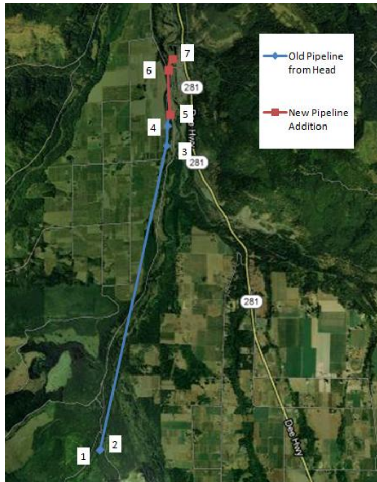
Figure 5. Map of the new pipeline route where point 1 corresponds to the Tony Creek screen house (and penstock head), point 2 the Tony creek bridge, point 3 the fairgrounds campsite, point 4 the beehive storage lot, point 5 the splice into the old pipeline, point 6 the west side of the new bridge, and point 7 the turbine house. Map was created by overlaying GPS measured coordinates onto a satellite image.
