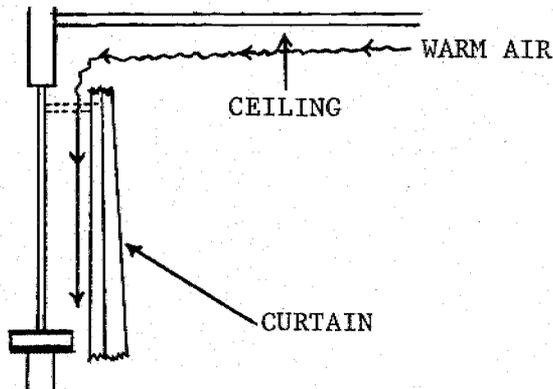
In the Illinois research,<sup>2</sup> a window shade installed within the window frame (with  $\frac{1}{8}$ " clearance on either side) resulted in a 28 percent reduction in heat loss through the window. This can be attributed to the placement of the shade inside the window frame close to the glass, which minimized the air flow between the shade and the glass. When a shade was hung outside of the window frame, heat loss was reduced by only 12 percent.
