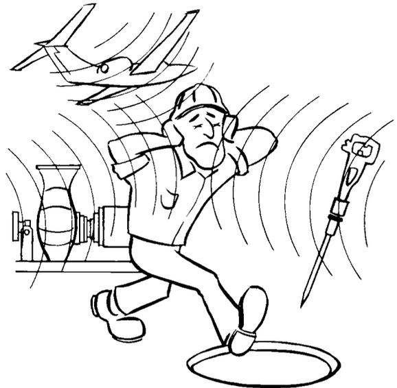
Much of the noise produced by industrial and construction sources can be reduced by installing modification to muffle the noise or by altering the basic design of equipment. For instance, quiet pile drivers have been developed which work on the principle of a humming vibration rather than pounding steam hammers. Pneumatic tools can be silenced by mufflers on intake and exhaust by as much as 20 dB(A). Much of the machinery used can be enclosed or encased in acoustical paneling.
