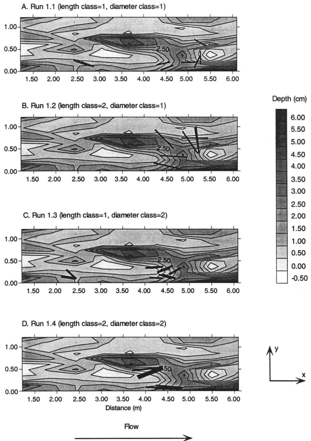
Figure 3.12. Maps of water depth and depositional location of pieces for runs 1.1-1.4.
