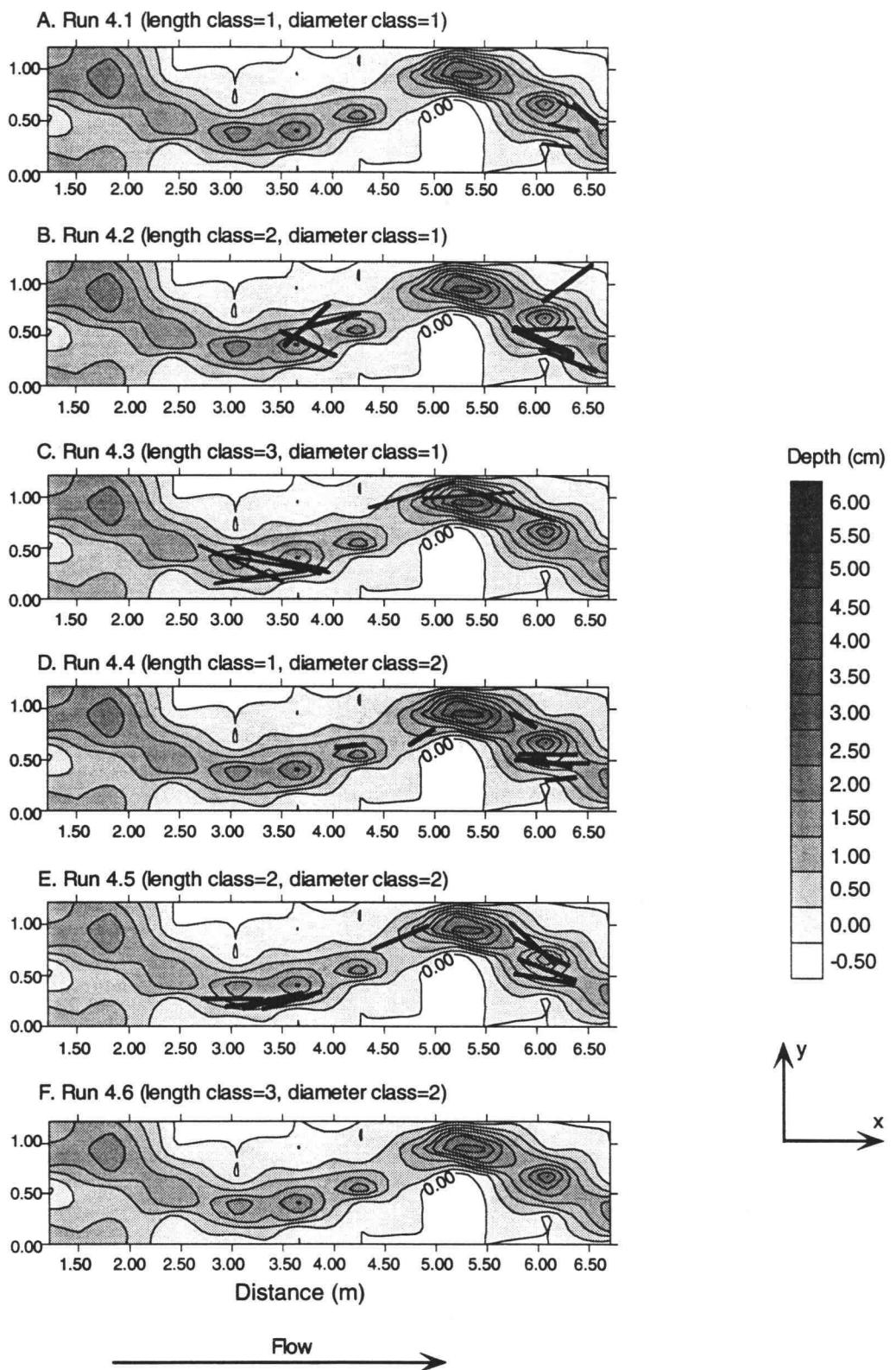
Figure 3.15. Maps of water depth and depositional location of pieces for runs 4.1-4.6.
