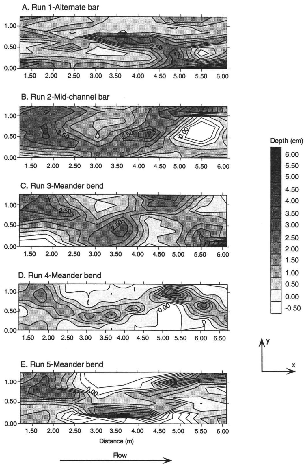
Figure 3.11. Contour maps of water depth for each of the 5 runs.
