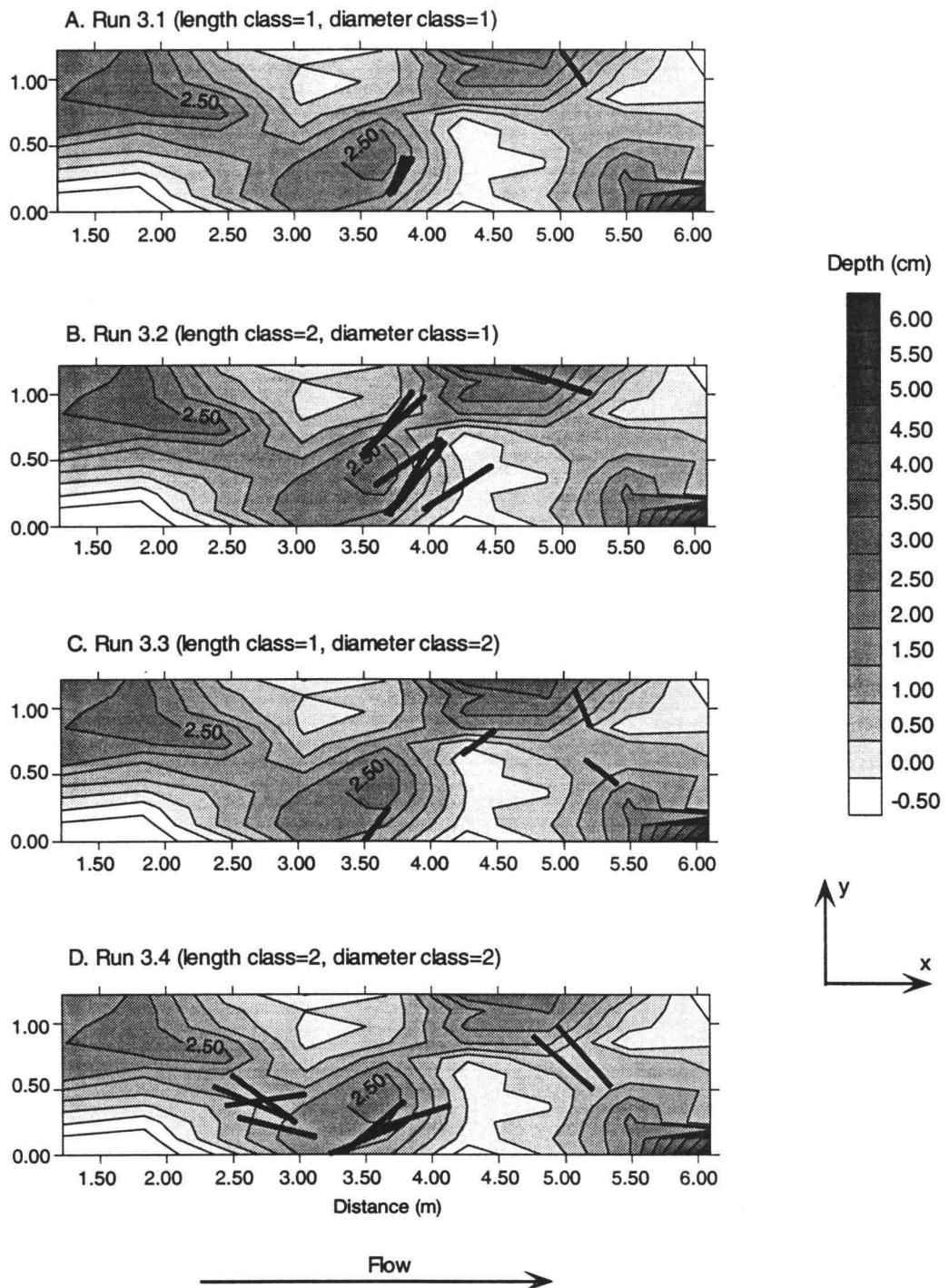
Figure 3.14. Maps of water depth and depositional location of pieces for runs 3.1-3.4.
