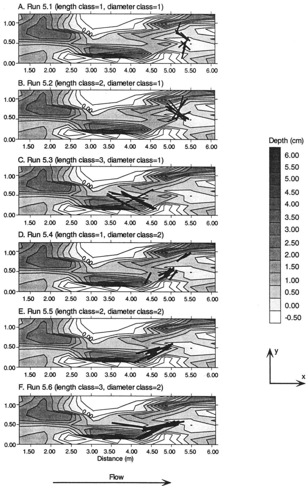
Figure 3.16. Maps of water depth and depositional location of pieces for runs 5.1-5.6.
