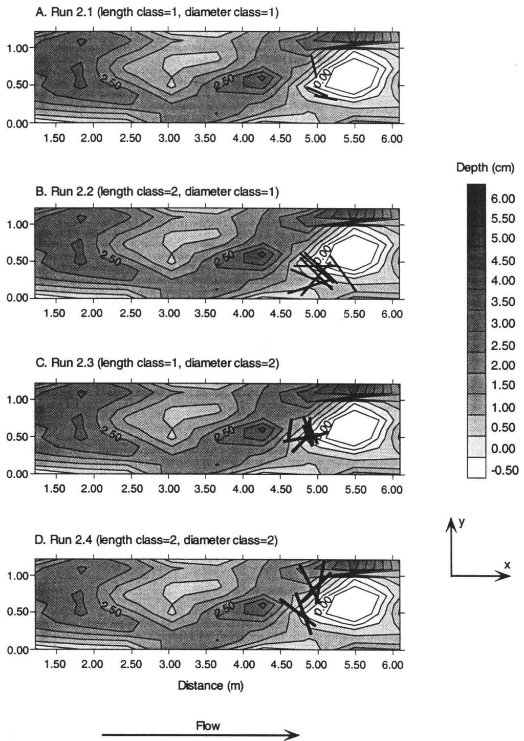
Figure 3.13. Maps of water depth and depositional location of pieces for runs 2.1-2.4.
