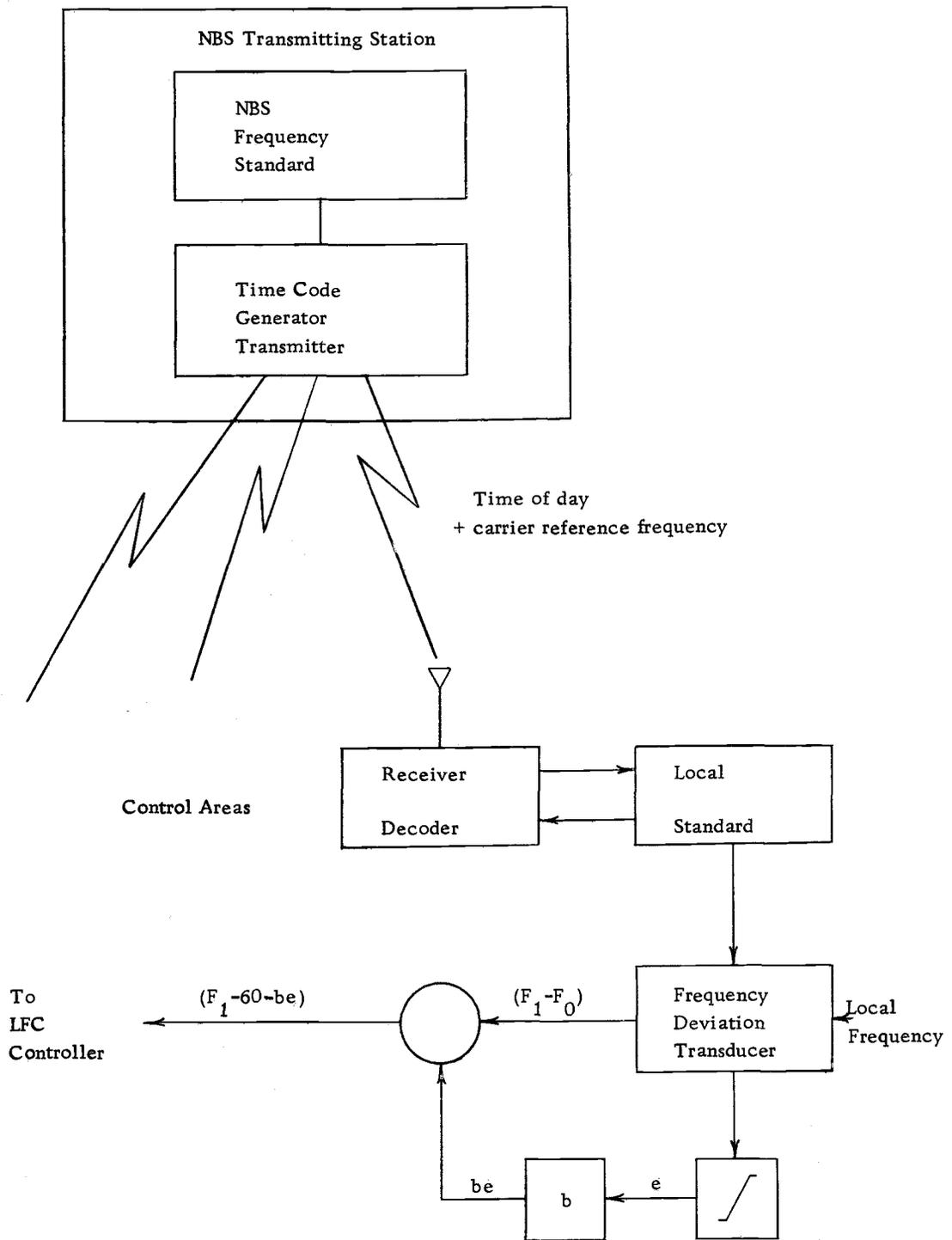
Figure 9. Automatic time correction system. Method II: Remote deviation calculation.
