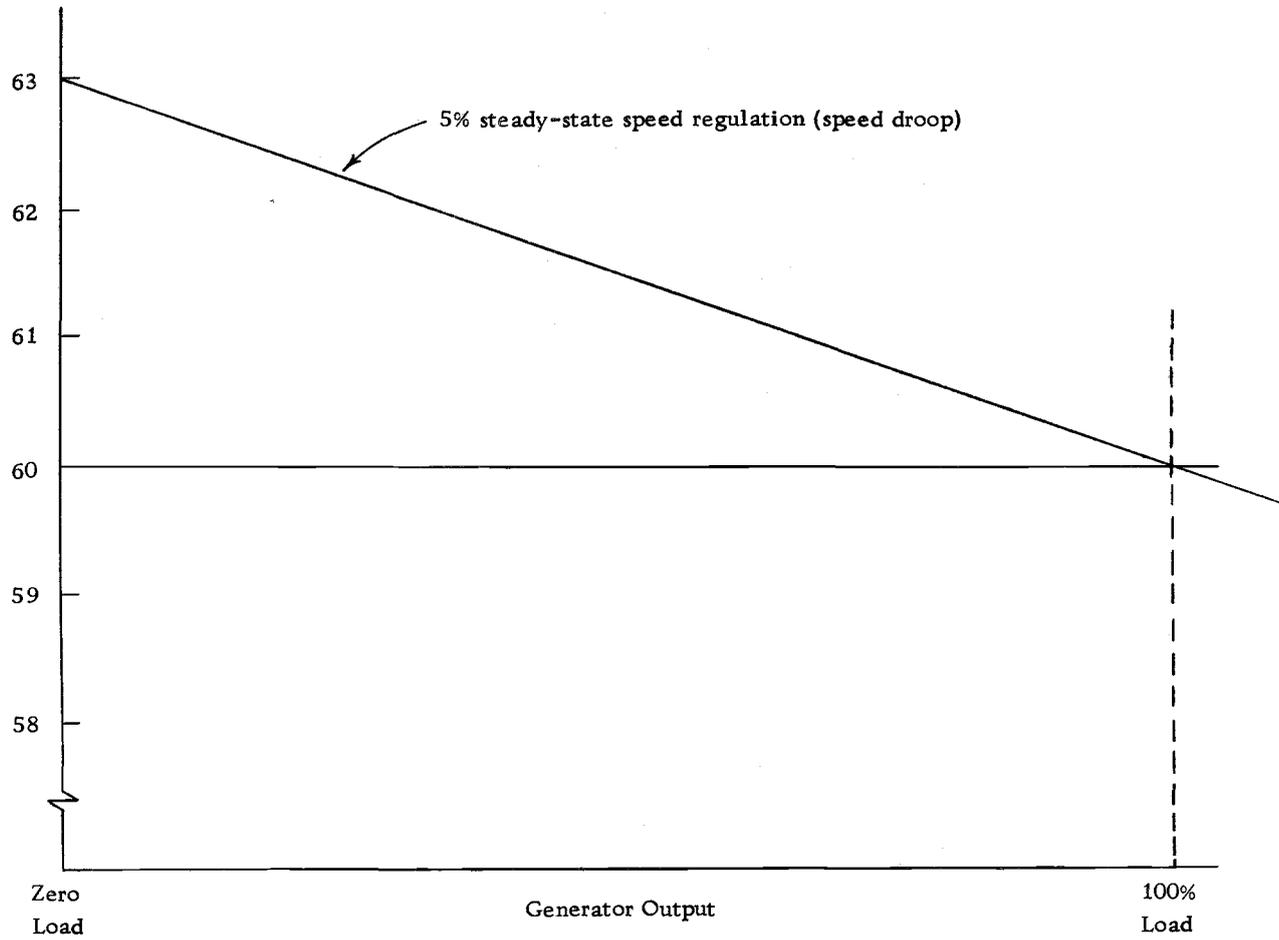
Figure 1. Steady-state speed regulation.
