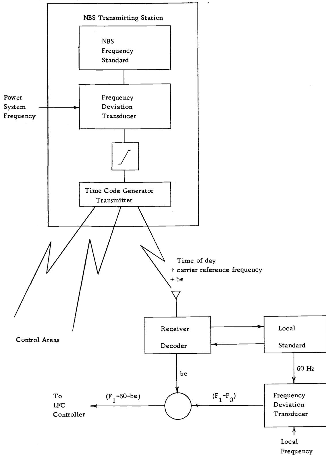
Figure 8. Automatic time correction system. Method I: Central deviation calculation.
