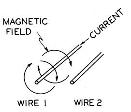
Figure 8. Interference in wire #2 due to expanding/collapsing magnetic field of wire #1.
