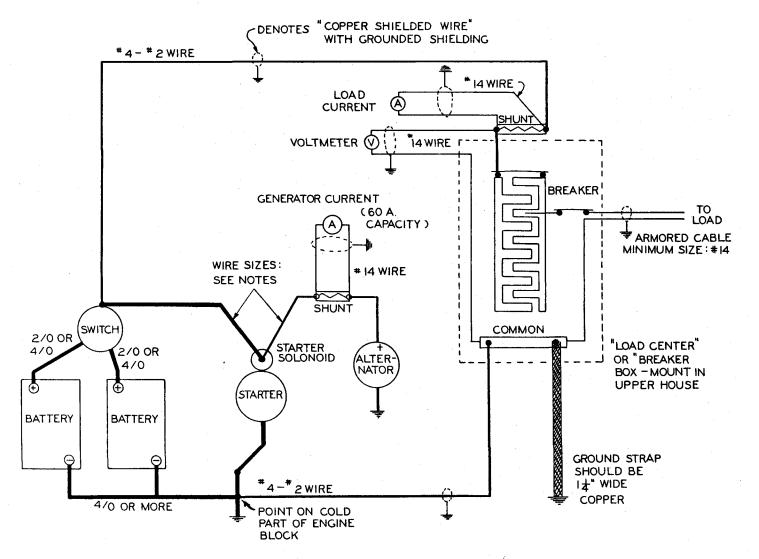
Figure 3. Boat wiring diagram (sizes for typical 12V system).
