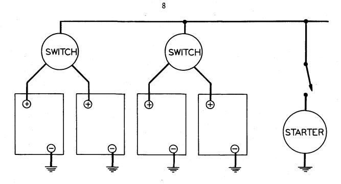
Figure 5. Safety switch for each two batteries.
