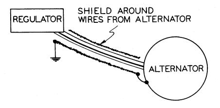
Figure 9. Typical shielded wire application.
