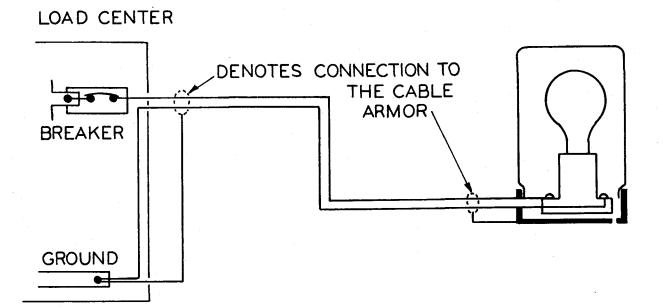
Figure 2. Wiring lights with shielded cable.
