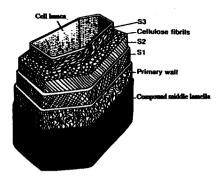
FIGURE 1. Layering structure of a wood cell. Source: Dry Kiln Operator's Manual
