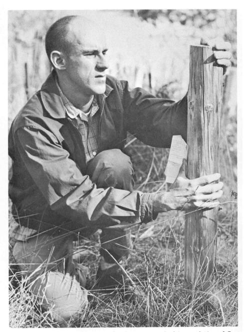
Figure 8. All posts of Douglas fir that were soaked in a solution of Osmosalts were in excellent condition after 12 years in service.
