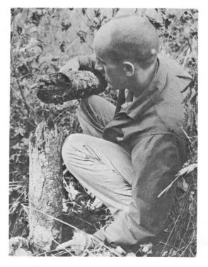
Figure 5. Tops of Douglas fir posts were not protected adequately when chemicals were placed in holes drilled near the ground line of undried, unpeeled posts. Brushing is <u>not recommended</u> for posts regardless of the preservative applied, for penetration of preservative is low, and amount of preservative retained by posts is small, even under optimum conditions.
