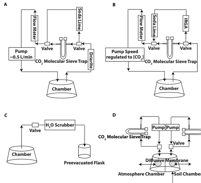
Figure 1 The four chambers that were modeled: (A) A dynamic chamber with a pump speed set to 0.5 L/min (Gaudinski et al. 2000); (B) A dynamic chamber with a pump speed that matches the flux rate (Schoor and Trumbore 2006); (C) A static chamber where  $CO_2$  accumulates for 30 min prior to sampling (Hahn et al. 2006); (D) A diffusion-driven dynamic chamber, which is based on the isotopic-forced diffusion (Iso-FD) design for a  $\delta^{13}C$  chamber presented in Nickerson et al. (2013).
