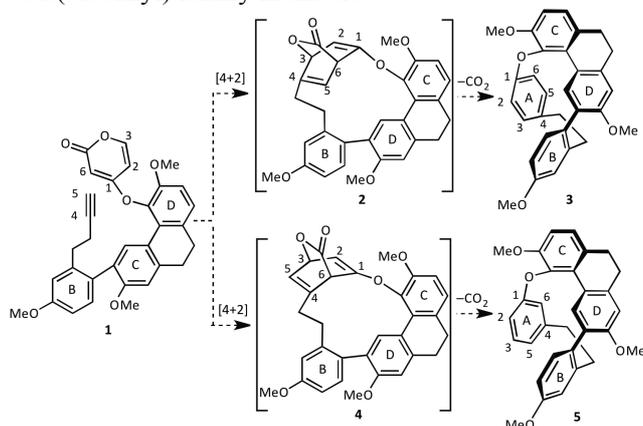
**Scheme 2.** Pyrone-Alkyne Diels–Alder Reaction for Cavicularin.
