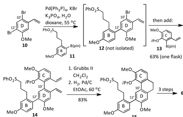
**Scheme 5.** Suzuki Reactions for Cavicularin.
