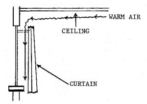
In the Ilinois research,<sup>2</sup> a window shade installed within the window frame (with  $\frac{1}{2}$ " clearance on either side) resulted in a 28 percent reduction in heat loss through the window. This can be attributed to the placement of the shade inside the window frame close to the glass, which minimized the air flow between the shade and the glass. When a shade was hung outside of the window frame, heat loss was reduced by only 12 percent.
