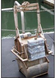
Figure 2: Box corer used for collecting infaunal invertebrates.
