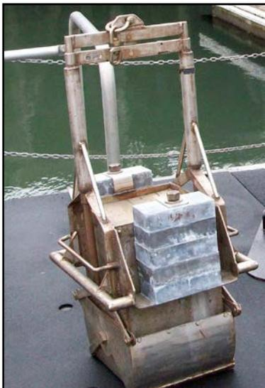
**Figure 2: Box corer used for collecting infaunal invertebrates.**
