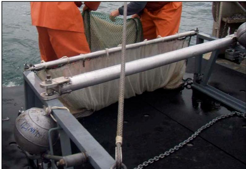
**Figure 3: Beam trawl used for collecting epifaunal invertebrates and groundfish.**
