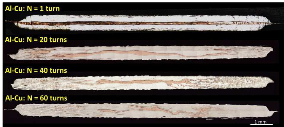
Figure 4.1 Optical micrographs of vertical cross-sections of the HPT-processed Al-Cu disks from top to bottom: 1, 20, 40, and 60 rotations.
